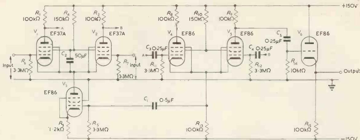
Fig. 5: Practical differential amplifier stage
