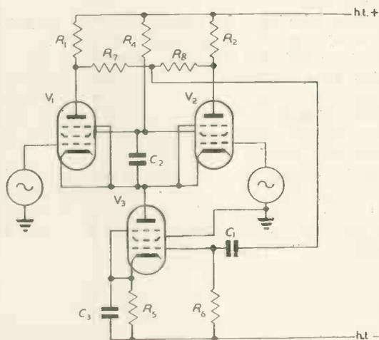
Fig. 4. Differential amplifier stage with additional feedback
