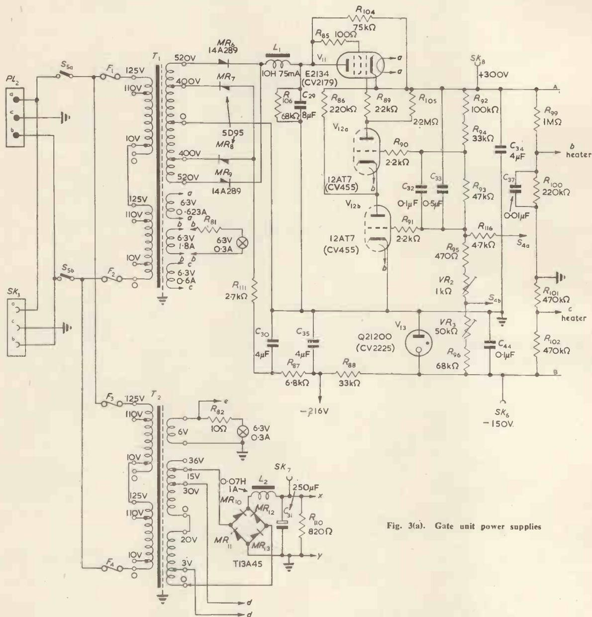
Fig. 3(a). Gate unit power supplies
