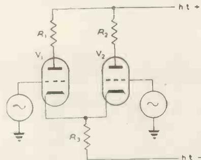
Fig. 1. Simple differential amplifier stage
