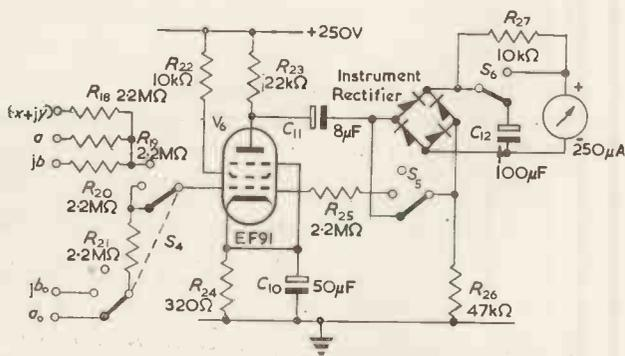
Fig. 4. Detector and voltmeter
