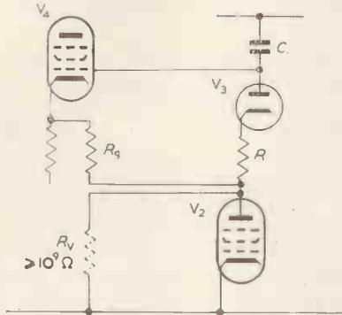
Fig. 3. Guarding circuit to minimize effect of leakage path across trigger valve  $V_2$ .
