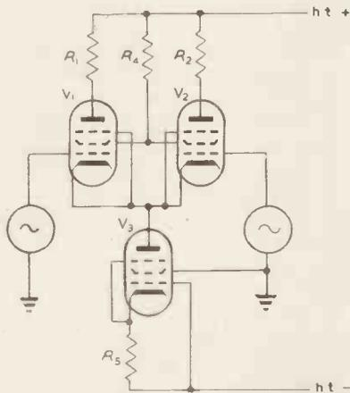
Fig. 2. Conventional differential amplifier stage using pentodes
