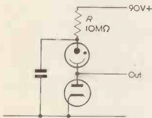
Fig. 1. Basic circuit
