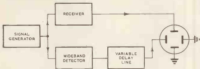
Fig. 21. Measurement of receiver phase delay
