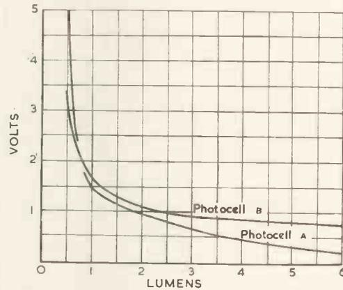
Fig. 9. Light/voltage characteristic of two different photocells, at constant current of 10 $\mu$ A
