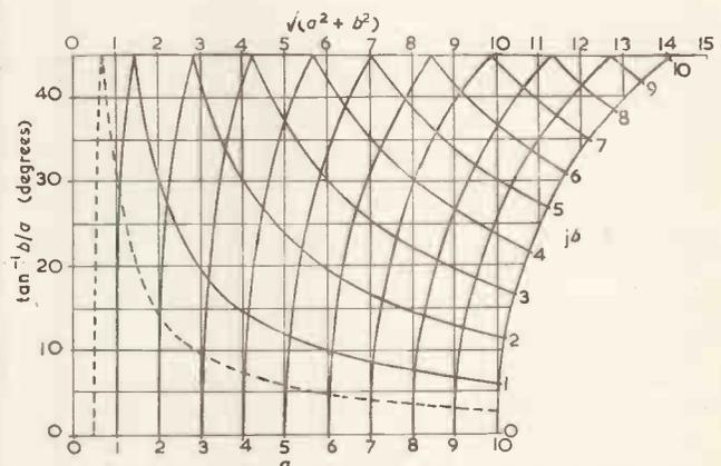
Fig. 5. Chart for obtaining the modulus and phase-angle
