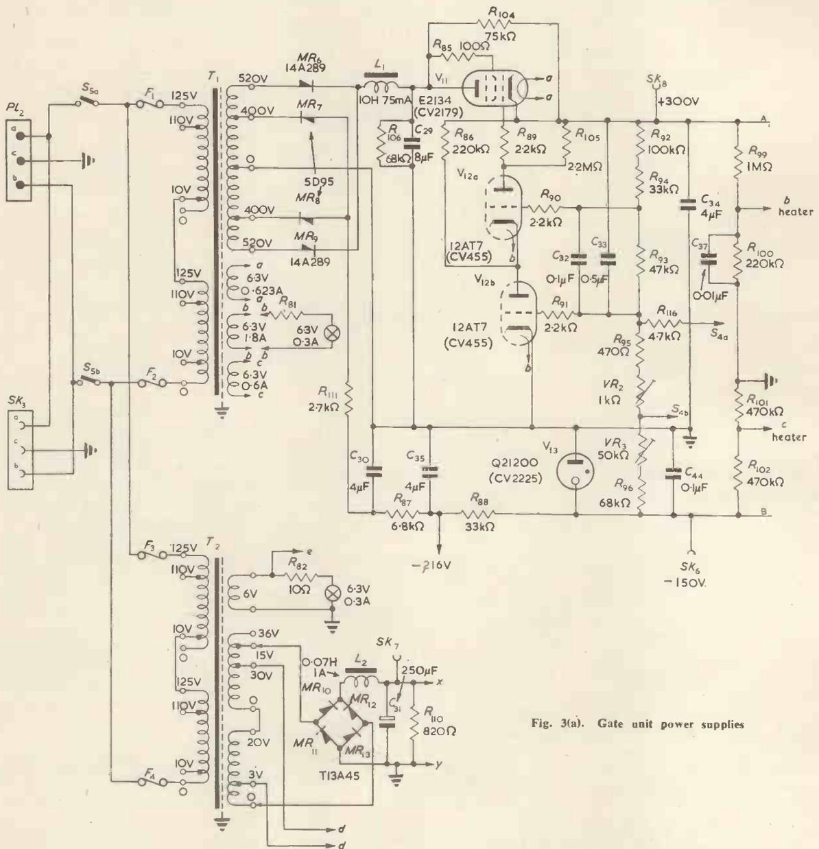
Fig. 3(a). Gate unit power supplies
