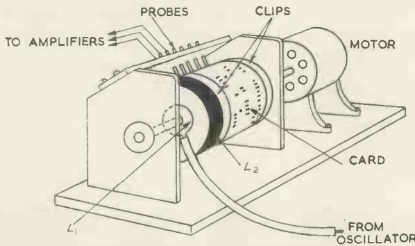
Fig. 1. Motor-driven drum mechanism
