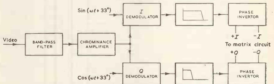
Fig. 14. Block diagram of  $I$ - $Q$  demodulation system
