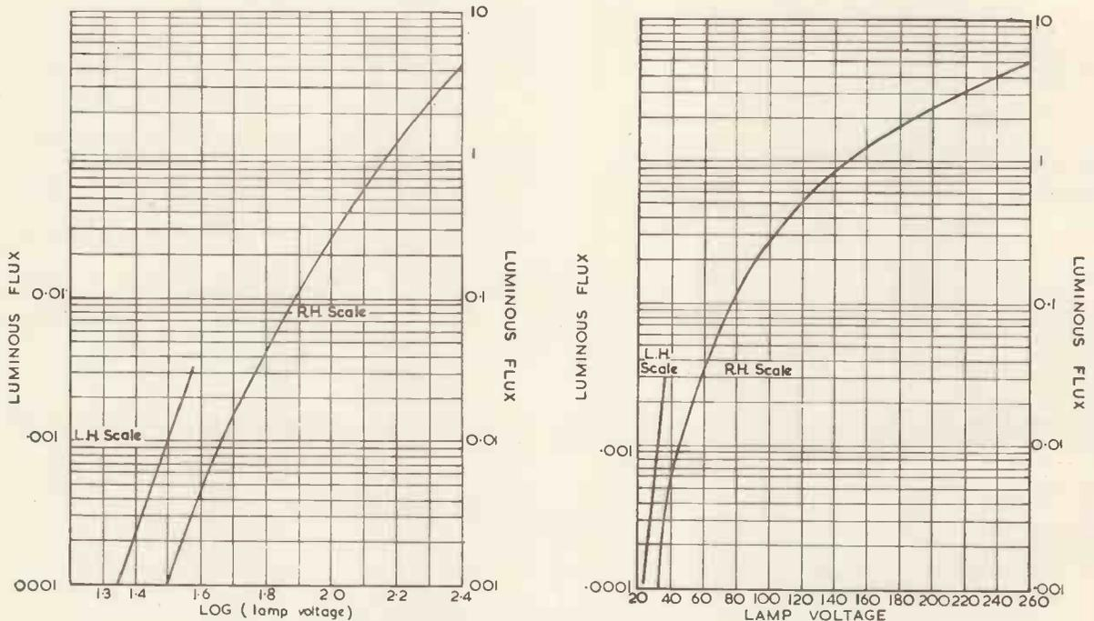
Fig. 11. Light output/lamp voltage for a 200W single coil tungsten filament lamp
