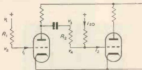
Fig. 4. Basic distortion reducing circuit
