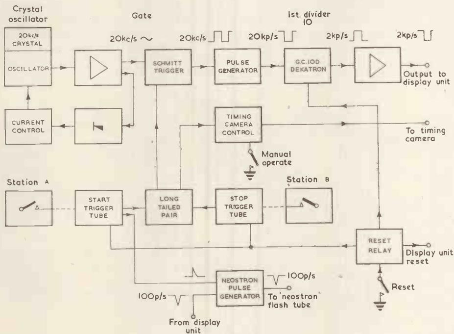
Fig. 2. Arrangement of gate unit
