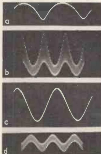
Fig. 3. Waveforms, showing distortions before and after correction
