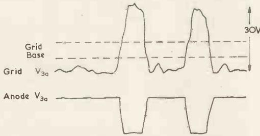
Fig. 3. Waveforms produced at grid and anode of  $V_{3a}$
