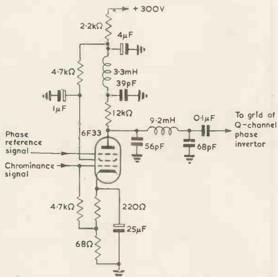
Fig. 16. A synchronous demodulator circuit
