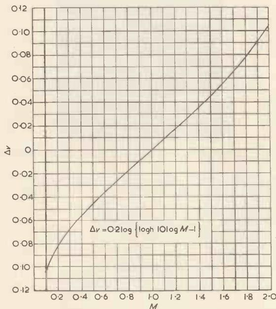
Fig. 5. Transfer characteristic of circuit with distortion correction
