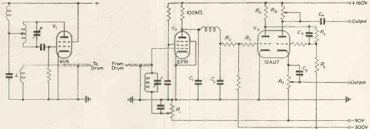
Fig. 2. Oscillator, probe amplifier, pulse clipping and shaping stages
