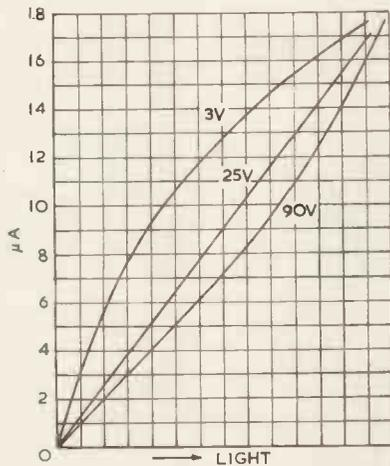
Fig. 8. Light/current characteristic of a particular photocell, showing non-linearities at high and low voltages. The light scale is linear in each case
