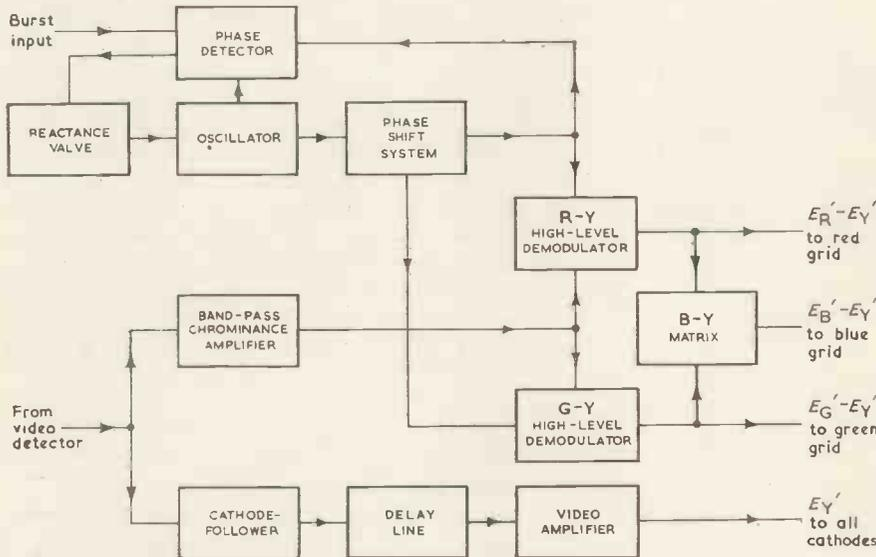
Fig. 15. The chrominance and luminance sections of a simple colour receiver
