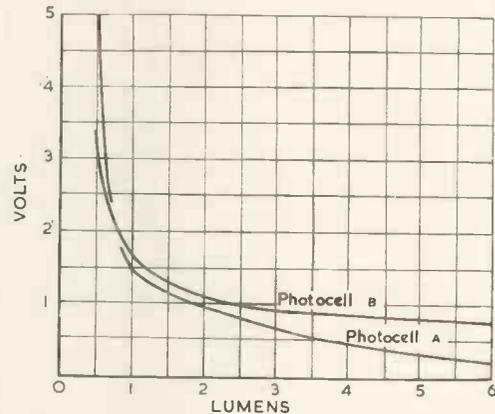
Fig. 9. Light/voltage characteristic of two different photocells, at constant current of 10 $\mu$ A
