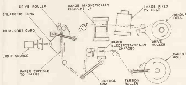
Fig. 1. Automatic enlarger printer
