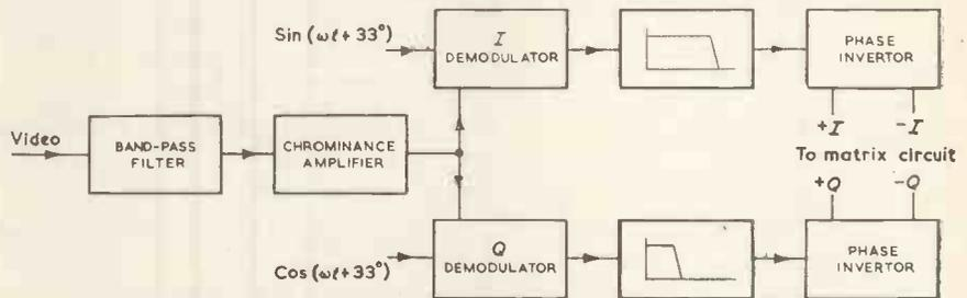
Fig. 14. Block diagram of  $I$ - $Q$  demodulation system
