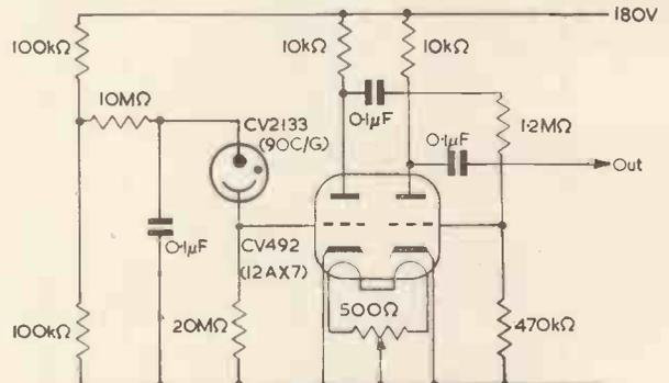
Fig. 6. Complete circuit, including distortion correcting circuit, using CV492 valve
