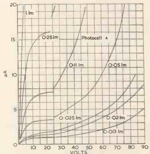
Fig. 7. Family of voltage/current characteristic curves for a particular CV2133 photocell, showing marked discontinuities at about 25V
