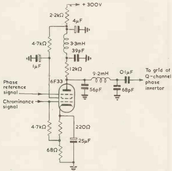
Fig. 16. A synchronous demodulator circuit
