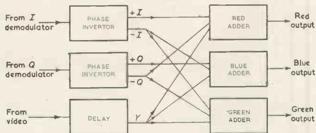
Fig. 17. Block diagram of I-Q matrix unit
