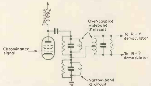
Fig. 20. Matrixing at sub-carrier frequency (after Hazeltine Corp.)
