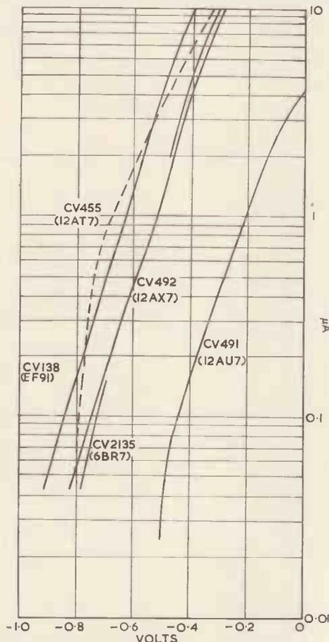
Fig. 2. Grid voltage/grid current characteristics of some triodes and pentodes
