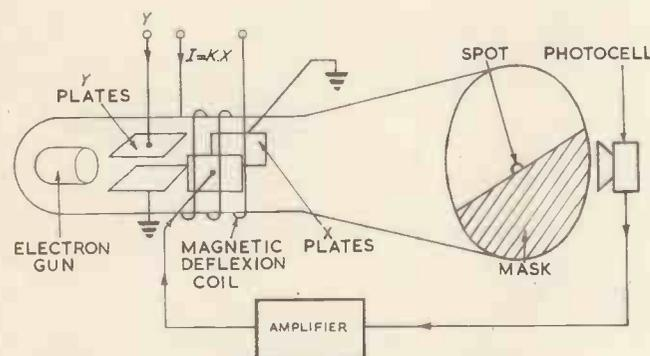
Fig. 7. Basis of an electron beam multiplier
