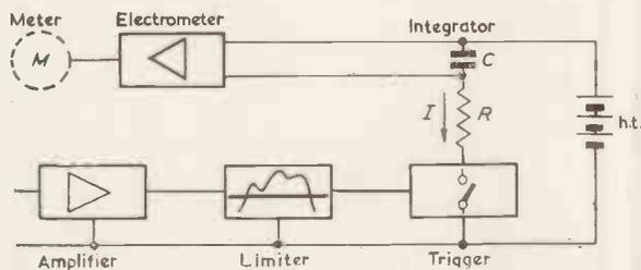
Fig. 1. Capacitance-integrator system
