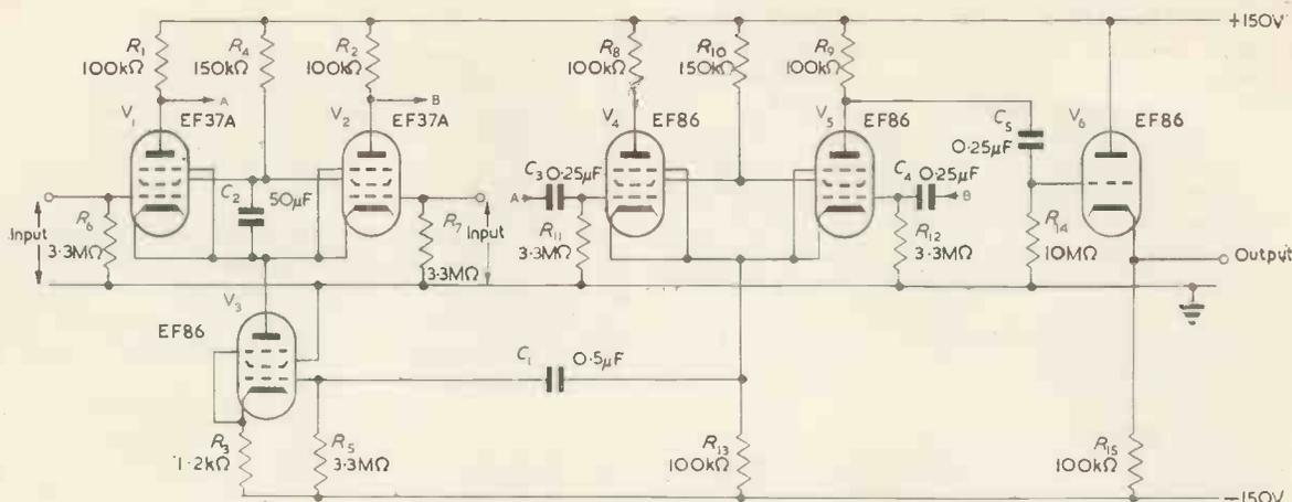
Fig. 5: Practical differential amplifier stage
