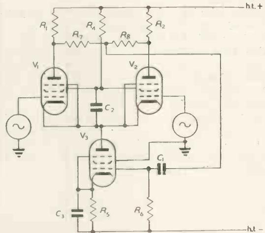
Fig. 4. Differential amplifier stage with additional feedback
