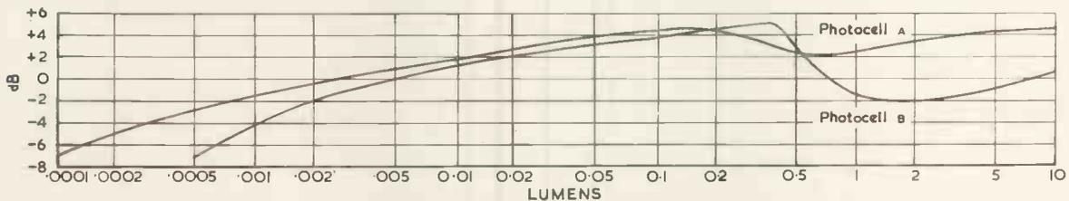
Fig. 10. Overall performance curves, using a 50c/s lamp source with 7 per cent modulation, showing the change in output due to the substitution of the two photocells A and B (see Figs. 9 and 7 for characteristics of these two photocells)
