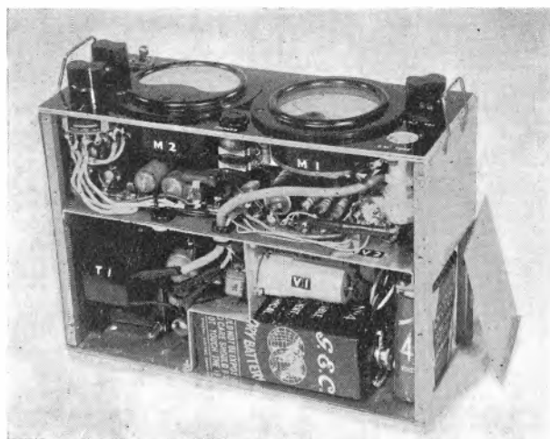
Fig. 2. Portable Geiger counter equipment (side panel removed)
