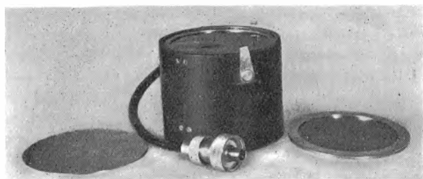
Universal ionization chamber for \alpha , \beta , \gamma and X-rays, approx. 500 c.c. (Courtesy Baldwin Instrument Co.)
