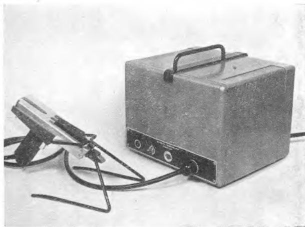
Fig. 5. Mullard ultrasonic soldering iron with 50 watt 20 kc/s. drive unit. Heating (extra) 100 watts, 50 c/s.
