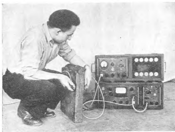
Fig. 3. The ultrasonic testing equipment "Ultracouel" being used to detect laminations in sheet steel. (Ateliers de Constructions Electrique de Charleroi)
