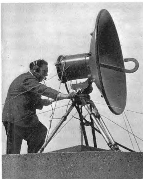
(left): Portable Microwave Television Receiving Equipment supplied by Marconi's Wireless Telegraph Co., Ltd. installed on a water tower at Warren Street near Lenham.
