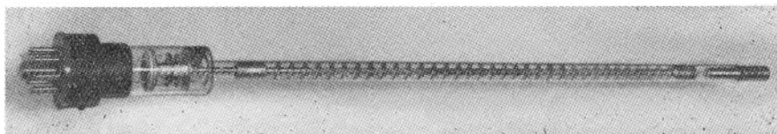
MS1 200. Medium Power Tube 3 600-4 200Mc/s
