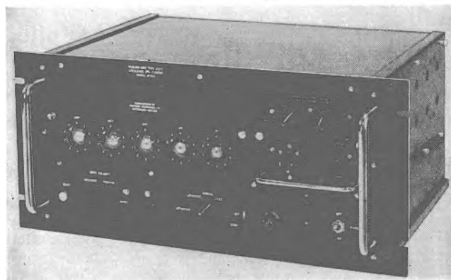
Fig. 5. The scaler complete with timing unit
