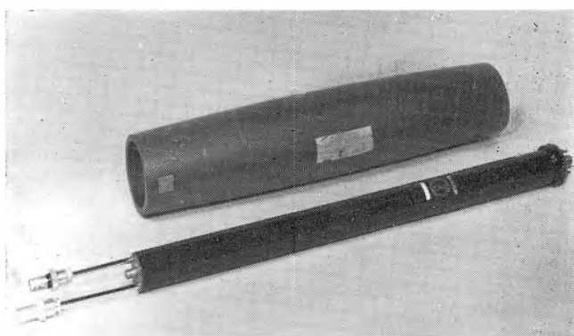
Fig. 2. A uniform permanent magnet shown with the travelling-wave tube for which it is intended
