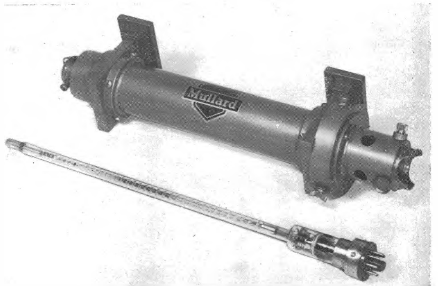
Fig. 3. Periodic permanent magnet and coupling system for the Mullard LA4-250 intermediate amplifier This t.w.t. will give over 25dB of gain and 250mW of power in the band 3.6 to 4.2kMc/s
