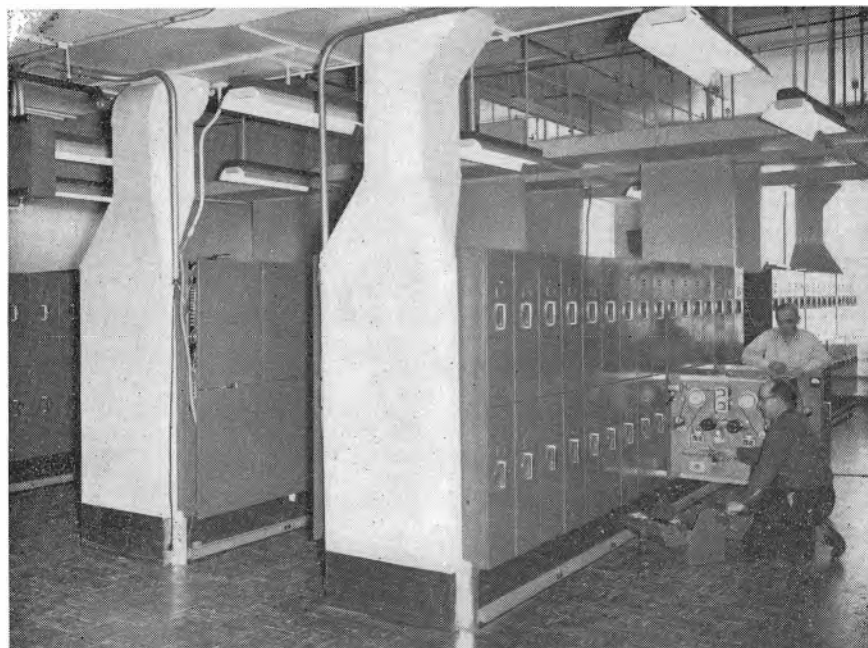
The banks of tape stations installed at OTAC
