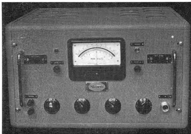
Phase indicating voltmeter (scheme A)
