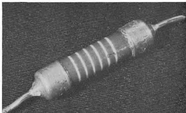
Fig. 13. RC2 resistor—arcing of longitudinal crack
