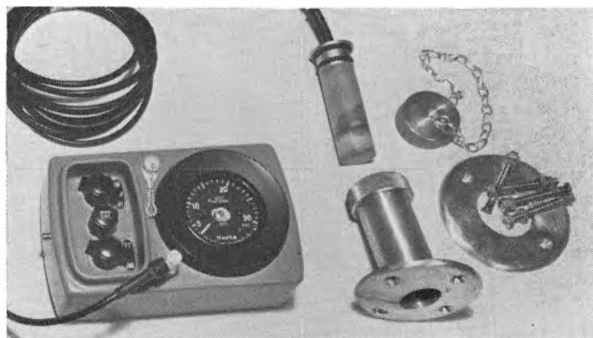
Fig. 5. The complete installation including the transducer housing which is fitted in a hole in the ship's bottom. The transducer is retractable for cleaning when the boat is afloat
