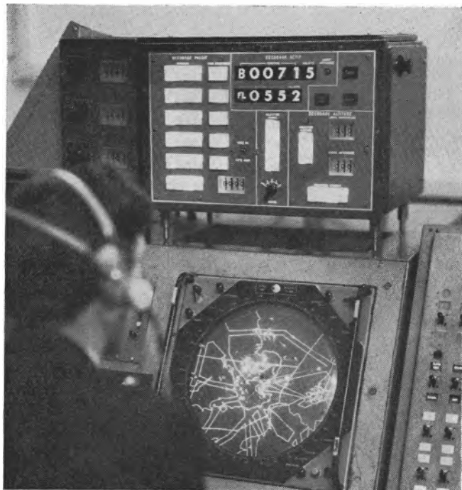
The SECAR control and indicator unit mounted above the normal p.p.i. display
