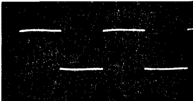
Fig. 7 (below). Amplifier response to 50c/s square-wave input, 16Ω resistive load
