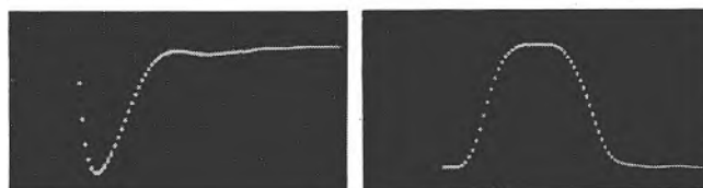
Fig. 6. Turn-on waveform of the 1000\mu sec pulse Horizontal scale: 5nsec/div . Vertical scale: 2V/div .
