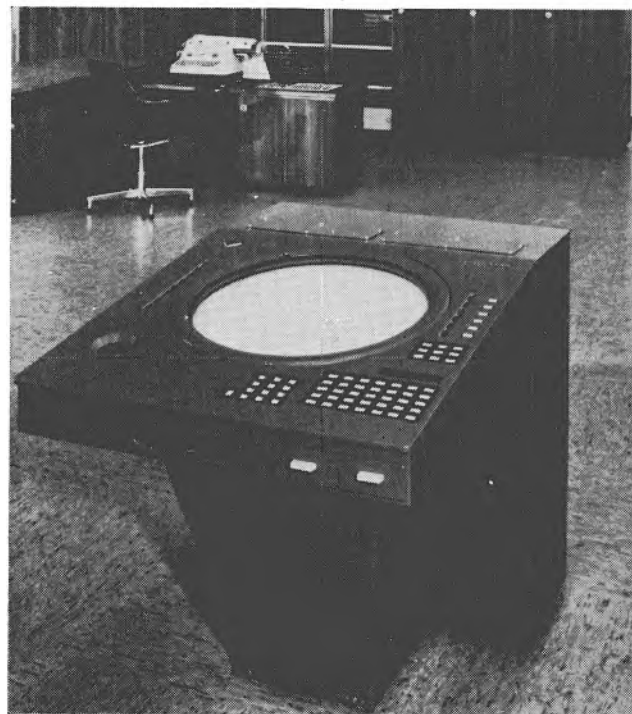
A display unit specifically designed for automatic air-traffic control use.
