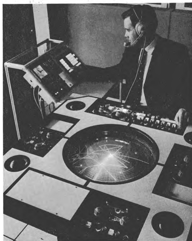
Horizontal radar display unit with video map, micro-tabular display, controls and keyboard
