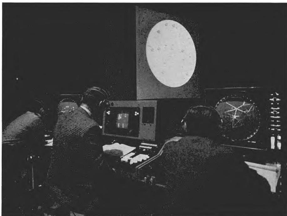
Supervision position—two radar consoles, one pilot's console, input keyboard and large screen display
