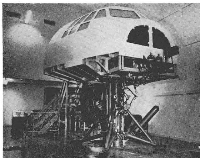
Fig. 1. The Belfast Three-axis Simulator weighing approximately 8000lb
