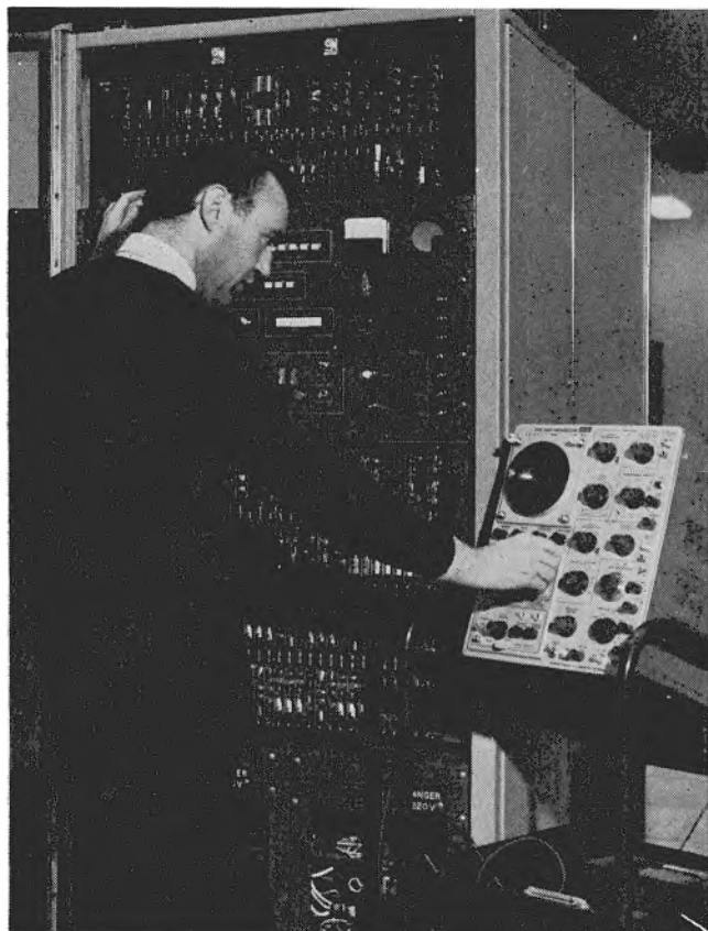
Radar simulator control panel for selection of radar characteristics
