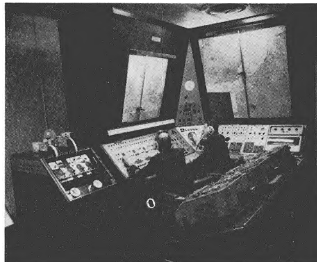
Fig. 2. The Instructors' Control Desk showing the several tape recorders and the maps of the routes of the simulated flight
