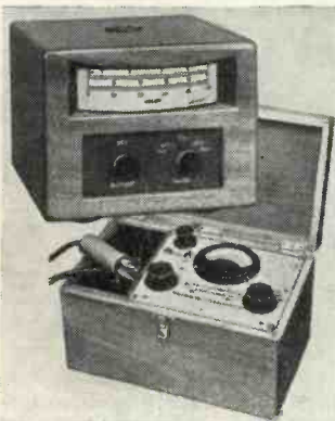
Fig. 1. Typical electronic precision measuring instruments—valve voltmeters by the Salford Electrical Co.
