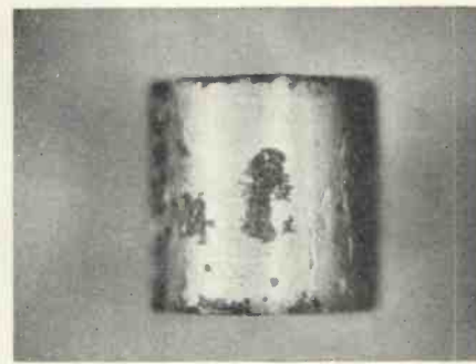
Fig. 2. Photomicrograph of semi-cylindrical contact showing the effect of flawed base metal.
