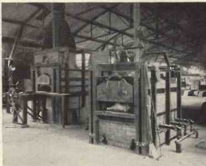
Processes in the manufacture of Mycalex : Fig. 3 (left) Compressing the mica-glass mixture in a hydraulic press before final firing, and Fig. 2 (right), The glass ingredients undergoing preliminary baking before being mixed with mica flour.
