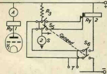
quired, one for relays with "make" contacts, and another for "break" contacts. It seemed to me that one universal instrument with a change-over switch incorporated would be more useful. Therefore, I append a modification of Mr. Bacon's circuit which appears as Fig. 4 in his article.
