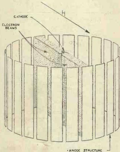
Fig. 1. Elementary tube structure showing focused beams.
