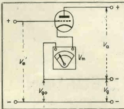
Fig. 3. Use of a boosting voltage (German Patent 690207)  $V_{gk0}$  grid-cathode voltage for  $I_a = 0$   $V_m$  voltage at an instrument connected as load of the anode circuit.
