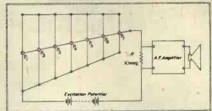
Fig. 4. The basic arrangement of electrostatic pickups in combination with stretched wires tuned to the musical scale. The arrangement exactly as shown is directly applicable with good effect to an ordinary piano.
