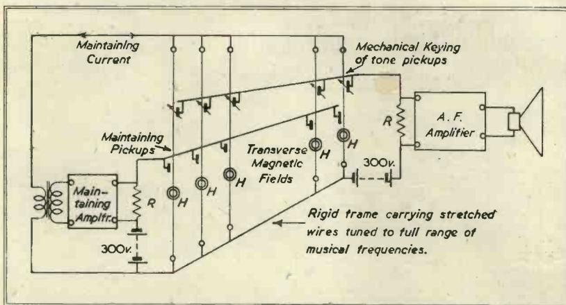
Fig. 5. The basic arrangement of an electronic organ using stretched wires continuously vibrating as tone-generators. One amplifier is used to maintain all the strings in vibration. A second amplifier provides the acoustic output.
