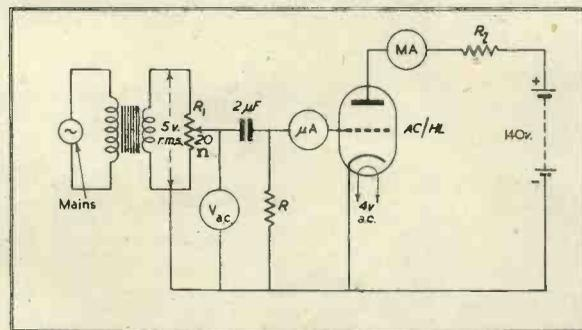
Fig. 5 (above). Determination of A.C. dynamic  $E_g$ - $I_a$  characteristics.
