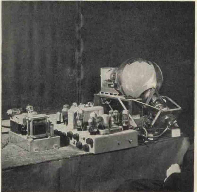
The experimental receiver and Tube assembled.
