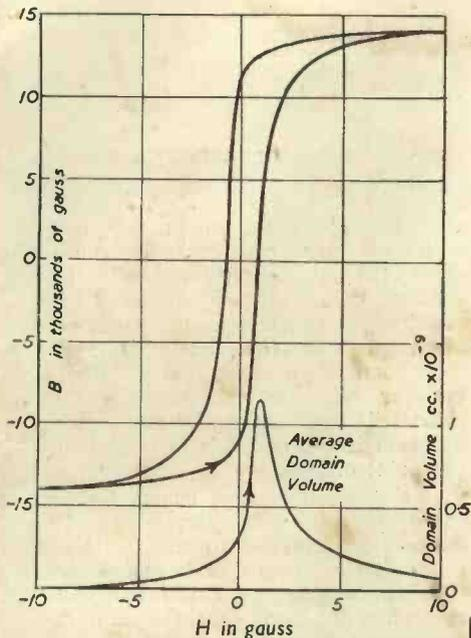
Fig. 5. Hysteresis loop and average volume of Domains for annealed iron.
