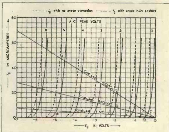
Fig. 2 (right).  $I_g-E_g$  characteristics for an AC/HL.
