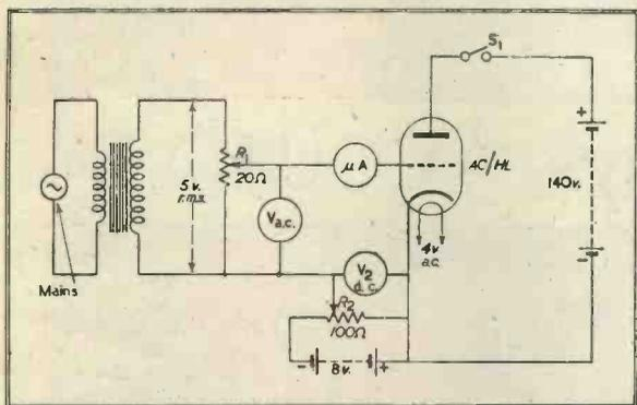
Fig. 1 (above). Apparatus for determining  $I_g-E_g$  characteristics.
