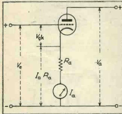
Fig. 1. Fundamental circuit.  $V_{gk}$  voltage between grid and cathode of amplifier.  $V_e$  input voltage to be measured.  $V_a$  anode voltage.  $I_a$  anode current.  $R_a$  resistance of the anode circuit.
