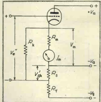
Fig. 4. Counterconnexion of  $V_{gk}$ . By the changes in cathod potential voltage changes at  $R_g$  are caused through  $R_k$  corresponding to  $V_{gk}$ .
