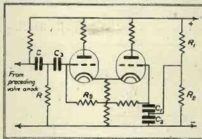
worst effects of leakage. At D.C. potentials, the resistance of the condenser  $C$  is much higher than that of the resistance  $R_2$ , and the P.D. across the latter is so low that objectionable leakage cannot occur through the coupling condenser  $C_2$  and the grid leak  $R_1$ .
