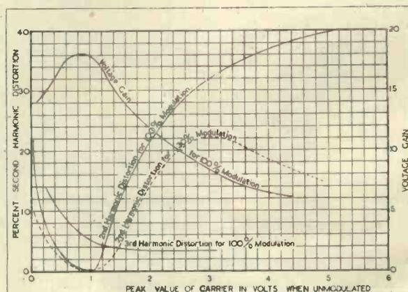
Fig. 8. Distortion of AC/HL for 100 per cent modulation (with 50,000  $\Omega$  anode load and 140 volts H.T. supply).
