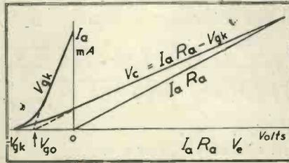
Fig. 2 Relations between  $I_a$  and  $V_{gk}$   $V_e$  and  $I_a R_a$ .
