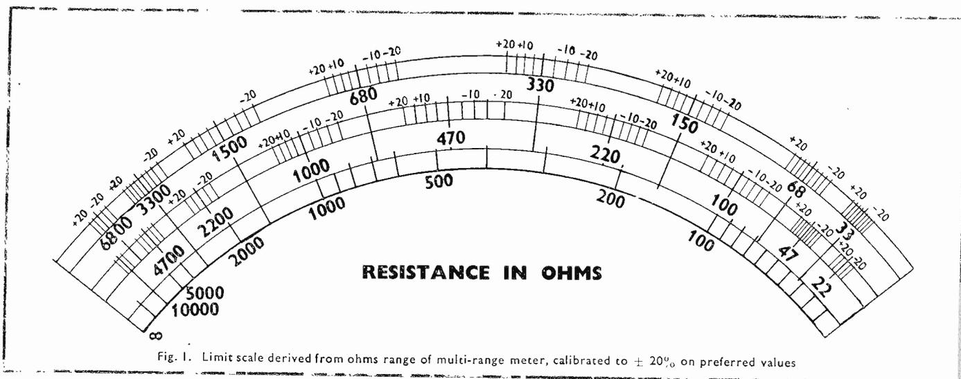
Fig. 1. Limit scale derived from ohms range of multi-range meter, calibrated to  $\pm 20\%$  on preferred values
