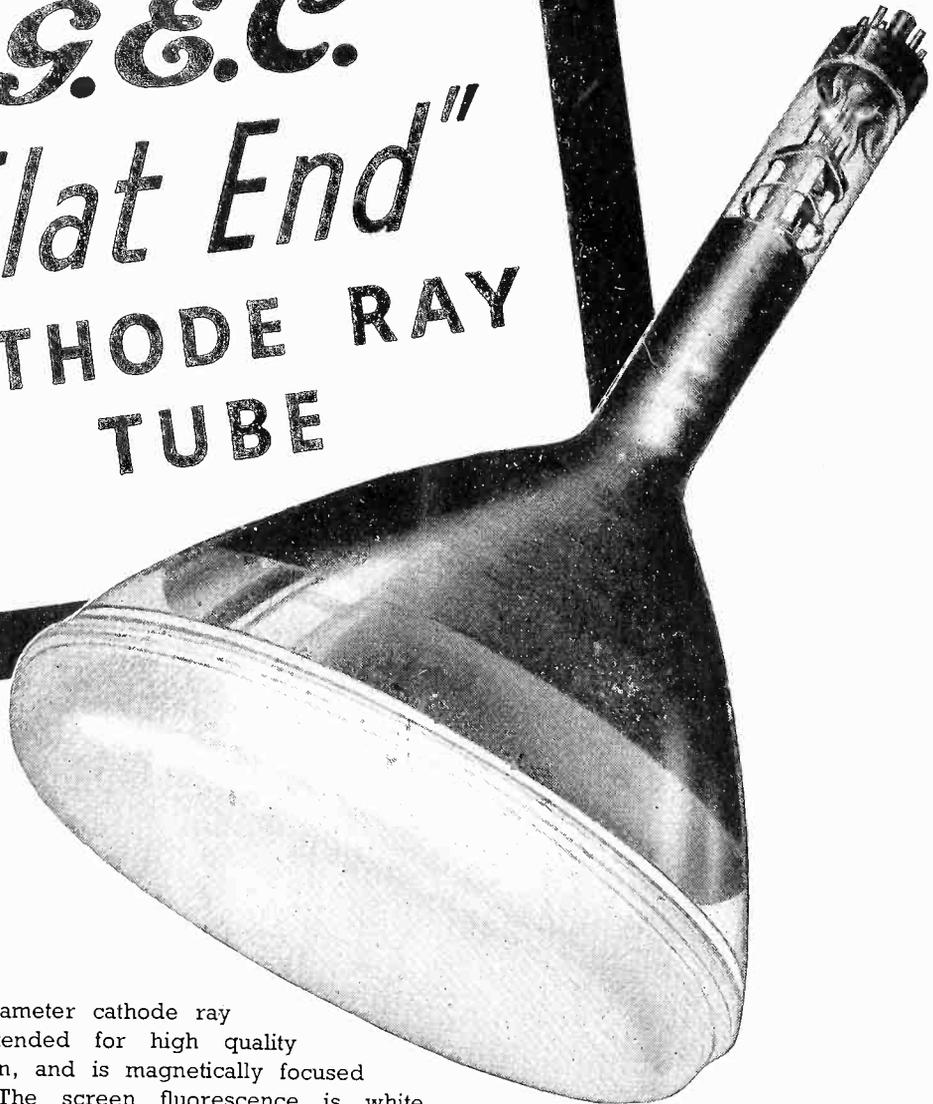
The G.E.C. 9" diameter cathode ray tube 6501 is intended for high quality television reception, and is magnetically focused and deflected. The screen fluorescence is white.
