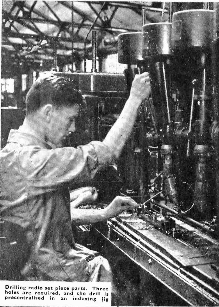
Drilling radio set piece parts. Three holes are required, and the drill is precentralised in an indexing jig
