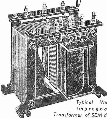
Typical Vacuum impregnated Transformer of SEM design
