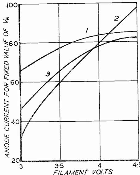
Fig. 7a. Variation of anode current with change of filament voltage for valves of varying emission quality
