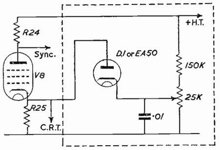
Fitting of the diode and its associated components on the sound receiver chassis can be very easily done as there is ample space and no special precautions are necessary.
