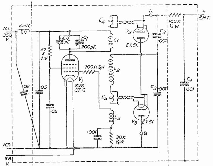
The circuit of the complete E.H.T. unit is shown on the right. Note arrangement of screening compartments, (broken lines).
