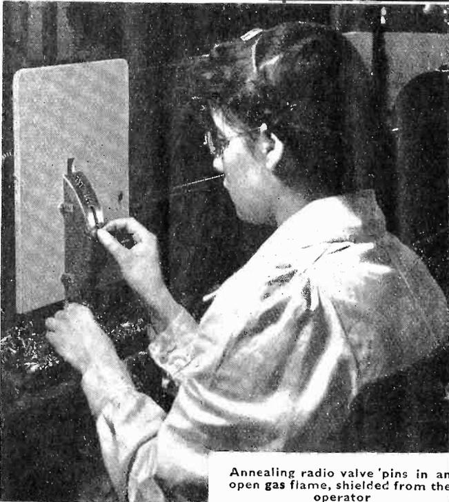
Annealing radio valve 'pins in an open gas flame, shielded from the operator
