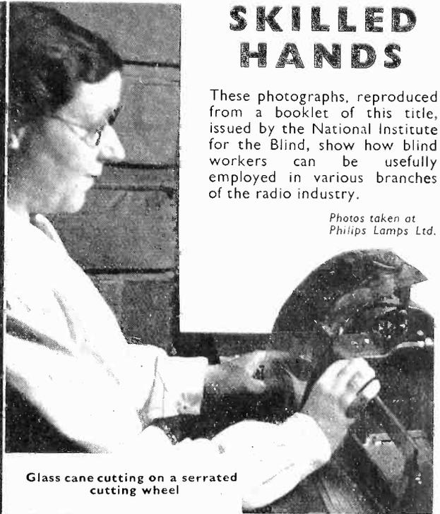
Glass cane cutting on a serrated cutting wheel
