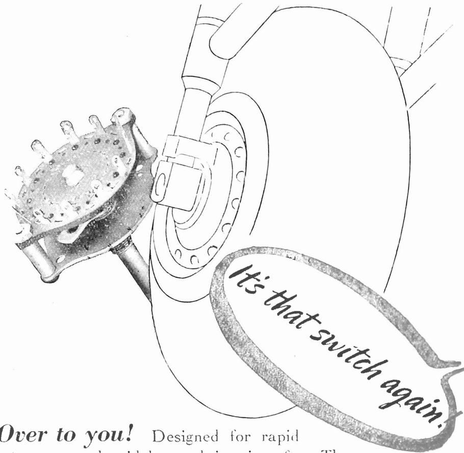
**Over to you!** Designed for rapid inter-com and widely used in aircraft. The Type 40/1542 is a simple two-way switch, spring biased so that it automatically returns to one position, normally used for speech. To listen the user rotates and holds in Position 2. This switch will find wide uses in civil aircraft and for inter-office communication on subsidiary stations.
