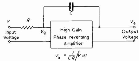
Fig. 1. Basic "Miller feedback" circuit
