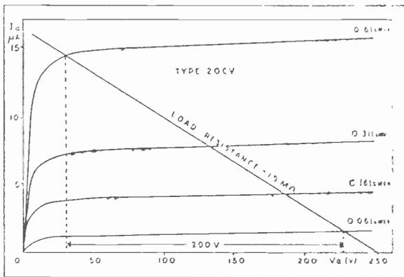
NOTE: 0.048 lumen sq. in. is the light intensity produced by a 60 watt tungsten filament lamp at a distance of 2 ft. 6 in. (Cathode area of Type 20CV = 1.25 sq. in.)
