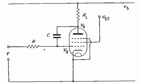
Fig. 2. "Miller Valve" circuit, using single pentode
