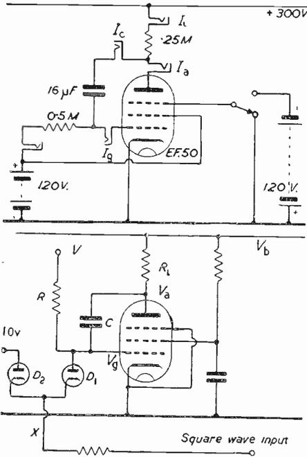
Fig. 4. Demonstration circuit for a suppressor-switched Miller valve
