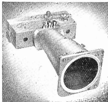
Specially developed for use with Cossor Oscillographs, it provides the simplest means of recording stationary or non-recurrent waveform<sup>s</sup> and slow transients by the moving film method on standard perforated 35 mm. film or paper. Of robust construction it has provision for power drive by the Cossor Three-Speed Motor Attachment, Model 1429.
