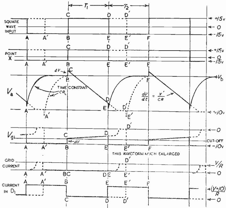
Fig. 5. Control by grid-switching. The waveforms at various points are shown on the right
