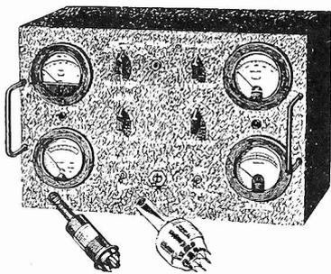
➔ **THE B.A.R. THERMOCOUPLE-IONISATION GAUGE CONTROL.**
