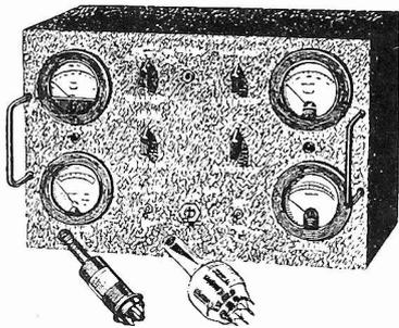
➔ **THE B.A.R. THERMOCOUPLE-IONISATION GAUGE CONTROL.**
