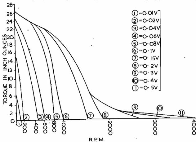
Fig. 9. Speed/torque curves (Mk II) Full feedback
