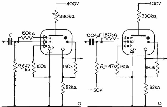
Fig. 11(a). Input circuit for pulses of type 1
