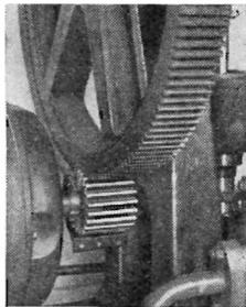
*A Tufnol Pinion meshing with a cast-iron wheel. The 18 h.p. motor provides the pump drive for a Hydraulic Accumulator.*
