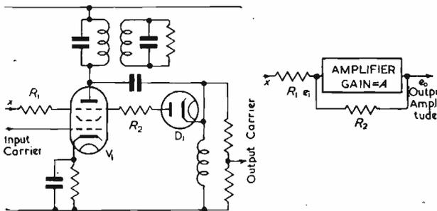
Fig. 2. Circuit for amplitude modulation      Fig. 3. Equivalent circuit
