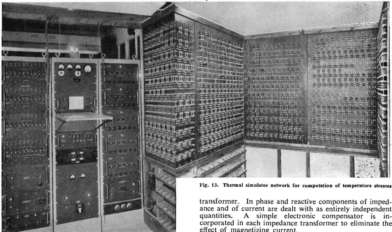
Fig. 13. Thermal simulator network for computation of temperature stresses
