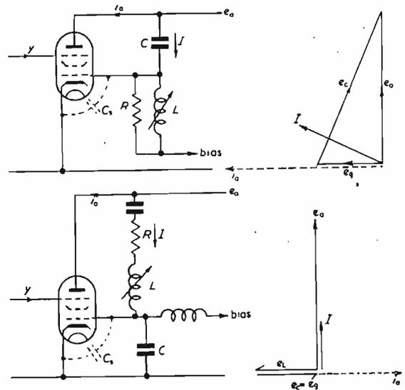
Fig. 4. Alternative arrangements to ensure that grid voltage is in quadrature with anode voltage
