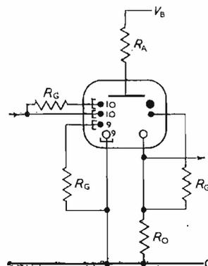
Fig. 8. Circuit referred to in tentative specification
