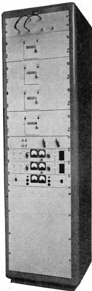
The Redifon R93 fixed frequency, high stability receiver is particularly suitable for monitoring, diversity reception or frequency shift operation. A typical application is this twin-channel, dual diversity, frequency shift radio teleprinter terminal. Multi-channel diversity or non-diversity racks can also be provided which incorporate a multi-receiver coupling unit (Redifon Type MCU.1) allowing up to eight receivers to be fed from a single aerial.
