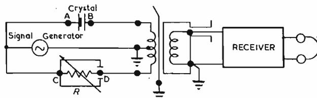
Fig. 1. Circuit for measuring resistance
