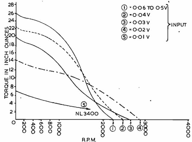
Fig. 8. Speed/torque curves (Mk II)
