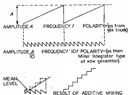
It operates as follows for ten steps: a sawtooth oscillator of amplitude  $A$ , frequency  $f$ , and positive polarity, is used to synchronize another sawtooth oscillator of amplitude  $A/10$  and negative polarity. These waveforms are  $A/10$  applied, one to each grid of a double triode having a resistance load common to both anodes. It can be seen from the above diagram that this arithmetic mixing produces a step waveform of the required shape.
