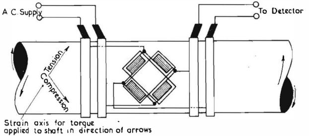
Fig. 15. Two methods of measuring torque
