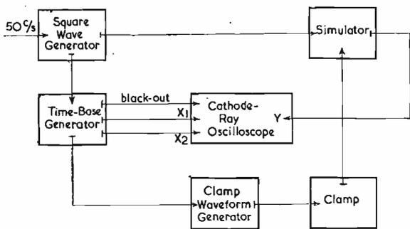
Fig. 4. Block diagram of the complete system
