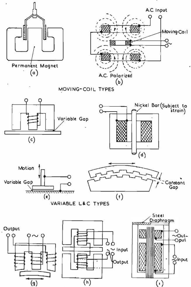
Fig. 14. Basic transverter elements
