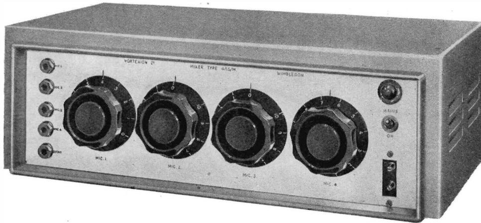
This unit has 4 built-in, balanced and screened microphone transformers, normally of 15-30 ohms impedance. It has 5 valves and selenium rectifier supplied by its own built-in screened power pack : consumption, 20 watts. Suitable for recording and dubbing, or large P.A. installations, since it will drive up to six of our 50 watt amplifiers, whose base dimensions it matches. The standard model has an output impedance of 20,000 ohms or less, and any impedance can be supplied to order.
