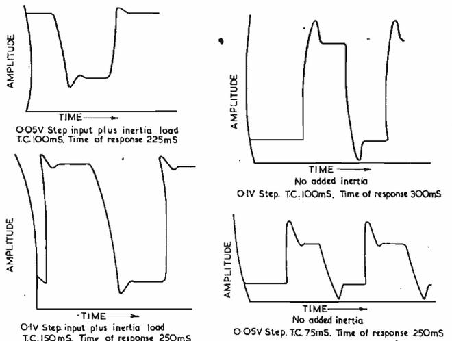
Fig. 10. Response curves of prototype (Mk II)
