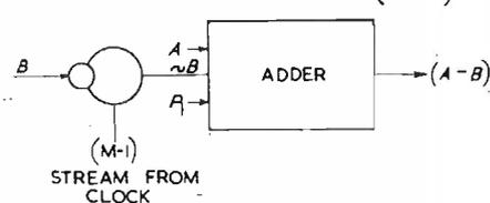
Fig. 10. Subtraction circuit
