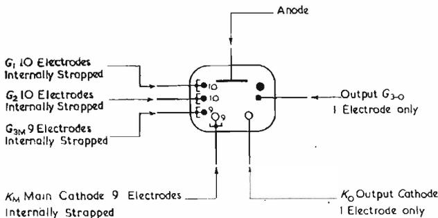
Fig. 7. Tentative signal for single pulse dekatron
