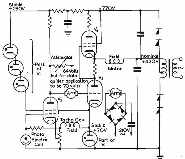
week, with occasional breaks of one hour or so for wash-down) by the introduction, where required, of stabilized resistors, stabilizing transformers, and stabilizing neons, whose long-term consistency of potential was high.
