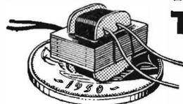
The high efficiency of these very small transformers is due to the special laminations, hydrogen annealed after stamping. Size of Transformer shown: 3/8" x 7/16" x 1/2" dia. bobbin.
