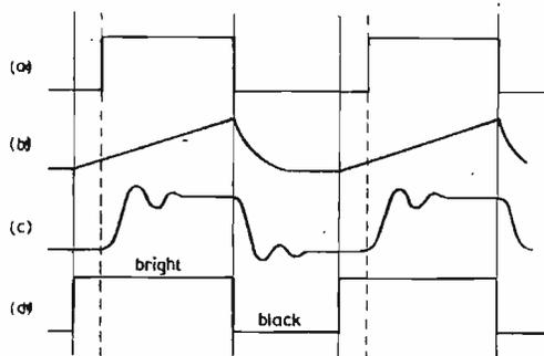
Fig. 1. Relative timing of the input square wave C.R.O. time-base, simulator response and C.R.O. blackout waveforms
