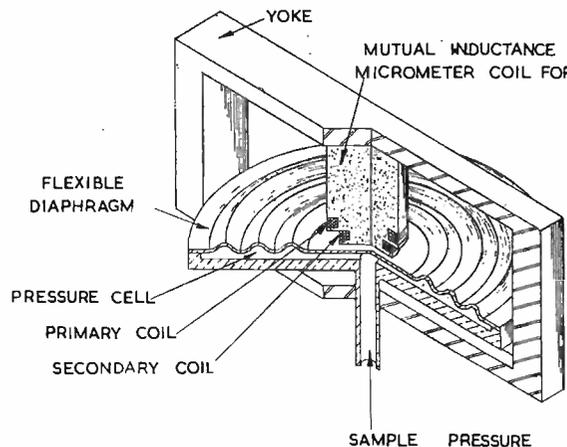
Cross-sectional view of the pressure cell.
