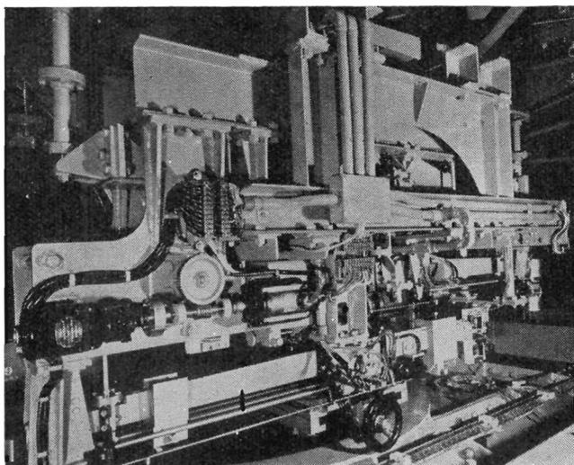
Fig. 9. Six-component wind tunnel balance
