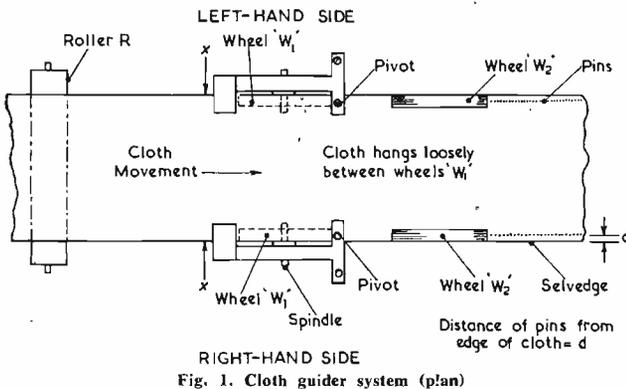
Fig. 1. Cloth guider system (plan)
