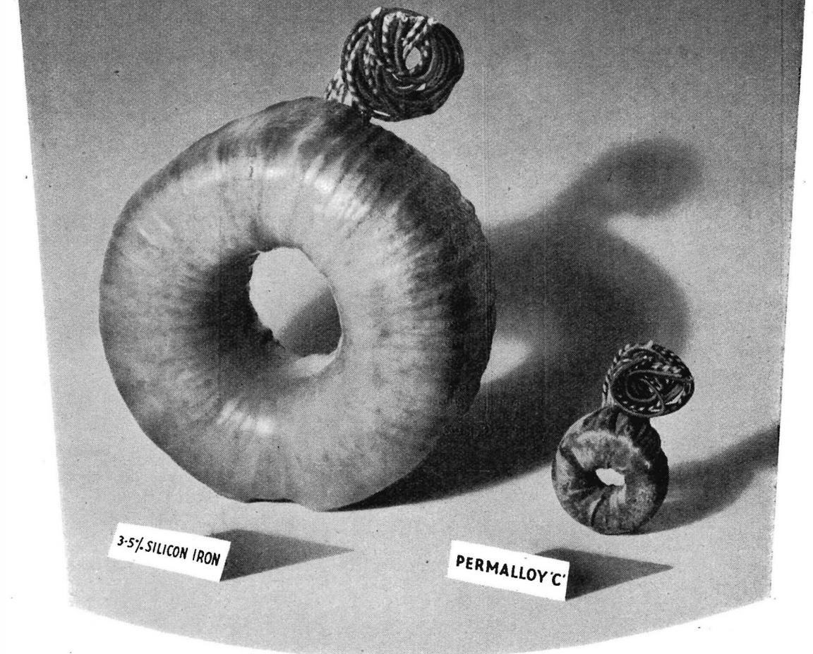
Comparison of the volumes of these two coils, 264 c.c. and 6.4 c.c. respectively, will underline the advantages of *Standard* Permalloys which have played so great a part in the technique of coil miniaturization and in the conservation of raw materials . . . 40 Permalloy 'C' Coils could be used in the same space as one Silicon-Iron coil.
