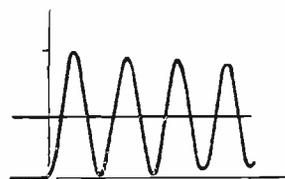
Fig. 11. Second order oscillating closed loop system
