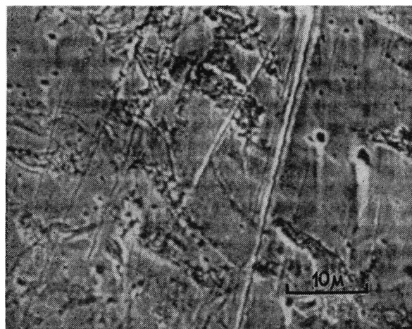
Fig. 8. Mild steel. Perpendicularly scanned, magnification \times 1500 , 15kV, 1.5 \times 10^{-10} A beam current, exposure 300 seconds
