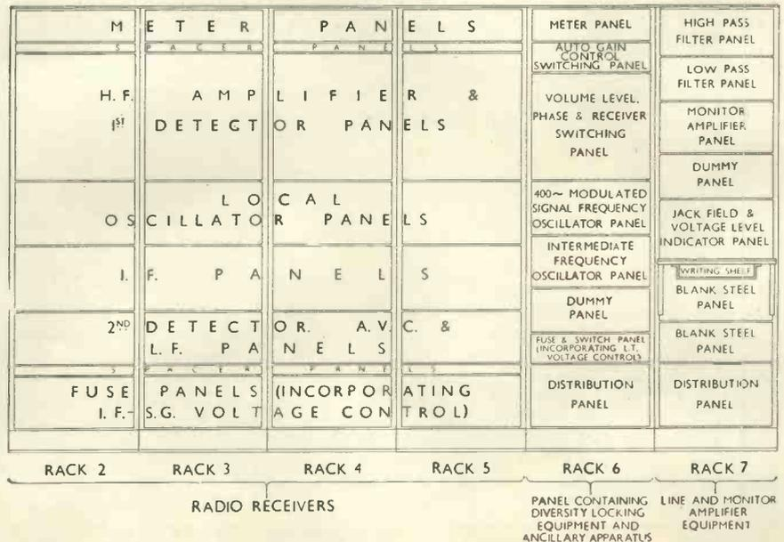
A plan of the control panel illustrated above indicating the functions of the various sections.
