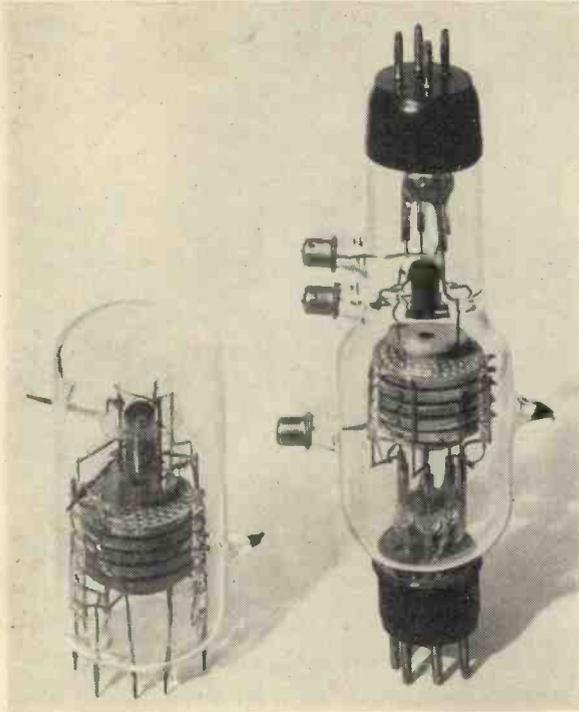
Fig. 3. Two examples of six-stage Augetrons: on the left is the footless type.
