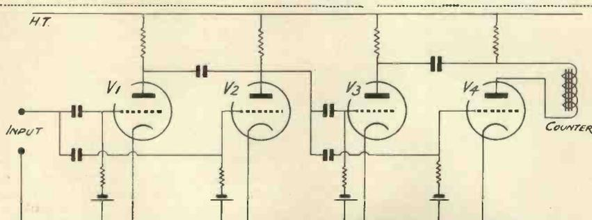
Fig. 4. The application of the circuit of Fig. 3 to counting rapid impulses.
