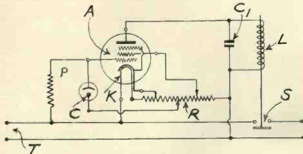
Circuit diagram of photo-electric relay. Patent No. 514,600.
