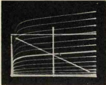
Fig. 9. Load line for the case in which the output valve is loaded with a pure resistance. The resistance here has the optimum value: the operating point lies in the middle of the section which is cut off on the straight load lines by the axes.
