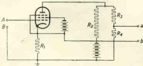
Fig. 7. First stage of the D.C. push-pull amplifiers for the deflection voltages. By giving the resistances  $R_1$ - $R_4$  suitable dimensions, upon application of an A.C. voltage to AB, the potential at  $a$  is made to increase by the same amount as that at  $b$  falls. The D.C. voltage potential at both points is adjusted to the same value by regulation of the anode direct current.
