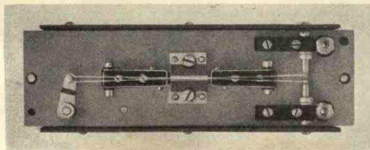
Fig. 2. Recording light-valve (Western Electric).
