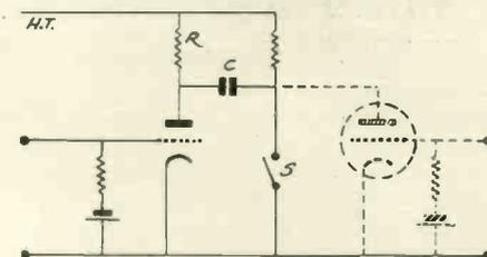
Fig. 3. Use of a condenser for breaking the circuit of a thyatron. A second thyatron acts as an automatic switch.
