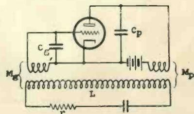
Fig. 1. Circuit of simple feed-back oscillator.
