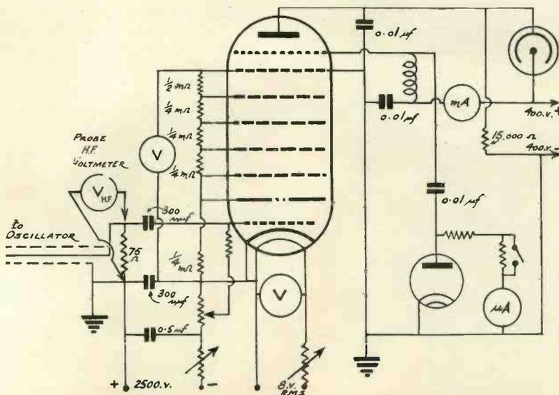
Fig. 1. Circuit diagram of the high-frequency test equipment illustrated in Fig. 2.
