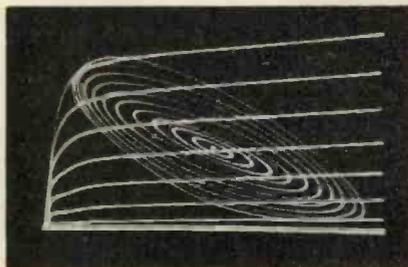
Fig. 11. With inductive loading of the output valve (connection to loud speakers) the load line becomes a more or less distorted ellipse around the operating point when the grid excitation voltage is sinusoidal. In this recording the amplitude of the grid excitation voltage was varied in steps with the frequency constant.
