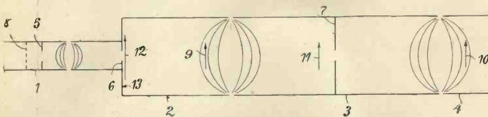
Diagram of electron microscope incorporating an electron mirror.
