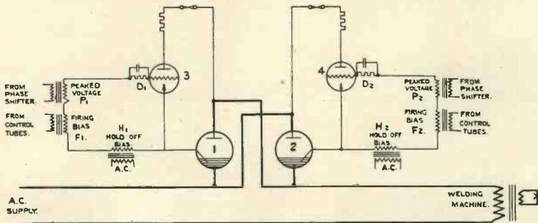
Fig. 5. Simplified circuit diagram of power circuit for ignitron welder control.
