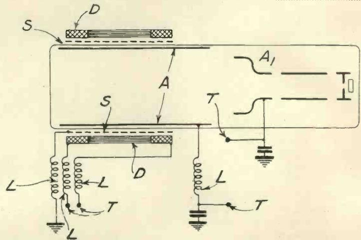
Protection against high voltages in C.R. tube deflecting coils. Patent No. 514,825.
