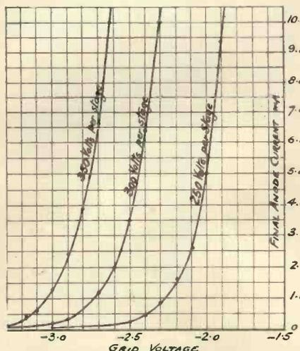
Fig. 4. The above curves of control grid voltage against output current are equivalent to the la-E<sub>g1</sub> curves of a standard valve.
