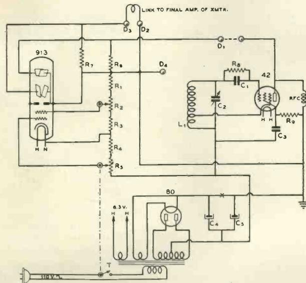
Fig. 3. Circuit diagram of the frequency monitor.
