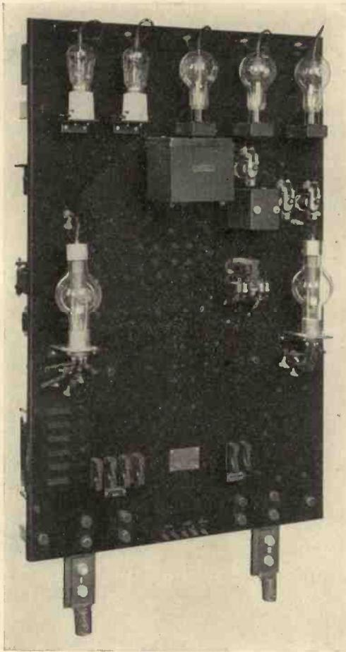
Fig. 1. Front view of B.T.H. welder control panel.
