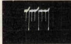
Three-to-one frequency division as shown on monitor oscillograph.
