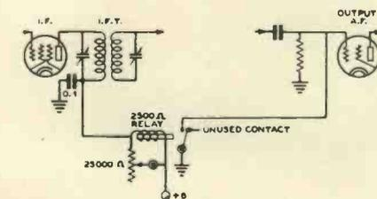
Fig. 2. Q.A.V.C. circuit using a relay.
