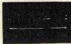
Vertical synchronising pulse superimposed on vertical blanking wave showing relative phase of the two signals.
