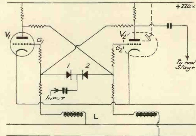
Fig. 6. A counting circuit by W. B. Lewis, using hard valves.
