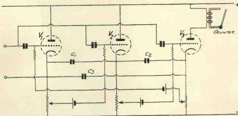
Fig. 5. The "ring" circuit for multiple counting.
