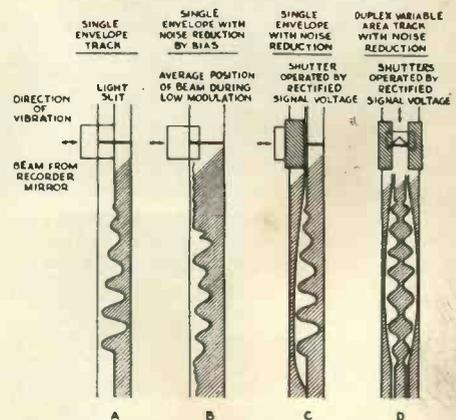
Fig. 5. Types of variable-area tracks: A single or unilateral open track; B and C with noise reduction; D bilateral or duplex track with noise reduction. (Courtesy S.M.P.E. Journal).
