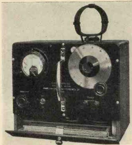
Modulation: 30 per cent. peak depth, 400 cycles. 1,000 cycles can be provided on request.
