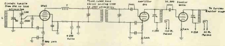
Fig. 2.— $L$  is a coil of #24 wire wound 32 turns per inch on a bakelite tube two and a quarter inches in diameter, the length of winding being two and three-quarter inches.  $T$  is the feed-back or tickler coil and consists of about six turns wound over the grounded end of  $L$ . An aluminium box contains the entire tuned circuit, grid choke and leak, coil  $T$ , and the band-pass filter.
