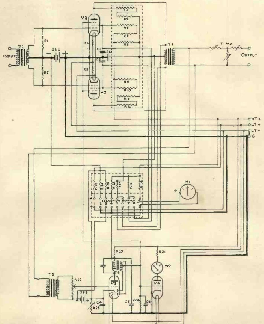
Fig. 7. Circuit of logarithmic volume-compression system. (Courtesy B.K.S. Journal.)
