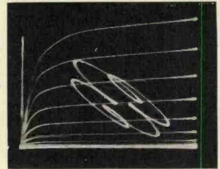
Fig. 12. Two A.C. voltages with a frequency ratio of 1:4 are applied to the grid of the inductively loaded output valve.
