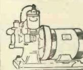
A 500-watt, Petrol Electric, single cyl. 2-stroke, water cooled, self-olling Stuart Turner engine; mag. ign., coupled to 50/70 volts, 10 amps., **£17:10:0** shunt dynamo 1,000 r.p.m.
