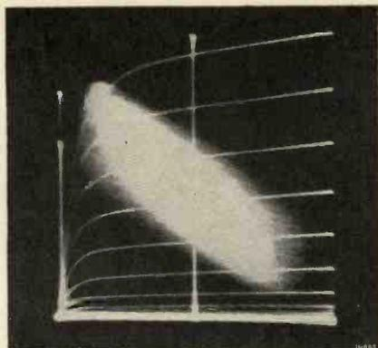
Fig. 15. The A.C. voltage of music is applied for some time to the grid of the output valve. A certain "load field" is now covered in the  $I_a-V_a$  diagram.
