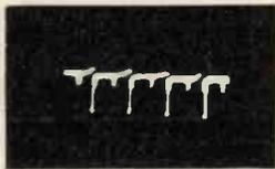
Two-to-one frequency division shown on monitor oscillograph of frequency divider.
