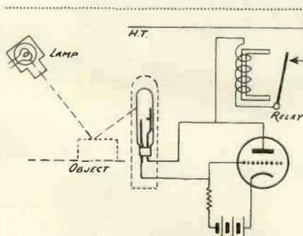
Fig. 2. Circuit for counting light flashes.
