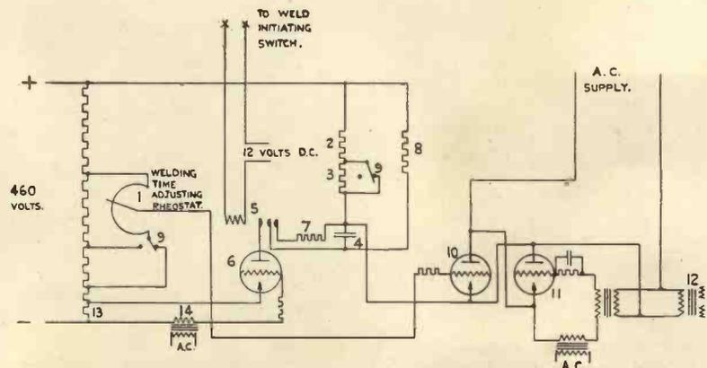
Fig. 2. Simplified circuit diagram for ignitron spot welder control.
