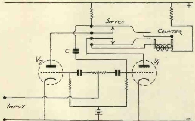
Fig. 7. "Watch-dog" circuit for storing impulses or for simple multiplication.
