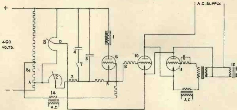
Fig. 3. Basic circuit diagram of ignitron seam welder control.
