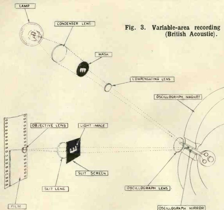
Fig. 3. Variable-area recording system (British Acoustic).
