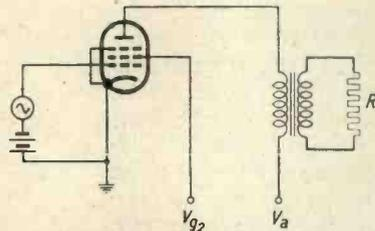
Fig. 2. A loading resistance  $R$  is included in the anode circuit of the output valve via a transformer 1:1.
