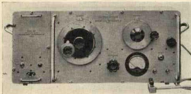
These photographs show two new Marconi-Ekco precision instruments. On the left is the type TF.517A U.H.F. Signal generator with a range of 150 to 300 Mc. (2 to 1 metres). Below is the type TF.643 U.H.F. wavemeter with a frequency range of 20 to 300 Mc.
