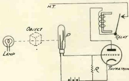
Fig. 1. Simple counting circuit operated by interrupting a beam of light on a photo-cell.
