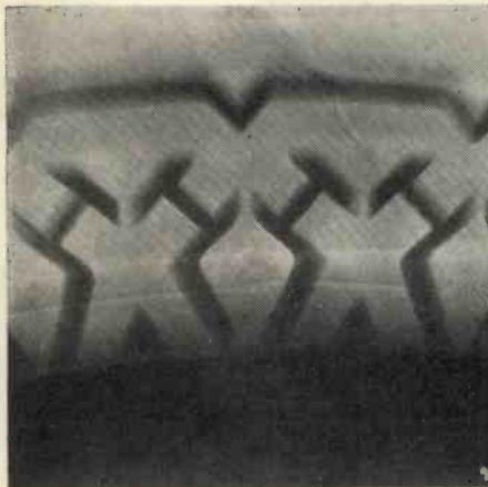
Radiograph of a motor car tyre.
