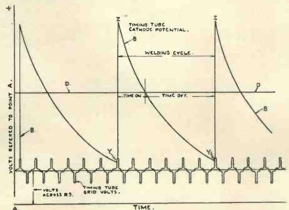
Fig. 4. Timing tube circuit voltage conditions.
