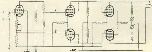
Fig. 8. Diagram of the complete circuit of the D.C. push-pull amplifiers;  $a$  and  $b$  correspond to the points  $a$  and  $b$  in Fig. 4.
