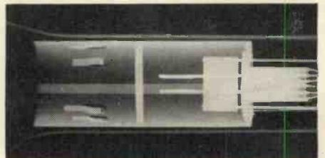
Radiograph showing positions of deflecting plates in cathode-ray tube.
