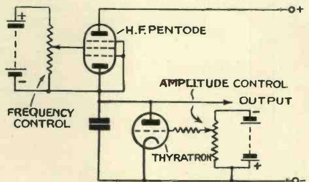
An example of a typical scanning circuit.
