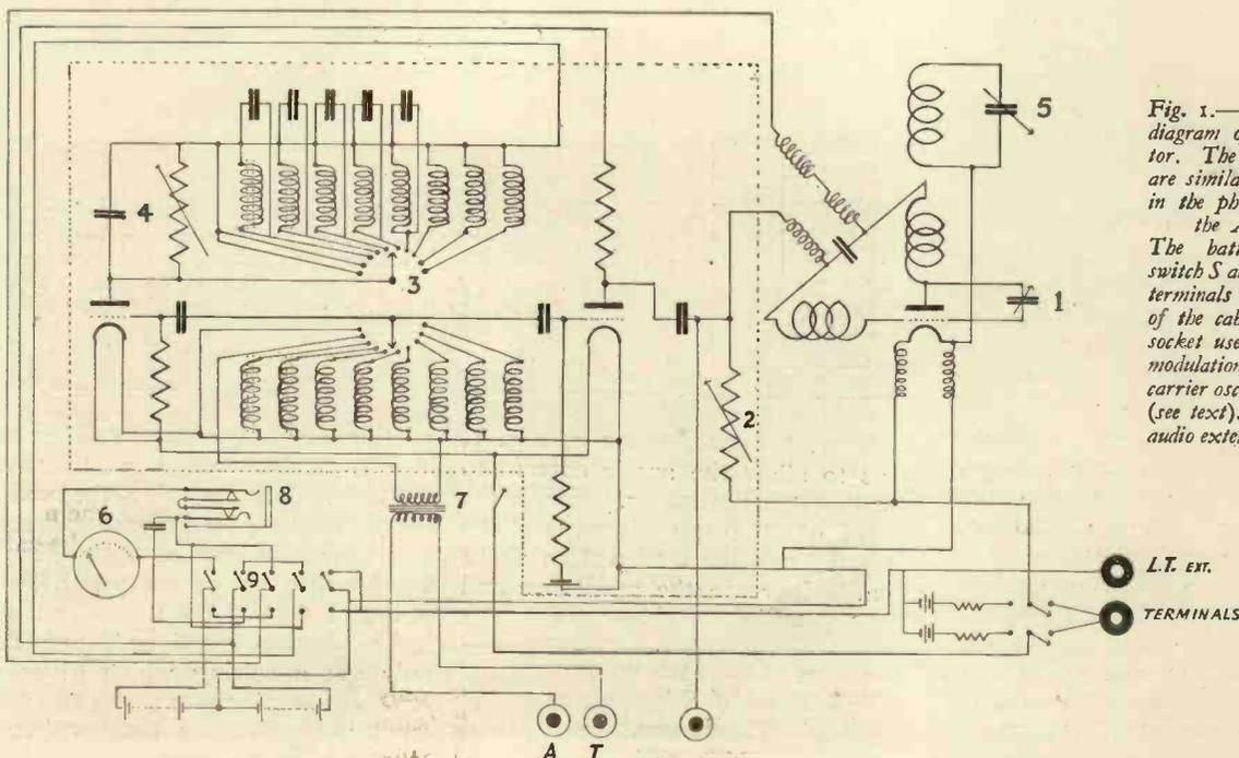
Fig. 1.—Complete circuit diagram of signal generator. The numbers 1 to 9 are similar to the controls in the photograph Fig. 1 the April issue. The battery change-over switch S and L.T. external terminals are at the back of the cabinet. T a test socket used for measuring modulation volts across carrier oscillator's grid leak (see text). A socket for audio external signal input.
