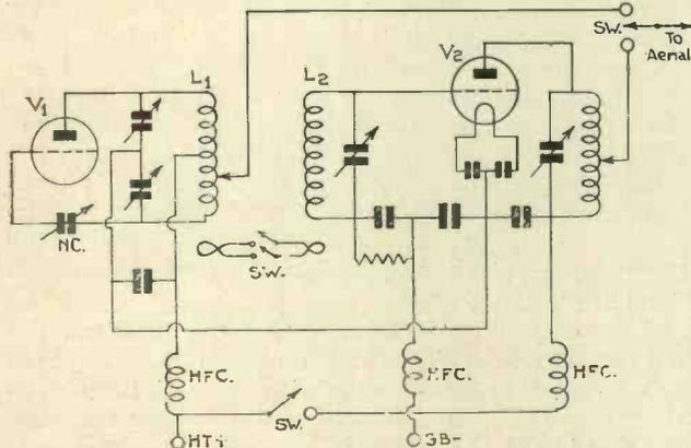
The 10-metre band is the most suitable for real DX at the moment. Try this arrangement as suggested.
