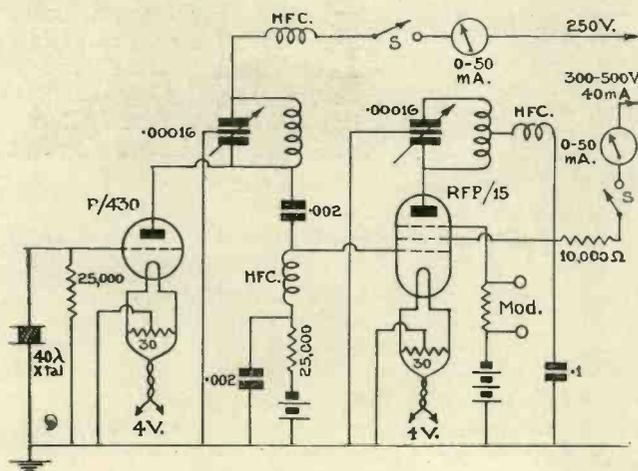
Fig. 2.—As split-stator condensers are used there is no need for anode by-pass condensers. Modulation is fed into the suppressor grid via the right hand jack. Make sure this jack is insulated from the panel. The tank coil shown is for the 20-metre band.
