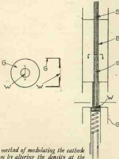
*A method of modulating the cathode beam by altering the density at the centre. (Patent No. 440,390.)*
