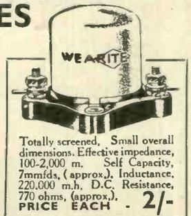
Totally screened. Small overall dimensions. Effective impedance, 100-2,000 m. Self Capacity, 7mmfd. (approx.). Inductance, 220,000 m.h. D.C. Resistance, 770 ohms. (approx.).
