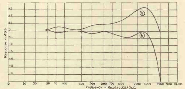
Fig. 36.—Frequency characteristics of the amplifier shown by Fig. 35.
