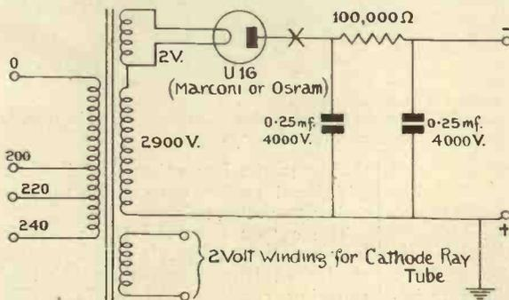
*The circuit of the cathode-ray exciter unit.*
