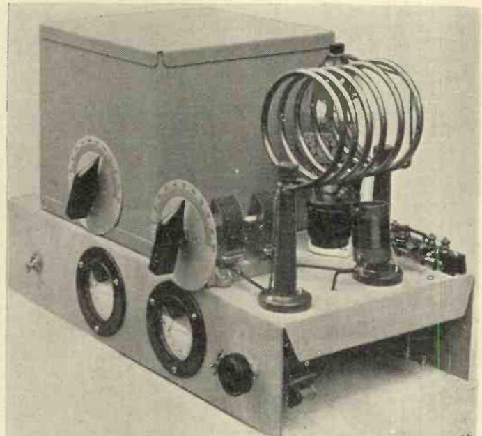
Fig. 4.—Two toggle switches are required, one in each anode circuit, so as to break the high-tension supply when required. The two meters measure the D.C. anode current.
