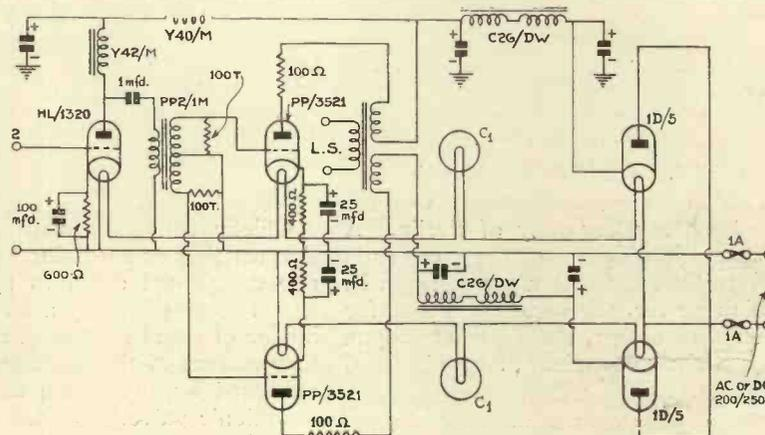
at 50 cycles and .5dB down at 15,000 cycles. This is, of course, including the output transformer. If the Baker loud-speaker is not used the bass response can be levelled up as previously suggested by the use of a 200-mfd. condenser across the cathode bias resistance.
