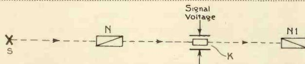
Fig. 1.—Diagram illustrating the action of a Kerr cell.
