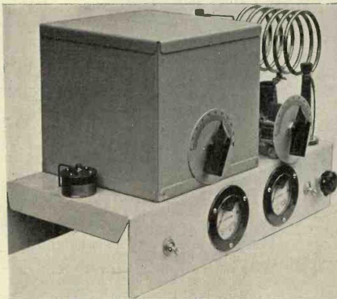
Fig. 1. The oscillator provides ample drive for the RFP-15 pentode. The resistance across the modulator input has a value of 1,000 ohms. Although satisfactory results can be obtained with only 250 volts, 500 volts must be applied to obtain 15 watts input.
