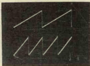
Fig. 1 (a) and (b).—The shape of the wave of deflecting voltage applied to the plates for producing the line screen.
