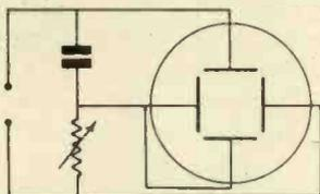
Fig. 6.—A circular trace modulated.
