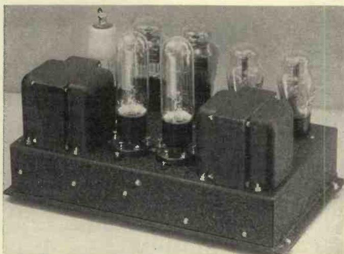
In the centre can be seen the two C1 Philips barretters. Resistances which plug in to valve holders can be used in place of the barretters which require the normal valve holder fittings.
