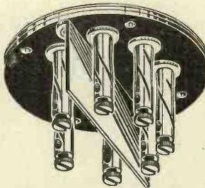
*Note the screen in these Continental type valveholders specially made by "Clix" for use with Cstar-Ganz Valves.*
