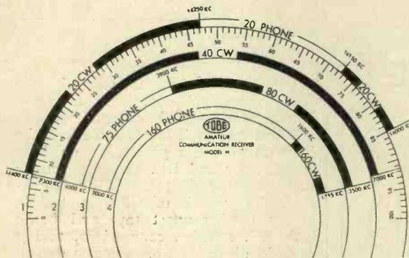
Every amateur will want a receiver using this amazing dial. The 20-metre band spreads over 6 ins. A receiver on these lines is almost completed and will be published in an early issue.
