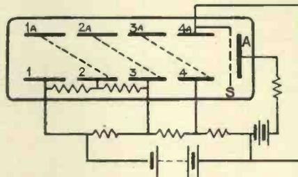
Diagram showing the operating principle of the electron multiplier.
