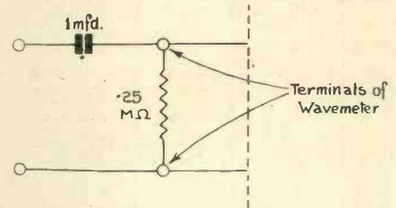
Fig. 3a (right).—Wavemeter with anode-bend rectifier as resonance indicator. The short-wave chokes (S.W.C.) consist of 55 turns of 24 S.W.G. wire closely wound on a 1/2 in. former. The dotted lines indicate complete screening. Fig. 3b (above).—Wavemeter connected to valve voltmeter.
