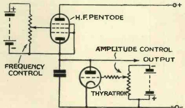
An example of a typical scanning circuit.
