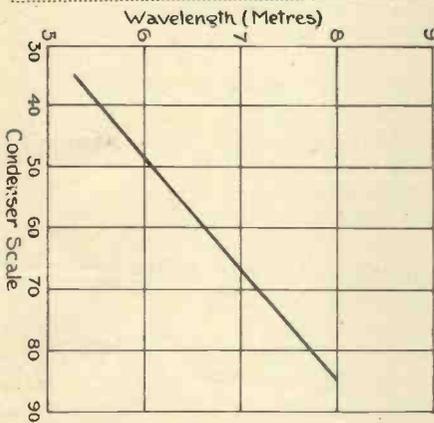
Fig. 2.—Wavemeter curve of the signal generator.
