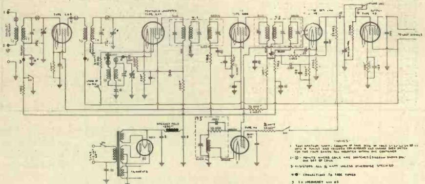
This is the circuit of the all-wave super using the standard Tobe tuner.
