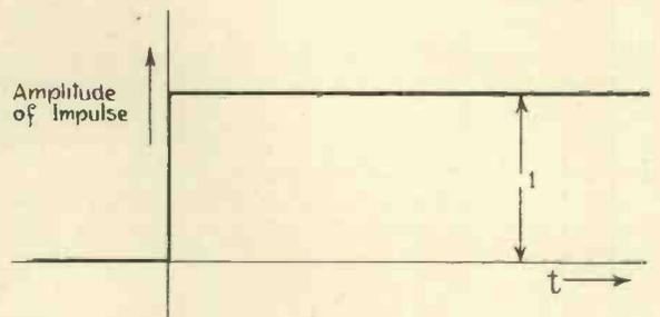
A Rule is given in an article by G. D. Robinson\* that the variation of the amplitude of the flat-topped alternating current component of the picture signal will not exceed  $\frac{50}{nCR}$  per cent., where  $C$  is the coupling capacity
