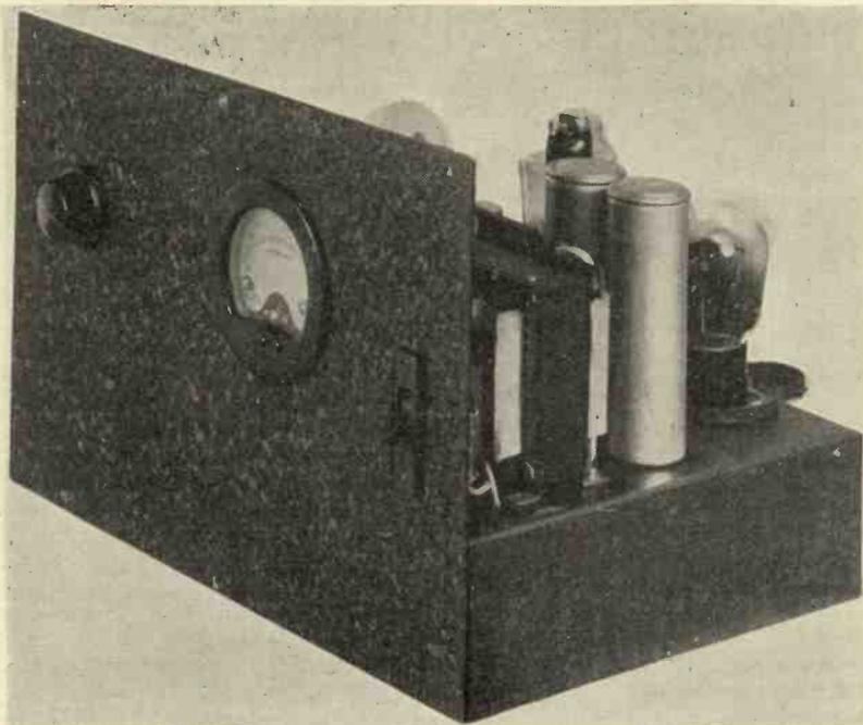
Fig. 6.—This modulator uses the high potential heater valves, while the actual output valve is a pentode giving between 3 and 4 watts on either A.C. or D.C.
