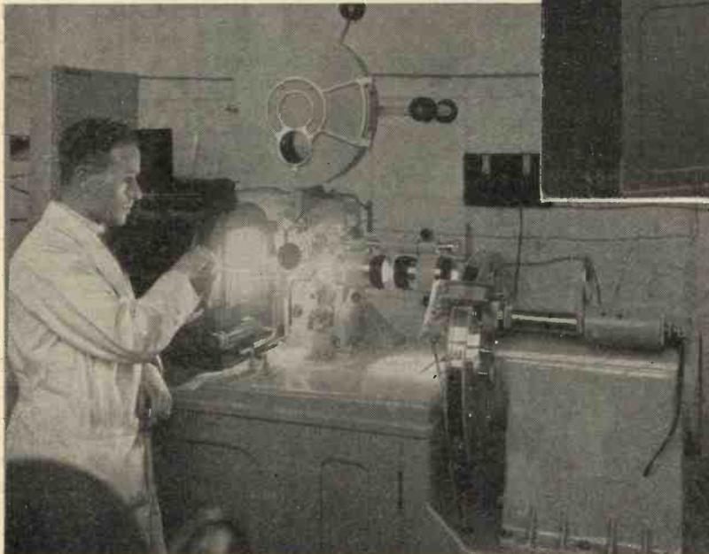
vacuum, photo-electric cell and A & B amplifiers in the large consoles. Below the projector box contains automatically controlled vacuum and water cooler pumps. Below the amplifier is the all-mains supply unit and behind the switchboard are the controls and sound panel. The photograph below shows the transmitter in greater detail.
