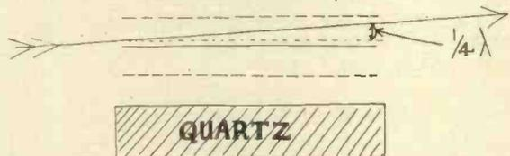
Fig. 3.—Oblique passage of light ray between supersonic wave crests.
