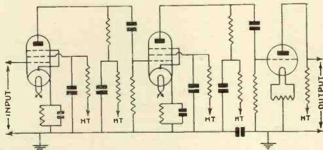
Fig. 35.—A circuit of pentodes in cascade followed by an output valve.
