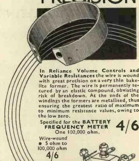
In Reliance Volume Controls and Variable Resistances the wire is wound with great precision on a very thin bakelite former. The wire is permanently secured by an elastic compound, obviating risk of breakdown. At the ends of the windings the formers are metallised, thus ensuring the greatest ratio of maximum to minimum resistance values, owing to the low zero.
