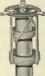
This simple little coil will be found to be of the utmost value in super-heterodyne receivers using 465 k.c/s. L.F. where no pre-l.c. H.F. stage is used. It requires no extra tuning, but resonates with the average aerial capacity to prevent the reproduction of repeat whistles, etc. Accurate wave-windings are spaced on a special impregnated former, and a bakelite plate carries tags for connections. Complete with full instructions.
