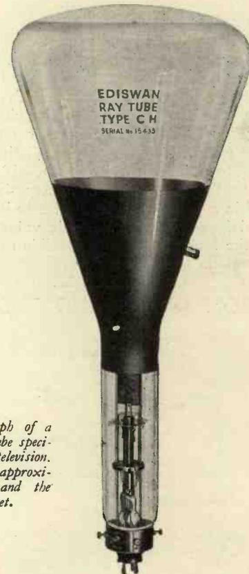
*This is a photograph of a typical cathode-ray tube specially manufactured for television. The screen diameter is approximately 10 inches and the total length 2 feet.*
