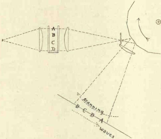
Fig. 1.—Diagram explaining simultaneous production of fifty picture details on the receiver screen.
