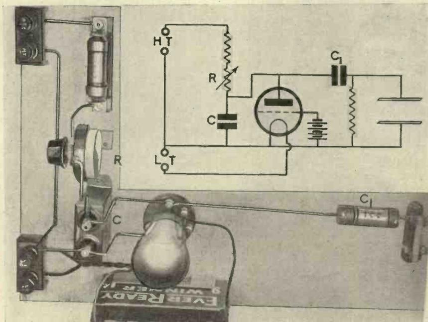
Fig. 2.—The simplest form of scanning circuit comprising a condenser and resistance with a relay for discharging the condenser.
