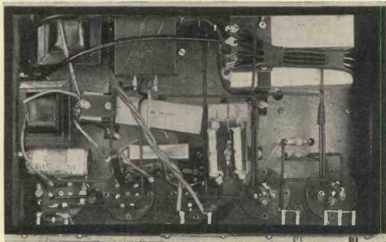
The under baseboard wiring is comparatively simple and if wires are braided together as shown it helps to preserve neatness.
