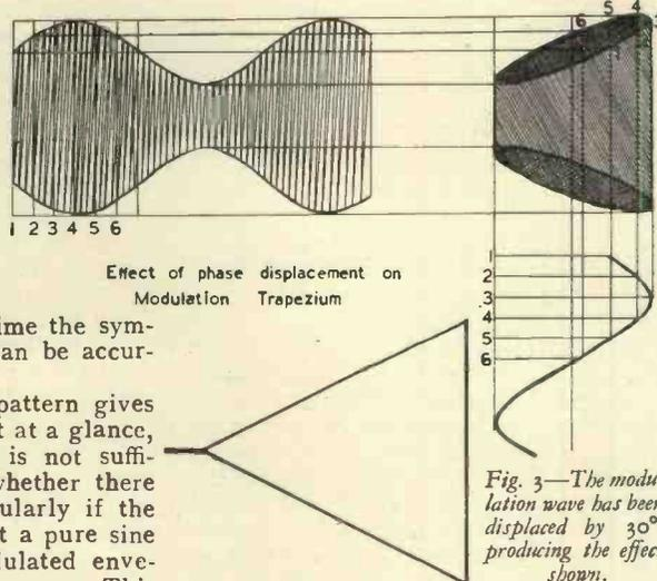
Fig. 3.—The modulation wave has been displaced by 30°, producing the effect shown.
