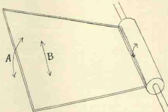
Fig. 11.—Flat sheet of light produced by high speed scanner.
