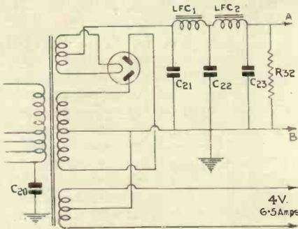
Fig. 7.—The power pack is conventional as can be seen from this circuit.
