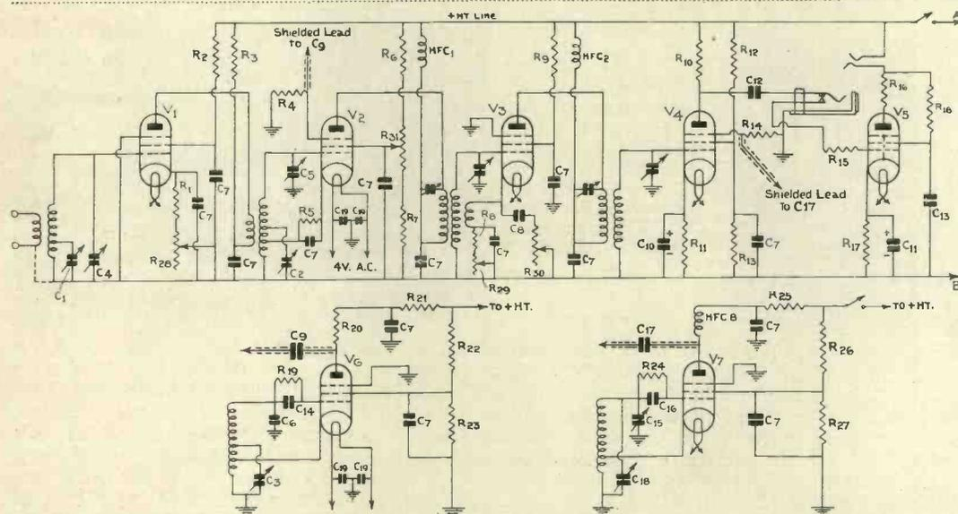
Fig. 5.—There are no complicated components in this circuit even though it uses all the features the amateur requires for good DX reception.
