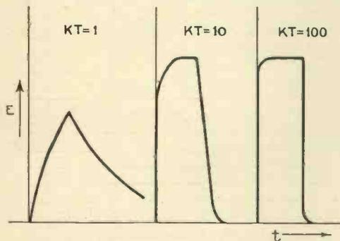
Fig. 39 (left).—The form of distortion due to high-frequency cut-off.
