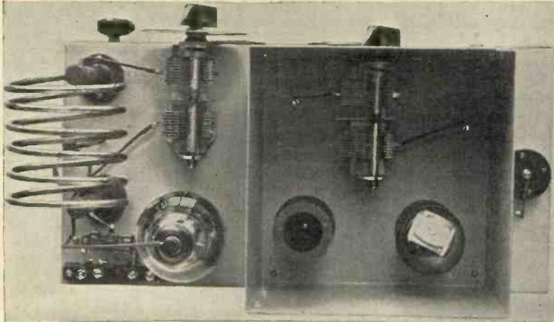
Fig. 3.—If the C.O. section is screened in this way there is no tendency for one circuit to pull the other. The Brookes crystal can be seen on the extreme right.
