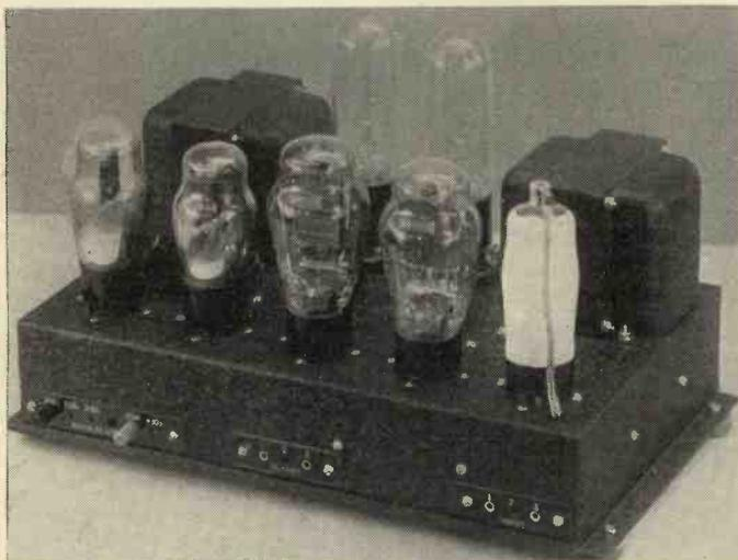
Valves are from left to right two ID<sub>5</sub> half-wave rectifiers, two PP3521 triodes, and an HL1320 medium impedance triode.
