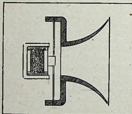
Fig. 1.—Cross-sectional drawing of an ordinary carbon microphone.
