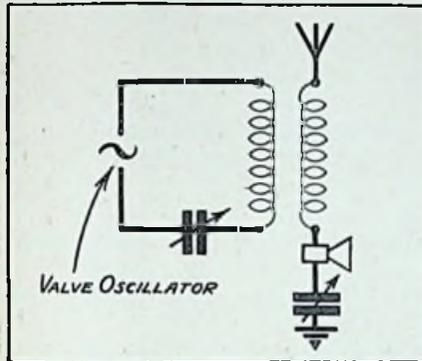
Fig. 3.—Circuit diagram of a wireless transmitter showing the simplest possible manner of connecting a microphone to modulate the transmitted wave.
