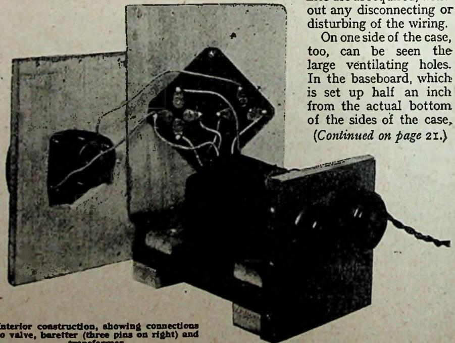
Interior construction, showing connections to valve, baretter (three pins on right) and transformer.
