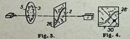
chronised scanning discs (5) in Fig. 3 having zig-zag arranged slots (3) in place of the usual spiral arrangement of holes. At the receiving station (Fig. 4), the intersection of two luminous lines (30) indicates the position of the luminous spot (2) on the transparent map (26) at the transmitter.
