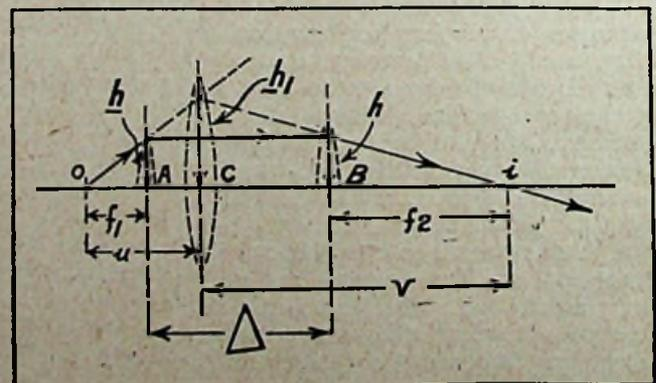
Fig. 2.—Solution of magnification problem by use of equivalent refracting surface.
