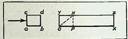
If, however, one of the "teeth" of the interrupter disc traverses *YHPO* in the opposite direction to that in which *abcd* is moving, then I contend that the amount of distortion will be much reduced. The same sort of thing will occur at the other end.
