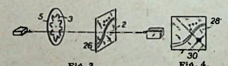
chronised scanning discs (5) in Fig. 3 having zig-zag arranged slots (3) in place of the usual spiral arrangement of holes. At the receiving station (Fig. 4), the intersection of two luminous lines (30) indicates the position of the luminous spot (2) on the transparent map (26) at the transmitter.
