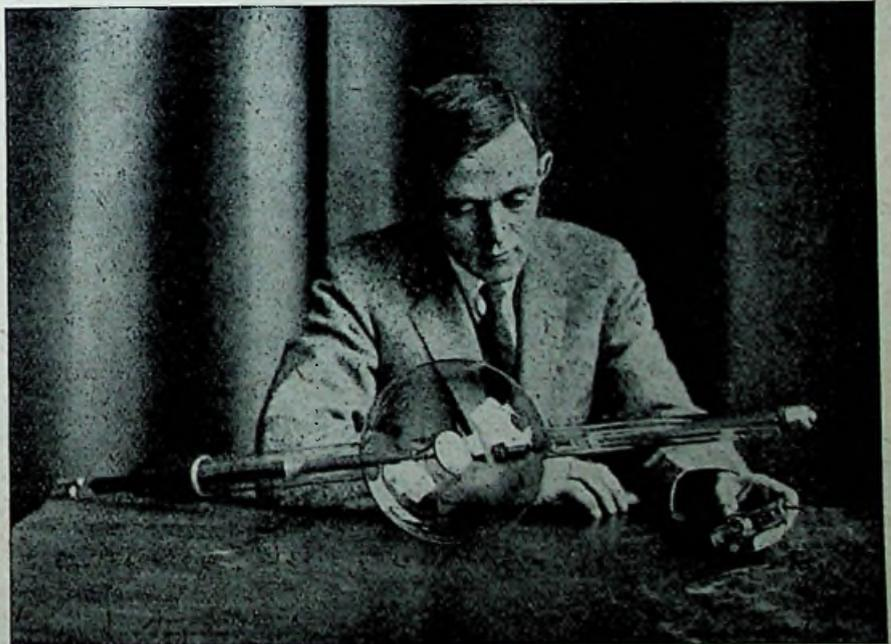
A large Coolidge X-ray tube, photographed beside one of the smallest tubes (in left hand of figure).
