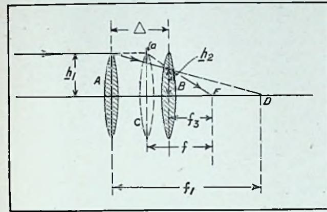
Fig. 3.—Ray diagram for two separated lenses imaging a distant object-point.
