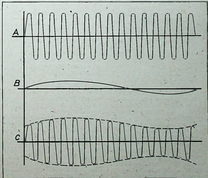
Fig. 4.—How the wireless wave is modulated.
