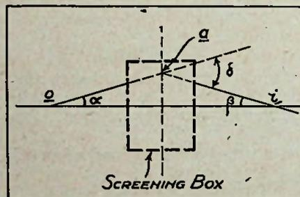
Fig. 1.—Diagram showing the derivation of an equivalent refracting plane for a lens system.
