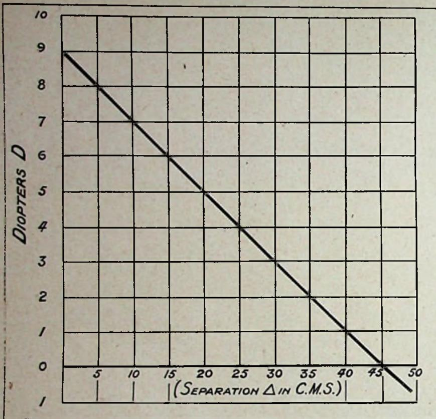
Fig. 5.—Graph for combination of two lenses, +5 D and +4 D, with variable separation.
