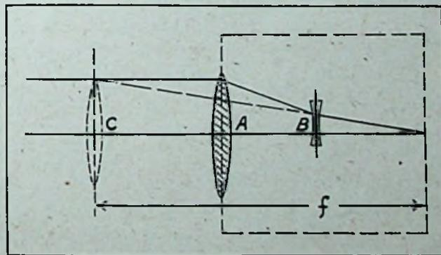
Fig. 4.—The optical action of a telephoto lens.
