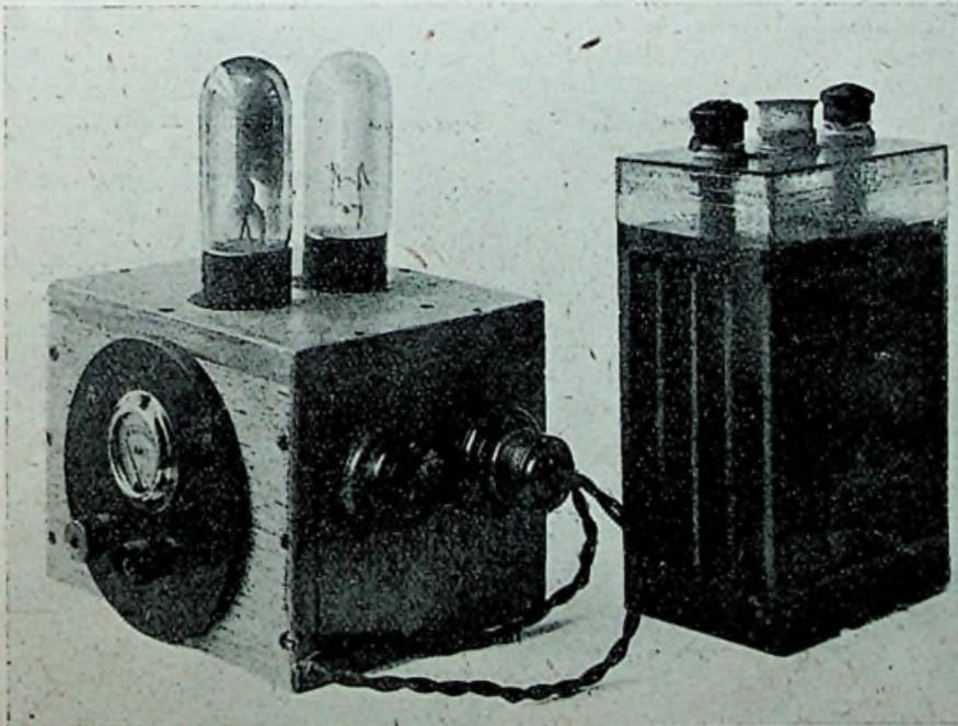
The rectifier with 2-volt 20 amp.-hour accumulator beside it. The buretter is the clear valve at the back. There are also shown the plug connection to the mains, switch, and output terminals with ammeter above them.
