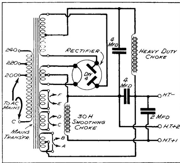
Fig. 2. Circuit of the H.T. eliminator.
