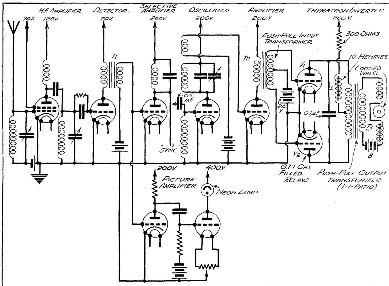
Fig. 2. The synchronising circuit described in the text.
