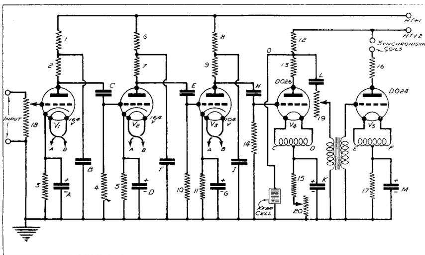
Fig. 1. Schematic circuit of the straight-line amplifier.
