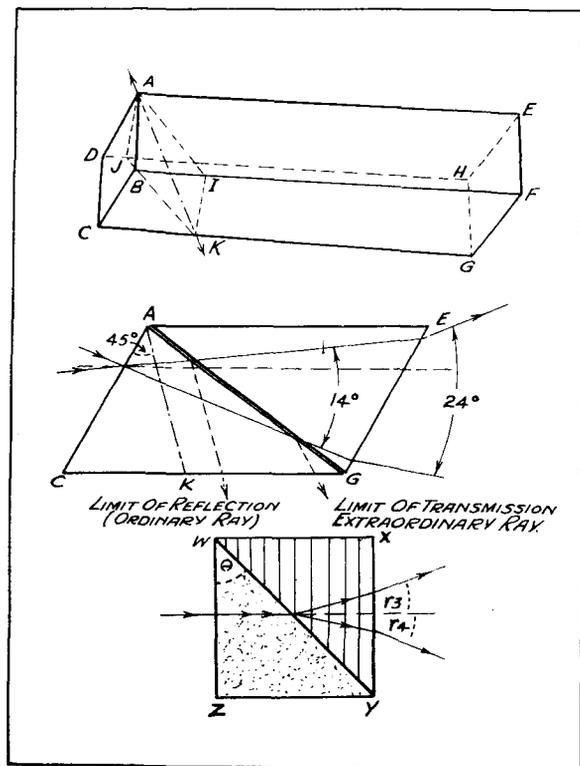
Fig. 1 (Top) Effect given by a natural crystal of Iceland Spar. Fig. 2 (Centre) Nicol's scheme for cutting the crystal. Fig. 3 (Below) Woollaston's prism.
