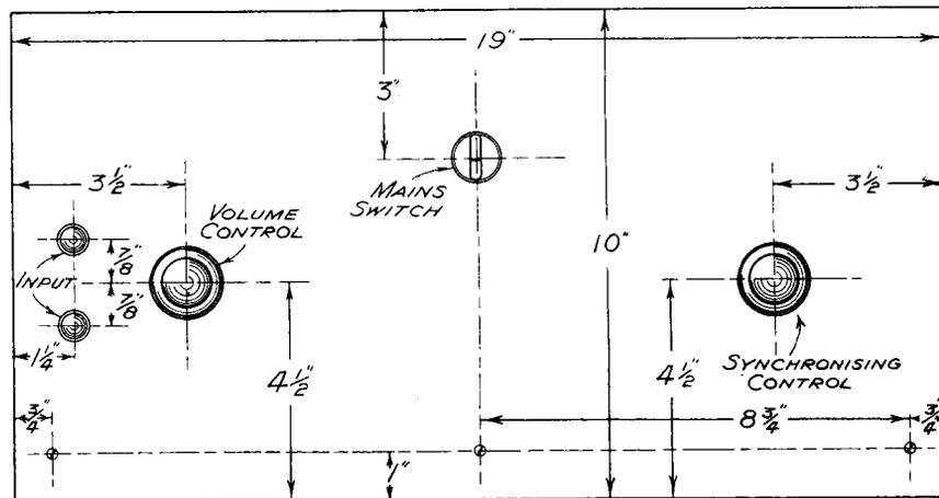
Diagram of the panel of the straight-line amplifier.
