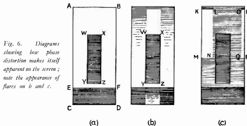
Fig. 6. Diagrams showing how phase distortion makes itself apparent on the screen; note the appearance of flares on b and c.
