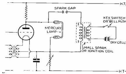
An output circuit with provision for striking the tube by pressing a button.
