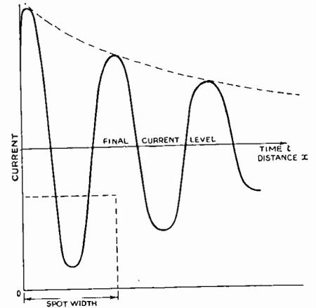
Fig. 2. Relation between amplitude of oscillation and spot travel.
