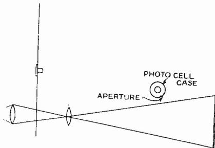
Fig. 3. Position of photo-cell relative to the subject being scanned.
