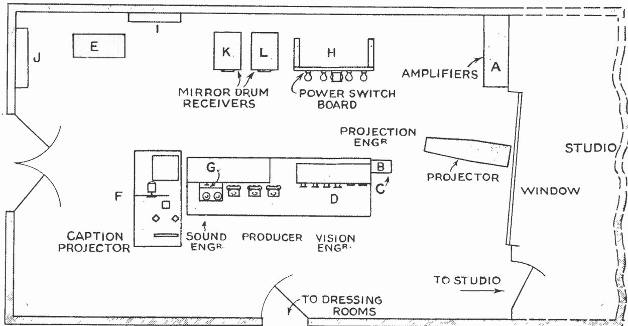
*Fig. 2. A plan of the control room from which the positions of the various units can be clearly seen. Reference to the photograph on the opposite page and the text will enable all these to be identified.*
