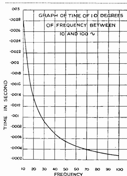
Fig. 5. Graph of the time period of 10 degrees for frequencies from 10 to 100 cycles.
