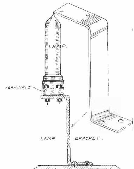
The special Nu-Glow neon lamp on its bracket; the actual bracket is shown separately on the right.
