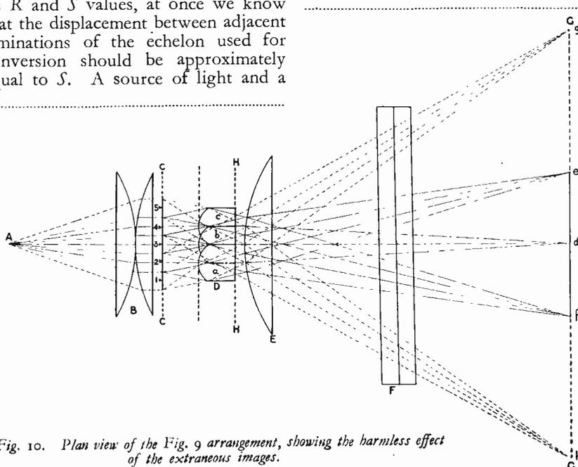
Fig. 10. Plan view of the Fig. 9 arrangement, showing the harmless effect of the extraneous images.
