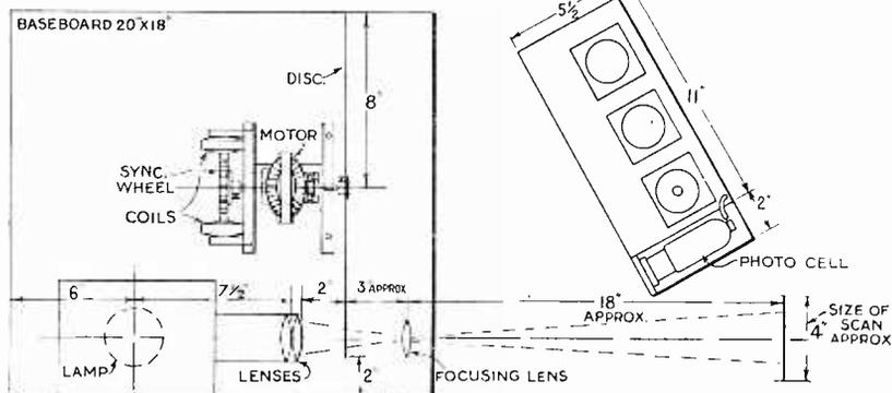
This diagram shows the arrangement of the scanner, subject and photo-cell with amplifier.
