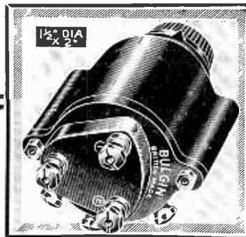
Variable Resistances and Potentiometers rated at 3, 4 and 5 watts, with and without switch. A 5-W. type is illustrated; values are available from 2,000—100,000 Ω. All wound with finest iron-free nickel-alloy wire. Dustproof moulded cases. Silent and reliable.
