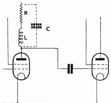
Fig. 2. Circuit for maintaining the upper frequencies.
