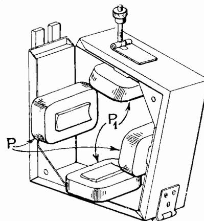
*A deflecting system for use with the cathode-ray tube.*
