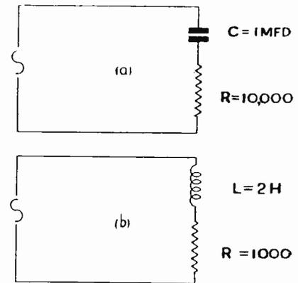
Fig. 2a. Condenser in series with resistance.
