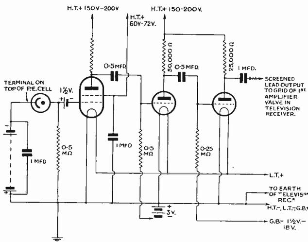
Fig. 2. Circuit showing the amplifier and photo-electric cell.
