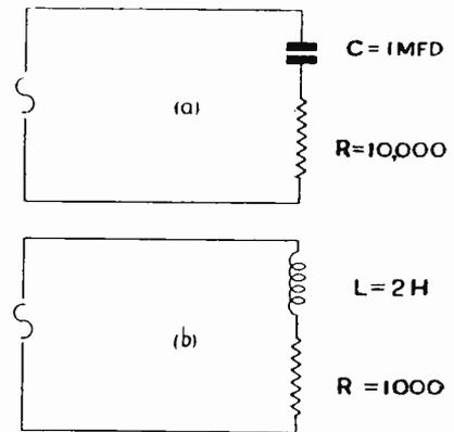
Fig. 2a. Condenser in series with resistance.
