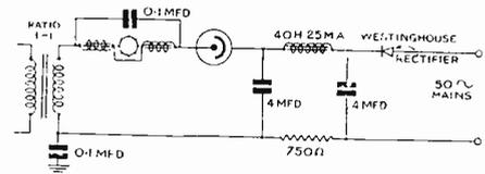
Method of lighting the neon lamp from a separate source: this diagram includes the synchronising circuit and if this is not used the connection should go straight from the neon lamp to the transformer.
