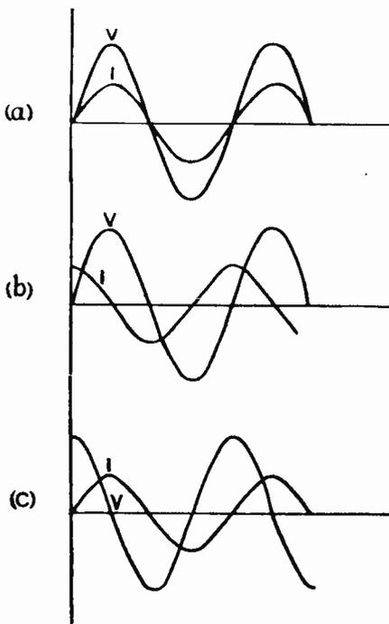
Fig. 1. Curves showing phase lead and lag.
