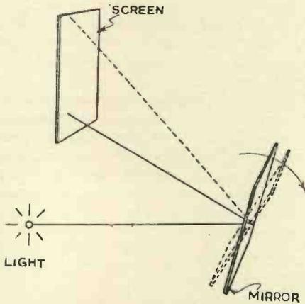
Fig. 1. A simple experiment to determine the correct arrangement of the mirrors of the screw.
