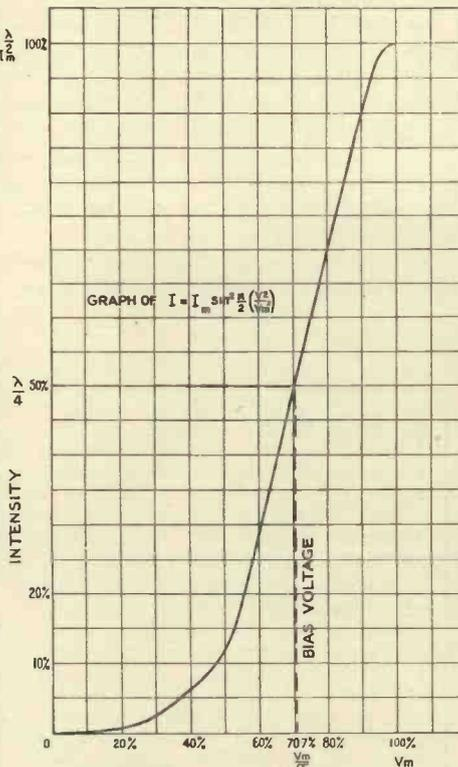
A voltage-intensity graph of a Kerr cell.
