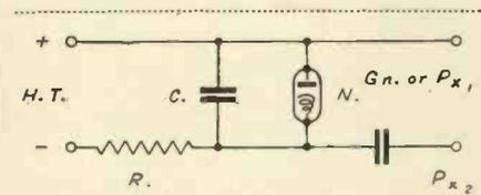
Fig. 4.—A simple time base circuit using a neon lamp.
