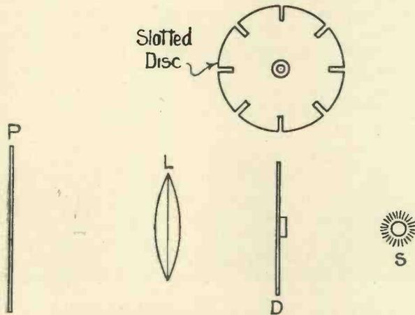
Fig. 3. A schematic diagram showing the layout of the light chopper.
