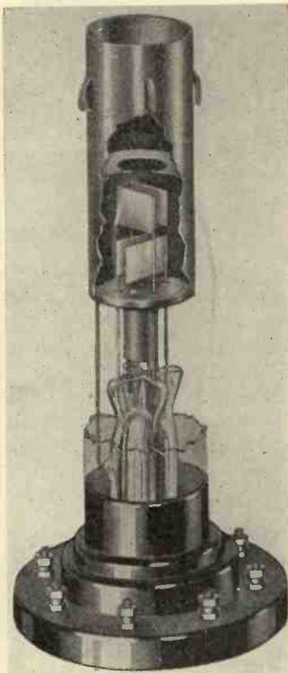
*A cut-away view of the Cossor cathode-ray tube showing the arrangement of the electrodes.*
