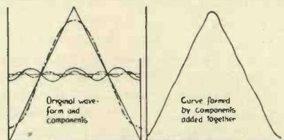
Fig. 1. The components of a triangular waveform and (left) the resulting figure.
