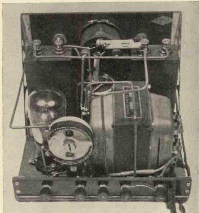
Fig. 2. — This plan view shows the arrangement of the components behind the panel, and it will be easily possible to identify these by reference to the adjoining list of components and the circuit diagram which was given in last month's issue.
