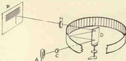
This diagram shows the working principle of the Mihaly stationary mirror-drum receiver.
