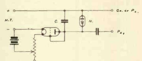
Fig. 5.—A time base incorporating a saturated diode to provide a more linear effect.
