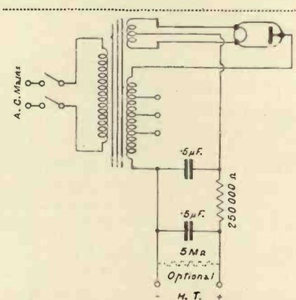
*Fig. 2.—A circuit of a simple eliminator with resistance smoothing for the high-tension supply.*
