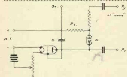
Fig. 6.—This diagram shows the addition of a synchronising circuit to the time base of Fig. 5.
