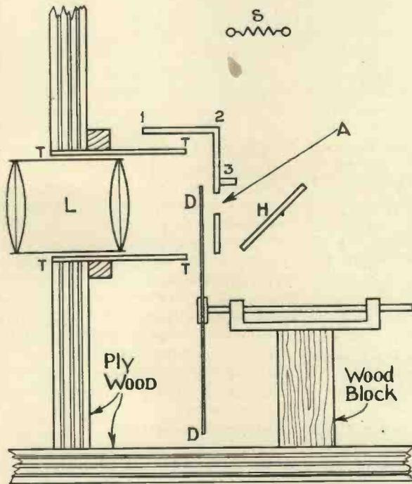
Fig. 5. This diagram shows the construction of the light chopper and the relative positions of the parts.
