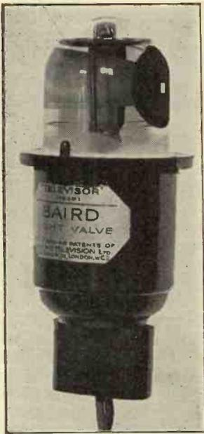
An example of an efficient grid cell—the Baird.
