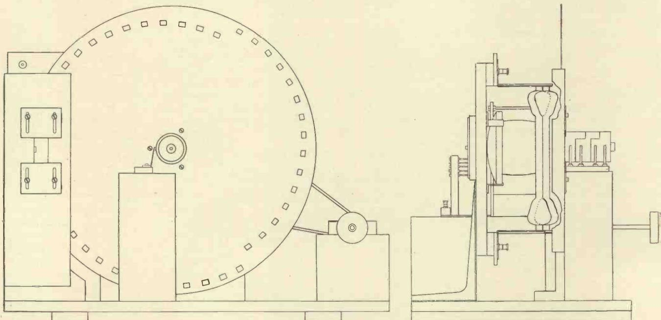
*These drawings are side and end elevations of the Baird colour television receiver.*
