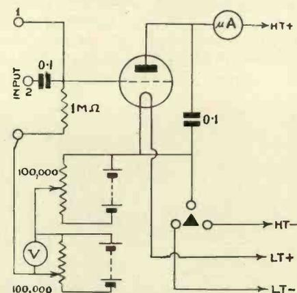
*Circuit of the simple slide-back valve voltmeter described in the text. Owing to its extreme flexibility it should find many uses in the experimenter's laboratory.*
