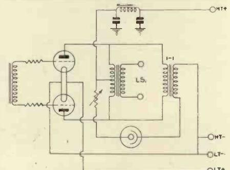
Fig. 5.—Showing the connections when the receiver has push-pull output.
