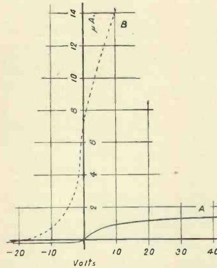
Fig. 3.—Typical current/voltage curve for a deflector plate, the other three plates being strapped on to the gun. Deflector Plate Current at 50μA Gun Current. Curve A: Shielded Structure. Curve B: Similar structure without Shield.
