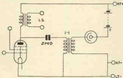
Fig. 2.—Method of connecting the neon to a commercial receiver through a 1-1 isolating transformer.
