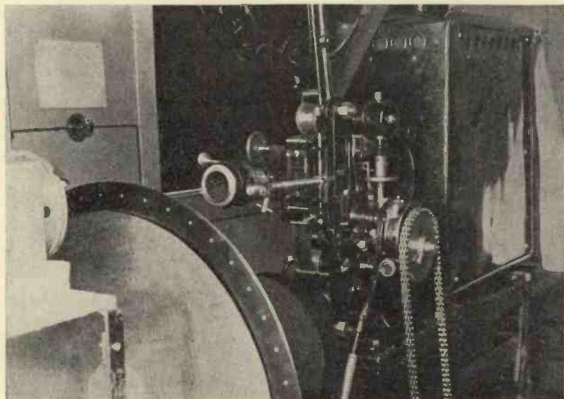
The 50-line experimental transmitter used by the International Television Corporation for test purposes. The disc and film are driven by two separate synchronous motors.
