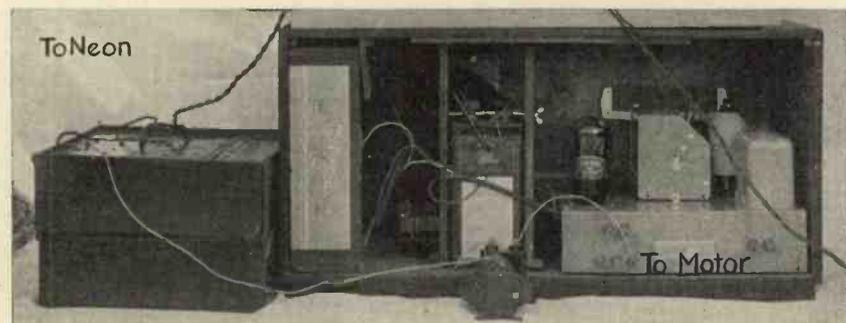
*A back view of the Halcyon Battery Three connected to a disc receiver; the output choke and condenser can be seen in the foreground.*
