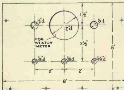
Fig. 1.—The drilling diagram of the front panel.
