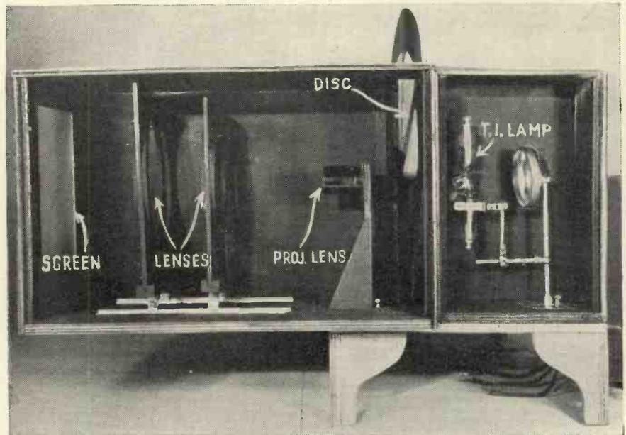
This photograph shows the assembly of the complete optical unit including lamp and screen; the disc revolves in a space between the two boxes.
