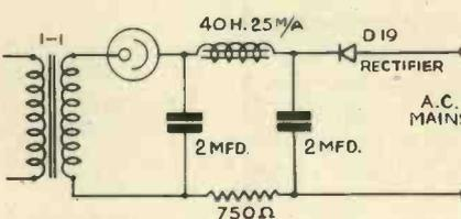
It is an expensive hobby running a neon lamp from dry batteries, so if you have mains laid on use a metal rectifier of the half-wave. Don't forget the small resistance in series with one side of the supply.
