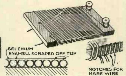
SECTION OF CELL USING ENAMELLED WIRE
