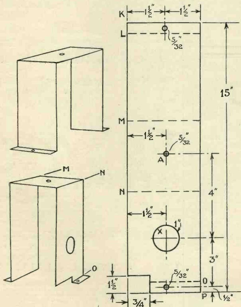
Fig. 1. Details of shield for enclosing the lamp.
