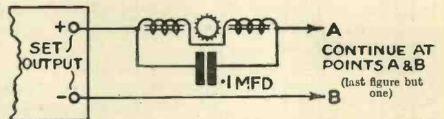
This simple synchronising circuit should be used in connection with the last figure but one and connected as indicated. It is again a simple arrangement that will keep your pictures steady.
