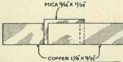
Details of the copper plates and insulation.
