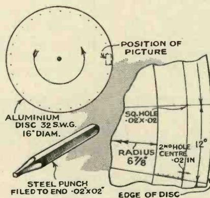
These drawings give all the necessary details to enable an amateur to construct a scanning disc.
