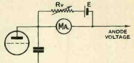
Fig. 3.—Circuit showing a method of increasing the sensitivity of a valve voltmeter.
