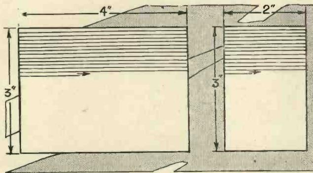
Fig. 1. A 180-line picture with a 4-to-3 ratio contains 43,600 picture elements. Half the normal picture with 2-to-3 ratio and 90 lines contains 5,450 elements.
