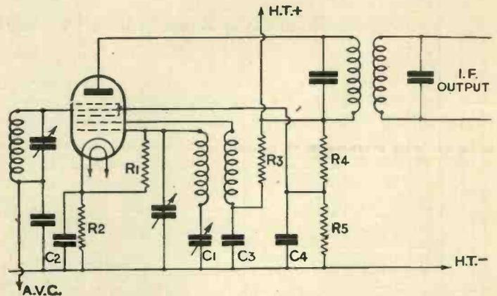
Fig. 4.—You can do away with a mains transformer and use this circuit on either A.C. or D.C. mains, providing you have an Ostar-Ganz high voltage pentagrid.
