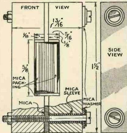
A condenser type of selenium cell built up from copper foil and mica.
