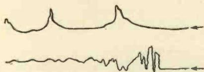
Fig. 6.—Waves of explosion pressures obtained by the crystal device. These waves are read from right to left.
