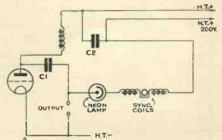
This is a simple circuit which makes use of a pair of synchronising coils. It is better for use with commercial sets when the internal connections are not accessible.
