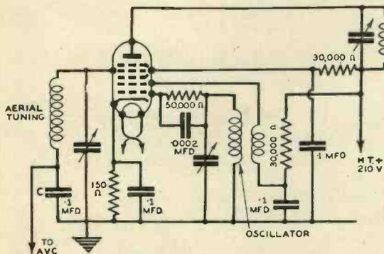
Fig. 6.—Cossors have developed this special circuit for use with their mains pentagrid. It can be added to almost any conventional super-het.
