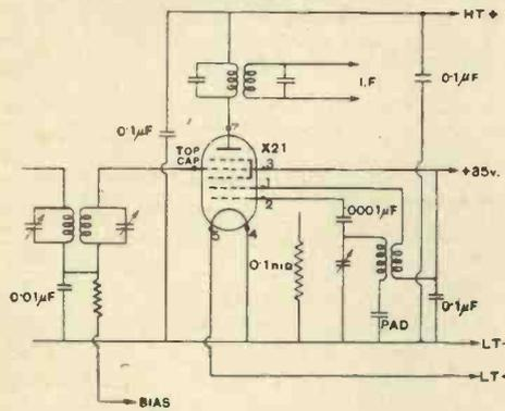
Fig. 3.—This is a good circuit in which to use your battery & heptode. Varley make special coils for the X21.
