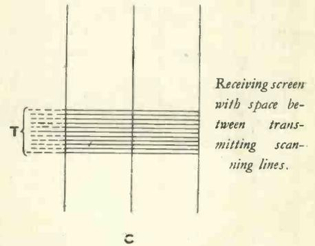
Fig. 2. Three diagrams showing the effect of spacing the transmitting scanning lines.
