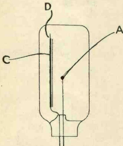
A glow lamp with part of the cathode coated with a substance having a lower extinction potential than the rest of the cathode. Patent No. 412,024.
