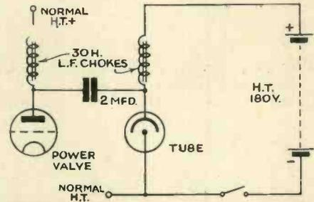
If you use a commercial receiver where the connections are difficult to get at, this is the circuit to use. The output from the power valve is fed to the neon lamp through a large fixed condenser. An extra battery is required to bring the voltage up to over 180 volts.
