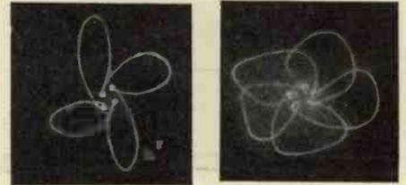
Fig. 7.—Two pretty patterns obtained by oscillatory circuits connected to the deflector plates.
