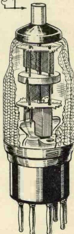
Fig. 5.—Talking about double diode triodes, this is the way the Ostar Ganz people make their version of this valve. You can see that the diodes are carefully screened from one another.
