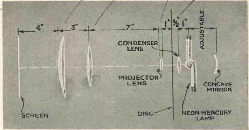
Diagram showing the arrangement of the optical system.
