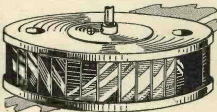
This sketch shows how the drum is assembled ready for filling with plaster.
