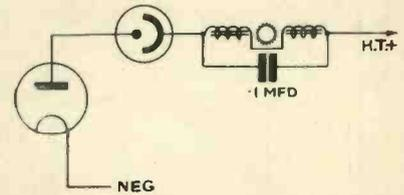
A simple circuit that will keep your pictures steady. The synchronising gear is quite standard and consists of two synchronising coils and a phonic wheel.
