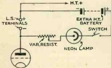
Better definition is obtained if the voltage applied to the neon is varied by means of a resistance. The additional battery in this case should be large enough to cause the neon lamp to strike with the resistance only half in circuit.
