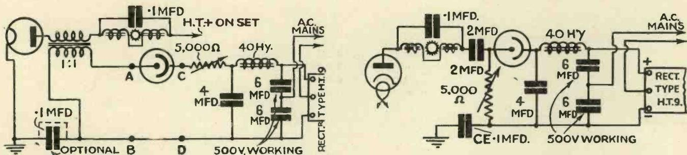
Over 300 volts can be obtained from this power pack so the output is enough to feed both the neon and the output valve. The usual variable resistance is included to improve the definition from the neon lamp.
