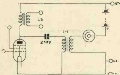
If you are troubled with reverse pictures, this circuit is worth considering. The images can be reversed by altering the transformer connections. The extra battery should be about 100 volts.
