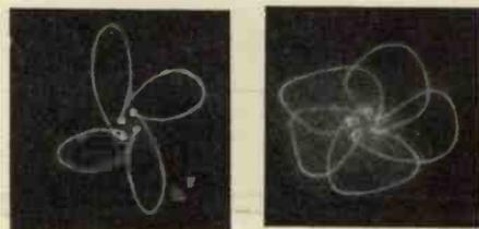
Fig. 7.—Two pretty patterns obtained by oscillatory circuits connected to the deflector plates.
