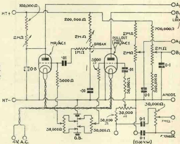
Fig. 2.—Alterations to double time base for recording wave forms.
