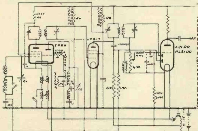
Fig. 1.—This is a good circuit that uses a double diode triode valve for rectification, low-frequency amplification, and provides automatic volume control.
