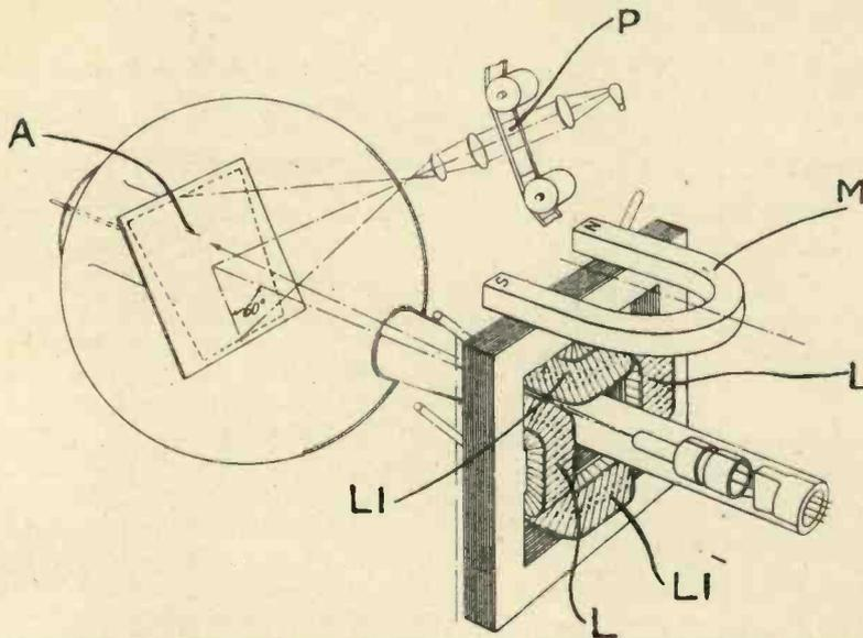
Arrangement of cathode-ray tube with means of eliminating "keystone" distortion. Patent No. 412,092. ▶
