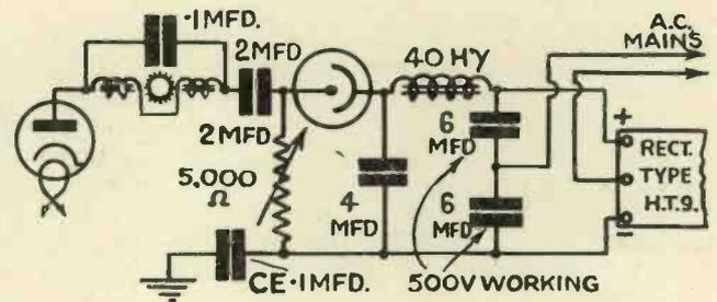
This is a simple arrangement in that there is no transformer and the potentiometer is across the supply instead of in series with the neon lamp. With the synchronising coils in series with the anode of the output valve the pictures are kept very steady.
