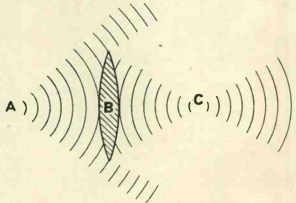
wave propagated in a homogeneous medium, for example, remains spherical throughout its travel, each little element of its surface being continuously propagated along a radius of the sphere.
