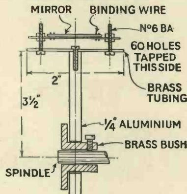
The drum is built up of a metal disc and brass tube. The method of fixing the mirrors is clearly shown.
