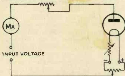
*Fig. 1.—Circuit of simple diode valve voltmeter.*
