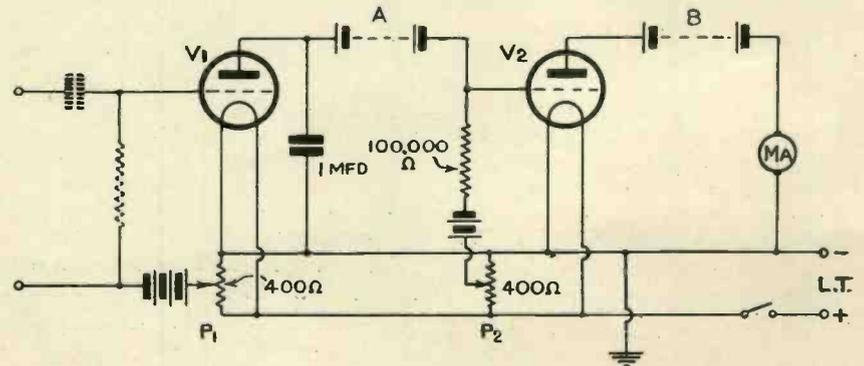
Fig. 4.—The circuit of the highly sensitive valve voltmeter described.
