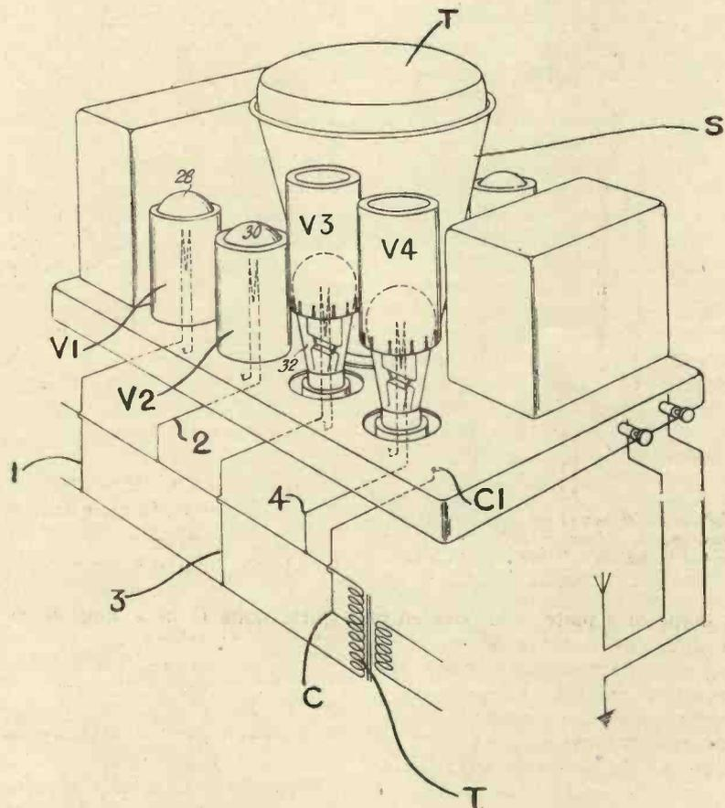
A wireless receiver with means for energising the valve filaments in groups with alternating current energy of opposite phase. Patent No. 412,435.
