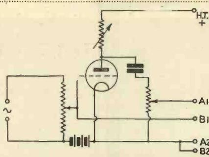
Fig. 4.—Connections for observing valve curves under working conditions.
