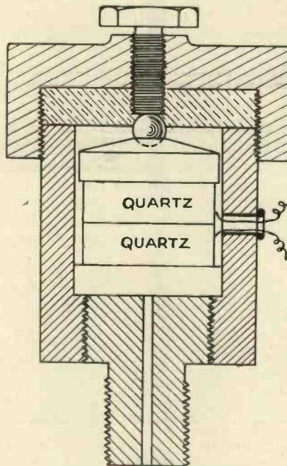
Fig. 5.—Crystal "pressure-gauge" for recording explosion pressures as used by Tokyo Institute.
