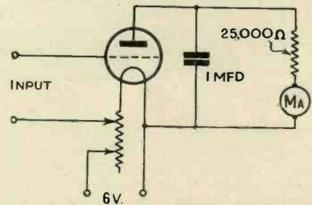
*Fig. 2.—Circuit of Moullin type valve voltmeter*
