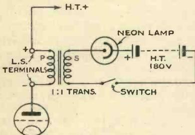
If you have two receivers and can spare one for television, this circuit can be recommended. Simply take off the loudspeaker and connect the neon lamp as indicated. The transformer primary connections should be reversed if the pictures are reversed.
