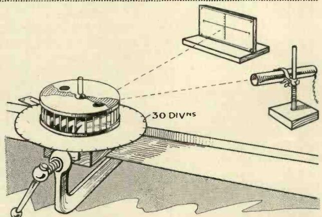
The lid with the boss fitted is then locked on a suitable length of spindle, which is arranged so that it will turn stiffly in a block of wood secured to a table. The sketch will make this
