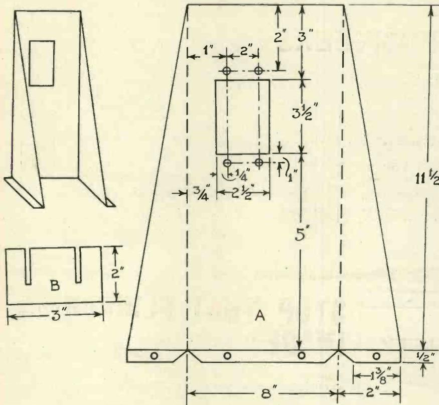
Fig. 2. Particulars of frame for providing the synchronising signal.
