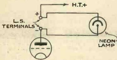
If you want to modulate your neon, this is the simplest circuit that will give good results. You want a high anode voltage, otherwise the circuit is straightforward.
