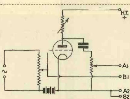
Fig. 4.—Connections for observing valve curves under working conditions.
