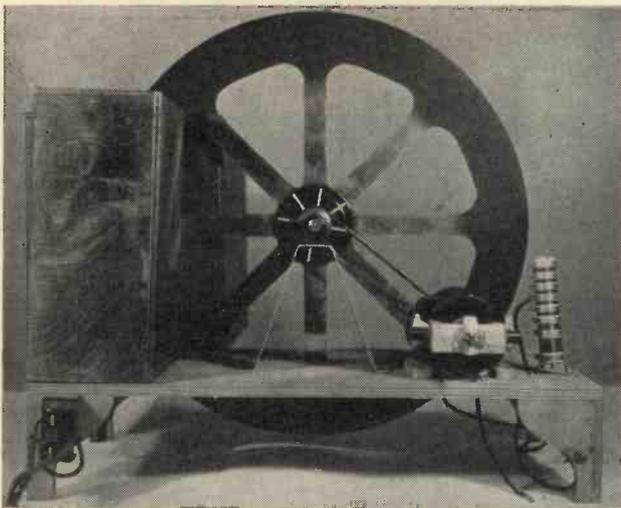
wide limits is possible. The two large lenses in the front light box are movable on short lengths of curtain rail which is obtainable from 6d. stores; the feet on the mounts are the sliders supplied with this rail.
