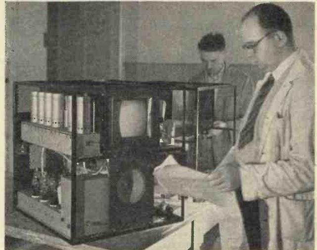
The chassis of the Telefunken cathode-ray receiver.
