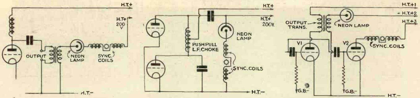
If you have over 200 volts available and can get at the anode circuit of the power valve, the neon can be modulated through a 1:1 transformer. The neon lamp is in series with the synchronising coils and the high-tension.
