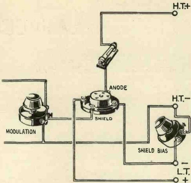
FIG. 4.—THE CIRCUIT FOR PRODUCING THE ELECTRONS.
