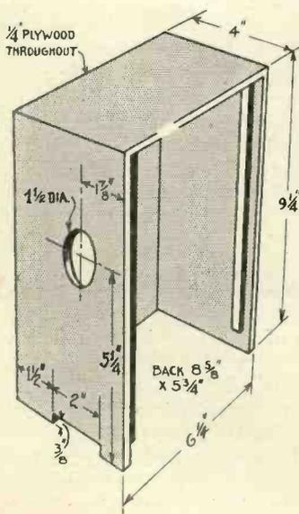
Details of the construction of the lamp box.
