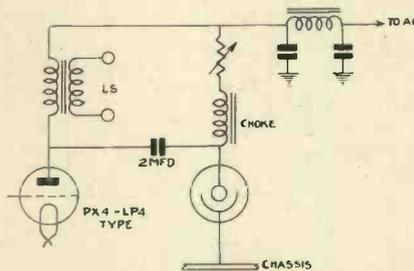
This is a circuit that can be used with the mains receiver. If the applied voltage is too high, the definition will suffer. This can be overcome by the use of the variable resistance.
