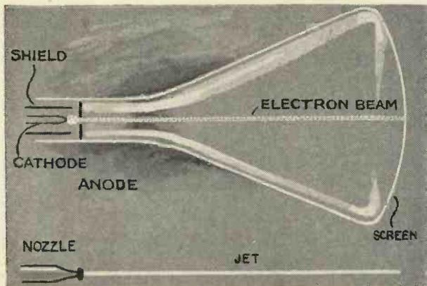
FIG. 2.—HOW THE BEAM OF ELECTRONS IS PRODUCED.
