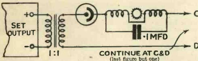
With this circuit simply remove the loudspeaker and connect a 1:1 transformer across the output terminals. In this way the circuit is suitable for home built or commercial receivers.
