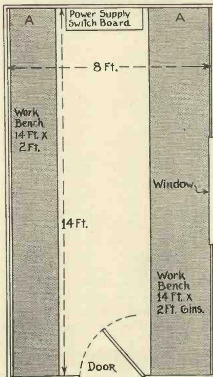
The arrangement for an outdoor laboratory utilising a shed about 14 ft. by 8 ft. The walls AA should be left clear for projection screens.
