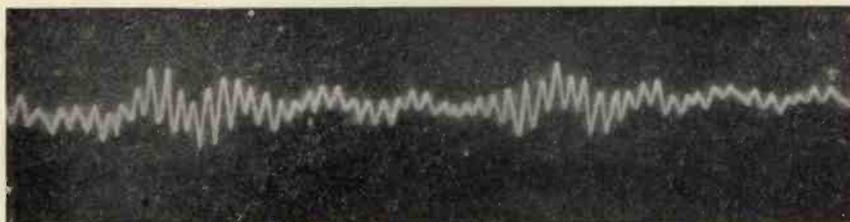
Fig. 3.—Sound record of vowel "e" recorded by microphone and moving film.
