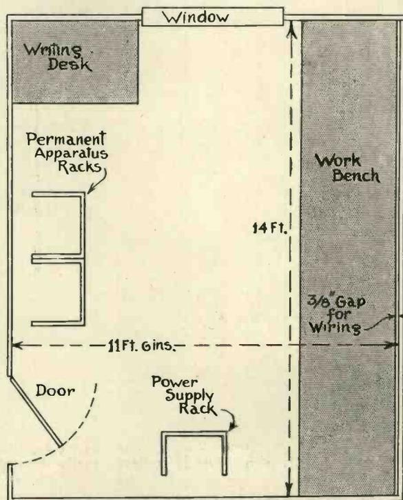
Plan showing the convenient arrangement of an average room for television experiment.
