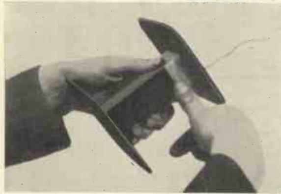
Winding the primary of the transformer.
