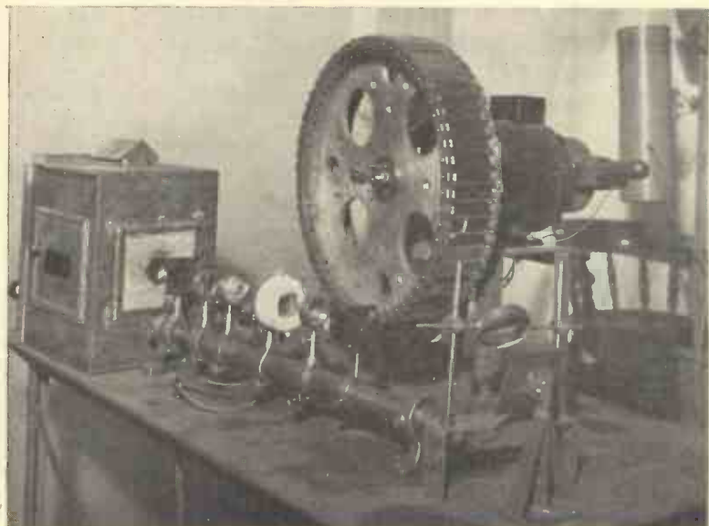
Close-up of the 60-line scanner showing the optical assembly.
