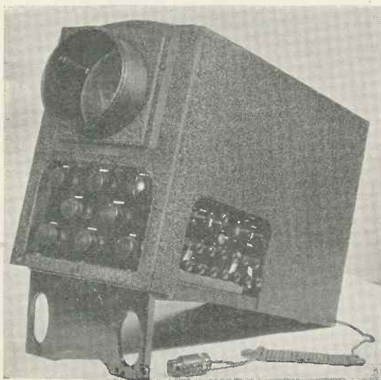
Fig. 2 (left).—Cossor mains operated oscillograph with self-contained valve amplifier.
