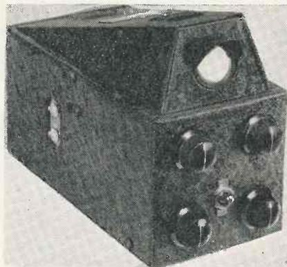
This small oscilloscope can be used for measuring modulation percentage with either a transmitter or on received signals.
