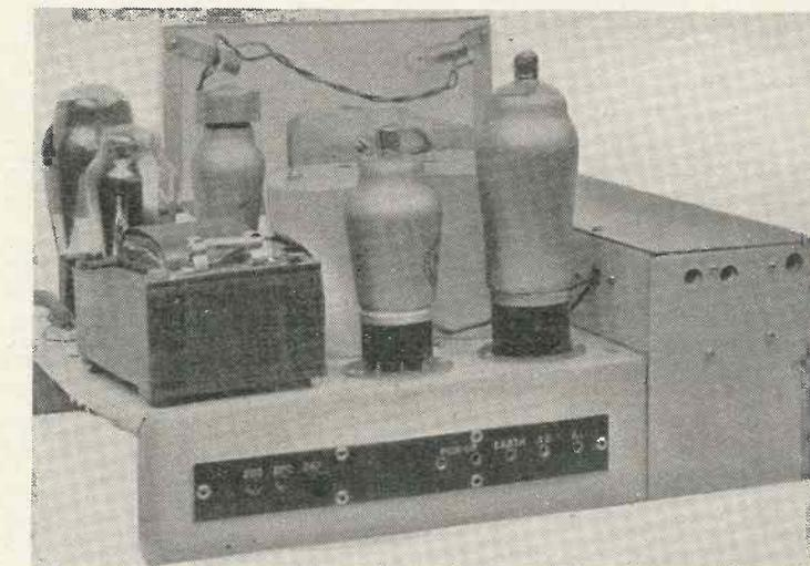
This super-het receiver is designed for all-wave reception and should be compared with the vision chassis illustrated on the preceding page.
