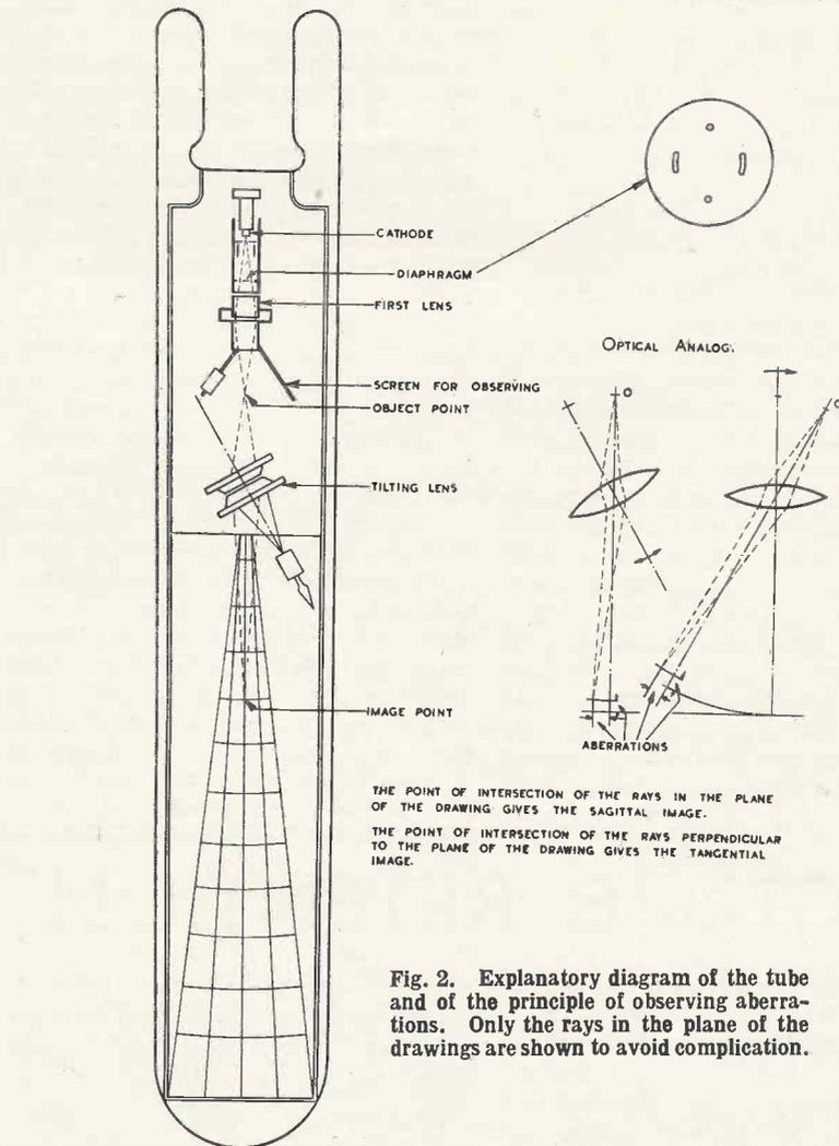
Fig. 2. Explanatory diagram of the tube and of the principle of observing aberrations. Only the rays in the plane of the drawings are shown to avoid complication.
