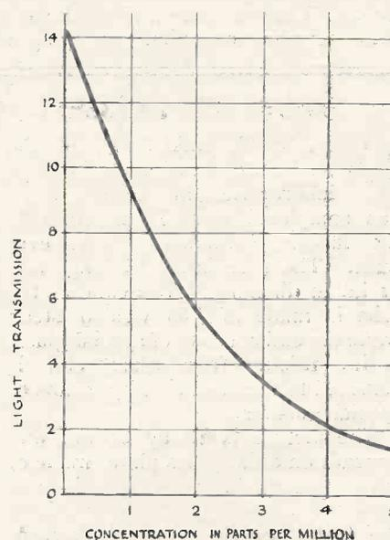
Fig. 2. Graph showing the proportion of light transmitted by solutions of colloidal graphite when acted on by a magnetic field.
