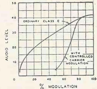
Fig. 8. Percentage of modulation in ordinary and controlled carrier transmitters at various audio levels.
