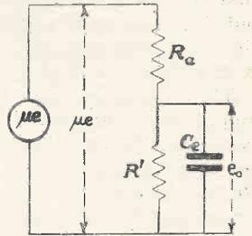
Fig. 1c. A further simplification showing how the stray capacities shunt the output voltage.
