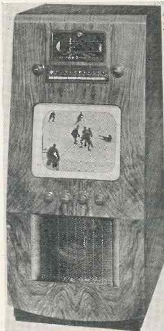
A console type receiver is the H.M.V. 1850. The picture size is 11 5/8 in. by 9 3/8 in., and in addition, an all-wave push-button radio is provided.
