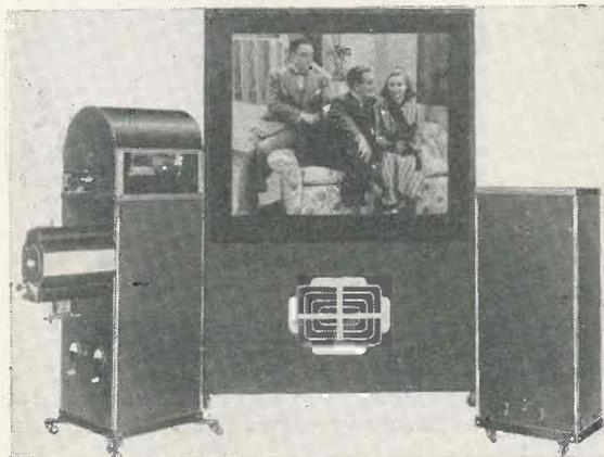
Of very special interest are the Scophony receivers as they are the only mechanical-optical type available. Above is the 4 ft. projection receiver and on the right a homes receiver giving a 2 ft. picture.
