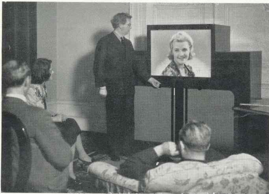
Mr. Baird's 600 line colour televisor. The screen receives either 600 line colour pictures or by pressing a button the B.B.C. 405 line monochrome pictures. It measures 2' 6" x 2' 0". The set includes an automatic record-changing radiogram and an all-wave wireless receiver.
