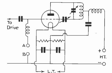
Fig. 4.—With this circuit in use the P.A. will operate down to 10 metres with grid modulation.
