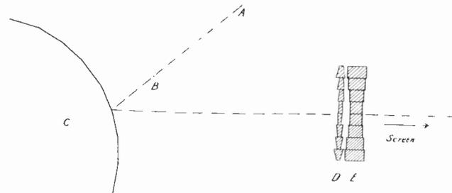
"ray divider"—a series of small angle prisms across which each patch of light in passing is made to go across the screen in eight contiguous lines; this it is hoped will shortly be marketed in a completely adjusted
