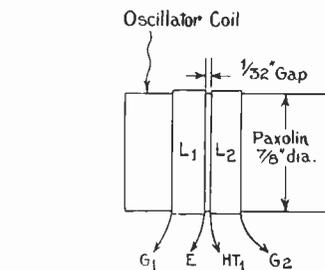
Fig. 4.—Here is the coil former, all the necessary winding data are given in the text in concise form.
