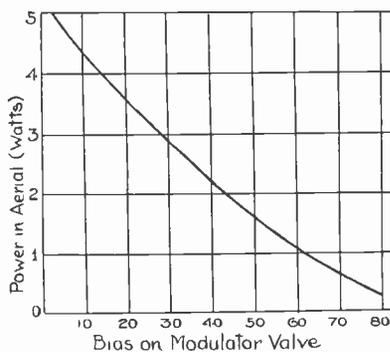
Fig. 6 (left).—Modulation characteristic.
