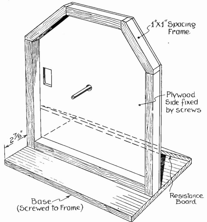
This drawing shows the partly assembled case.
