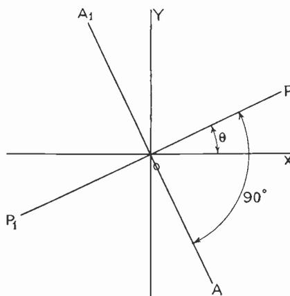
Fig. 1.—Linear polariscope with crossed nicols.— $PP_1$  is the vibration direction of polariser;  $AA_1$  is the vibration direction of analyser;  $OX, OY$  are the vibration directions of birefringent section in the polariscope.
