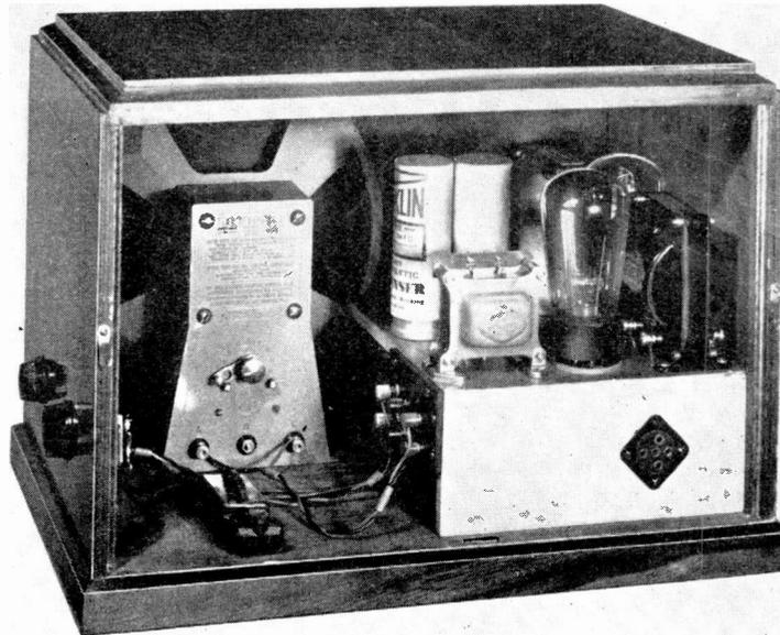
*Most of the wiring is point to point. This is most essential on the higher frequencies. Keep the connecting wires short.*
