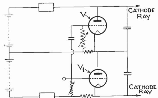
Fig. 1.—Circuit for producing interleaved scanning. Patent No. 423,101.
