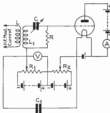
*This is the circuit for the suggested meter. It is better to use this than to rely on the fact that 23 per cent. rise should mean 100 per cent. modulation.*
