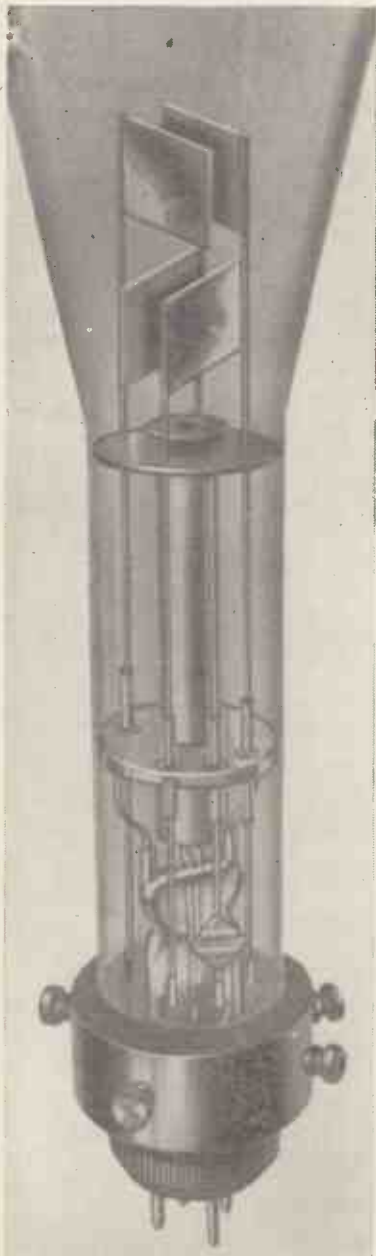
Fig. 1.—Photograph of the electrode assembly of the cathode-ray tube.
