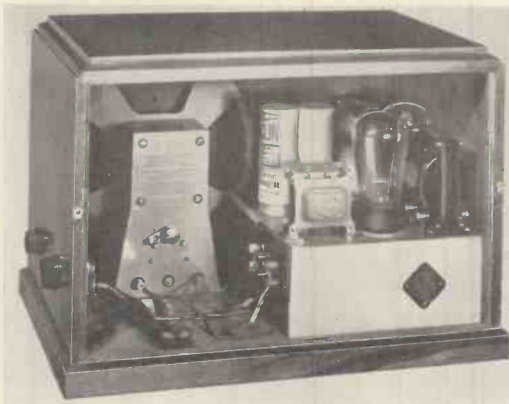
Most of the wiring is point to point. This is most essential on the higher frequencies. Keep the connecting wires short.
