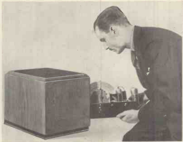
Both the cabinet for the receiver and the cabinet for the power pack match up. They have been arranged to fit together one above the other.
