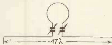
Fig. 1 (left).—The leads to the valve form an oscillating circuit as shown.
