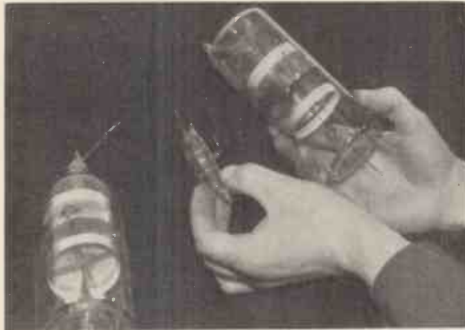
Three forms of electron multiplier are shown by this photograph.
