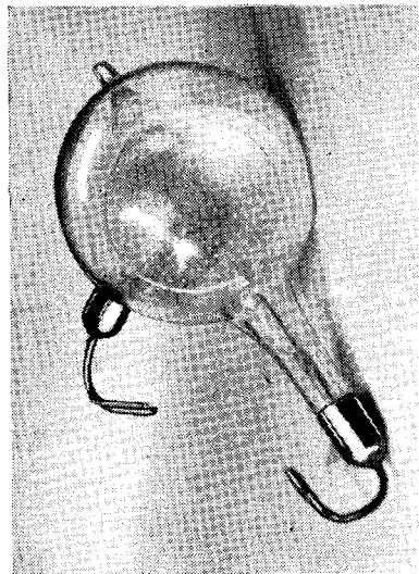
Fig. 7b.—A caesium photo-electric cell of the "plate-cathode" type, suitable for televising films. Commercially produced for talkies.
