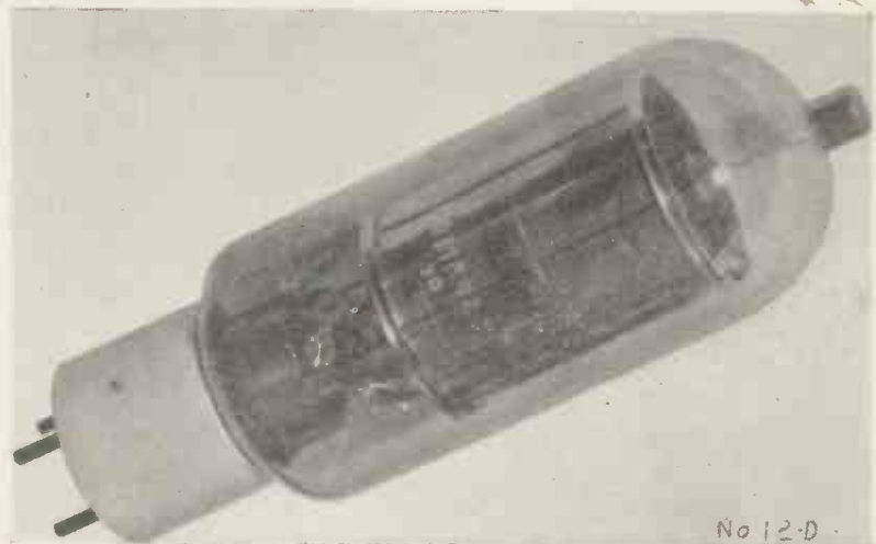
This photograph shows a \frac{1}{2} -kilowatt Multipactor tube for use as an oscillator.
