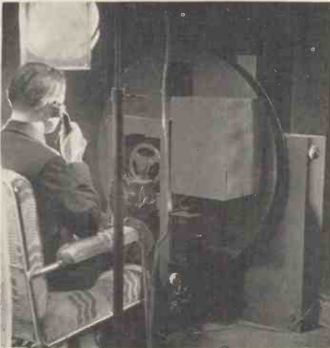
This photograph shows the scanning arrangements. The synchronising projector is contained in the case at the right and its photo-cell and associated amplifier at the rear. The vision photo-cell case can be seen at the back at the top and below this are the amplifiers.
