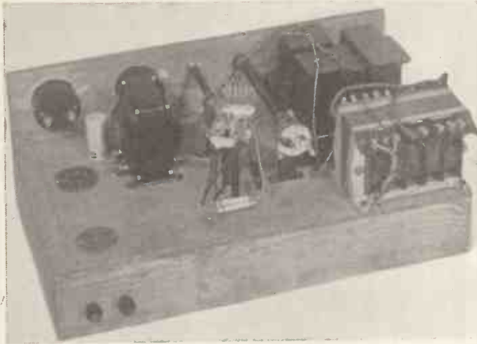
The oscillator section is mounted between the other two stages to prevent hum pick-up by the L.F. amplifier.
