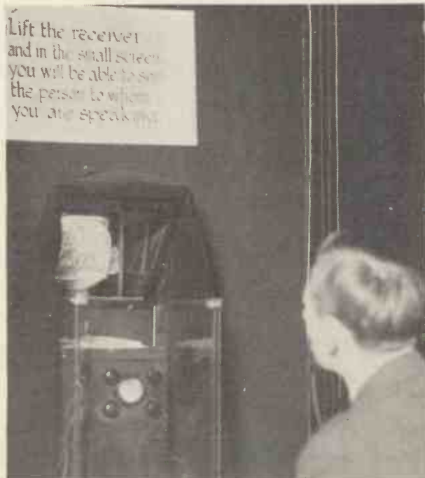
The cathode-ray receiver installed in a booth; the viewing screen is a mirror placed at an angle of forty-five degrees.
