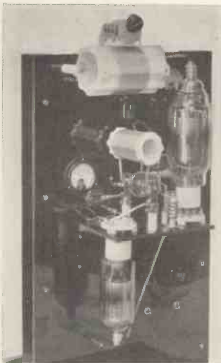
The Farnsworth Multipactor tube in use as a power amplifier driven by a smaller tube used as an oscillator.
