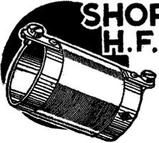
An efficient low-loss type of skeletonised H.F. choke designed for use on short-wave bands. This choke has a paxolin former with a winding of high quality enamelled wire, strip-type terminals, for connection by soldering if desired.
