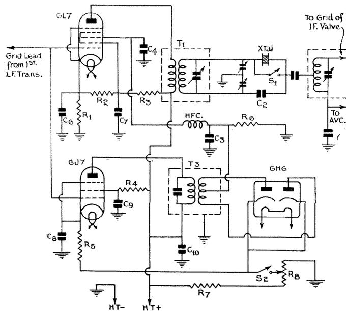
*As most of the noise in the average large amateur super-het comes from the intermediate-frequency stages this silencer should be of particular interest to constructors.*
