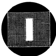
*Insufficient line amplitude. Faulty valve or low H.T. to line scan unit.*
