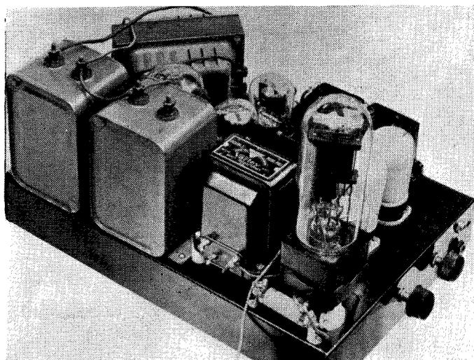
*The 60-watt valve shown is only used for anode modulation. This valve has its own power supply on the same chassis.*
