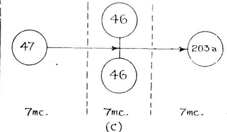
Fig. 4c.—This is the final valve line-up when used on the lower frequencies.
