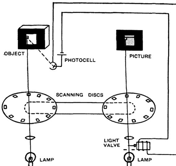
Fig. 1.—Diagram showing the elementary principle of television.
