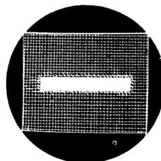
*Insufficient frame amplitude. Faulty valve or low H.T. to frame scan unit.*
