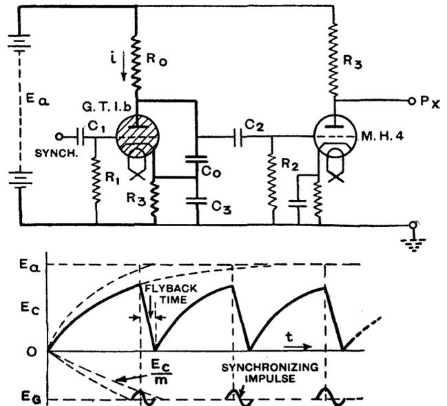
Fig. 5.—Time base circuit using gas-filled relay and (below) the saw-tooth wave form produced.
