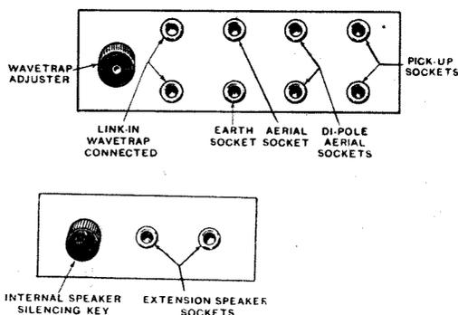
*These are the terminal panels on the back of the cabinet. Connections are made by plugs.*
