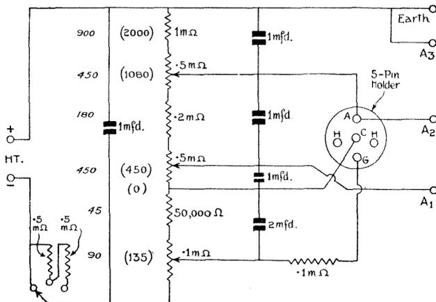
Fig. 1.—Circuit diagram of resistance chain.
