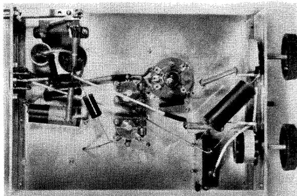
The Mullard AP4 valve is mounted in a special Bulgin low-loss holder.
