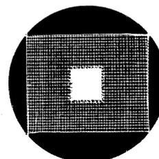
*Both amplitudes small. Low H.T. to scan units. Faulty rectifier valve.*
