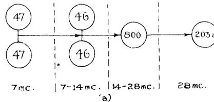
Fig. 2a.—An additional stage is required for 10-metre work.
