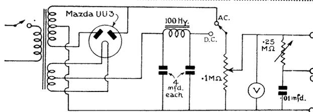
Fig. 2.—Circuit for providing A.C. and D.C. for calibrating tube deflections.
