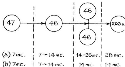
Fig. 4a.—Shows the circuit for 10-metre operation and Fig. 4b for 20 metres.
