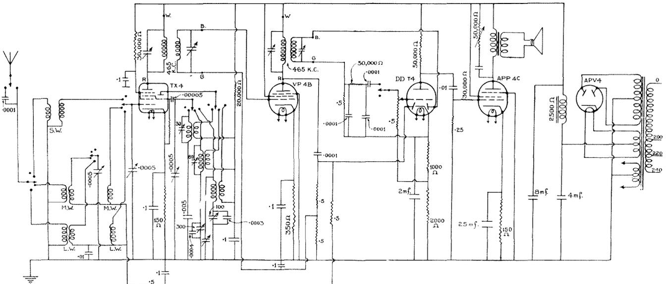
*An output of over three watts is possible with the APP4C pentode. This 3-channel receiver tunes from 16 to 2,000 metres.*
