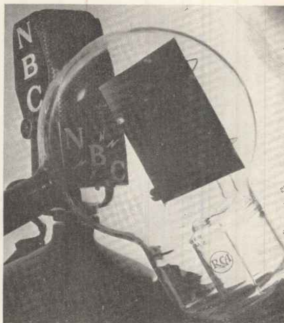
R.C.A.'s famous Iconoscope, the tube which transforms what it "sees" into electric impulses. In the background is the well-known N.B.C. microphone.
