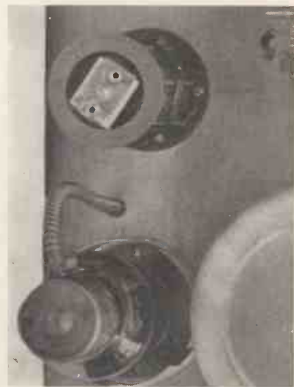
This close-up view of the detector coil shows how the trimming condenser is mounted. The X 41 valve is also shown without screening.
