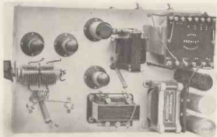
In this plan view, the metal screening can has been removed, showing the exact layout of the components. Note in the text the remarks concerning the mains transformer, intervalve transformer and smoothing chokes.
