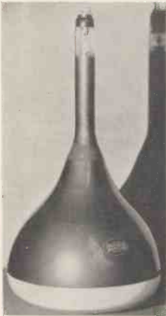
The Ferranti tube is one of the few in this country to employ magnetic scanning.
