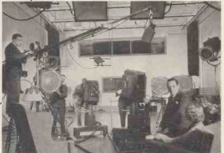
General view of the N.B.C. experimental studio in the R.C.A. building. The "camera-men" are focusing Iconoscopes, and the microphone is swinging into position.
