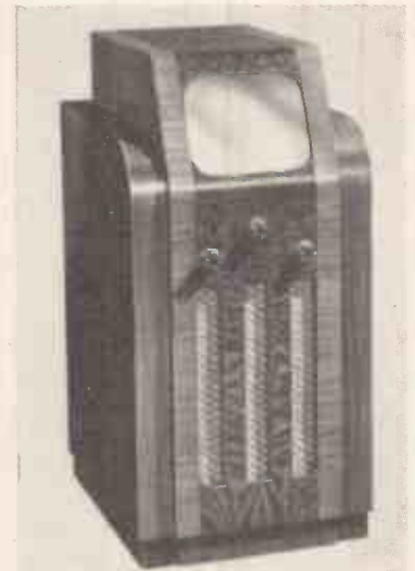
The Pye Minor model is a console with a directly viewed picture. Except for picture size it is built upon conventional lines.
