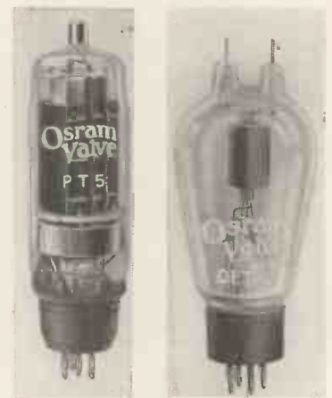
On the left is the new PT5 transmitting pentode suitable for amateur use. On the right is a triode valve with carbon anode and very low inter-electrode capacity. The type number is DET12.
