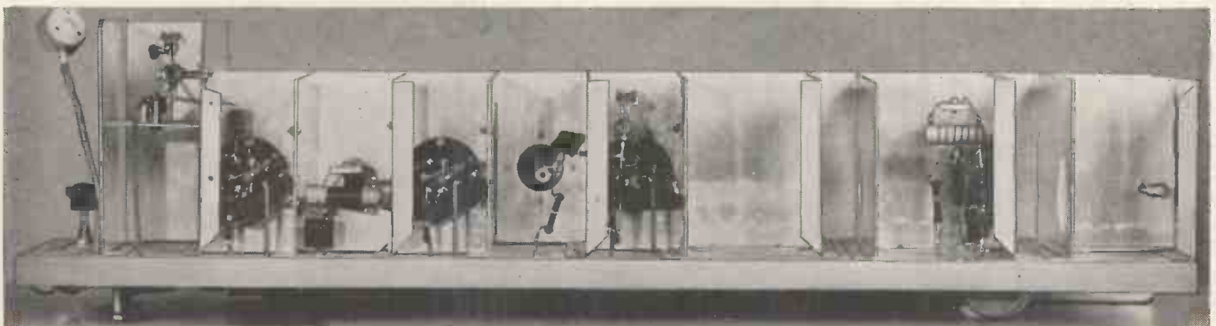
A photograph of the left-hand side of the receiver chassis showing the components in position. The simple construction will be apparent.
