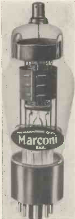
Notice the new Octal base with 8 pins and a locating key on this new Marconi W63 pentode which is the equivalent of the American 6 K7G.
