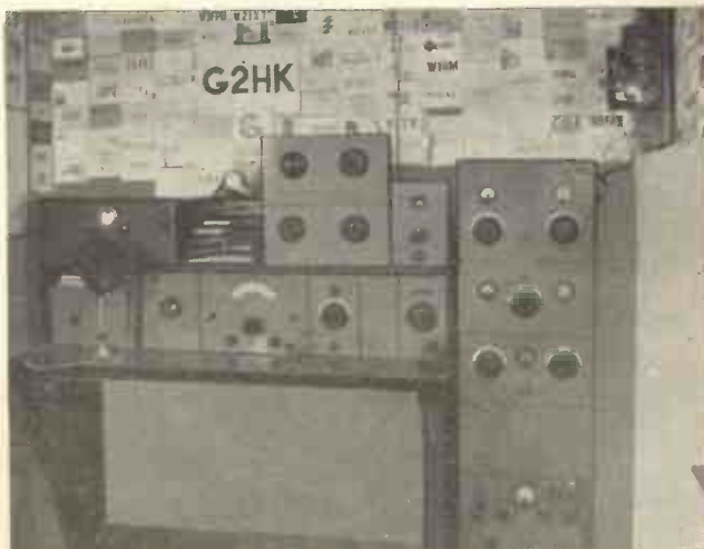
This is G2HK who operates mainly on 20-metre phone with an input of 8-10 watts. In this illustration can be seen the communication receiver and 5- and 20-metre transmitters.
