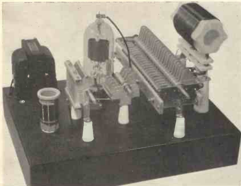
A good example of efficient P.A. design using the T-125 triode amplifier. Notice the short leads and the lay-out chosen.
