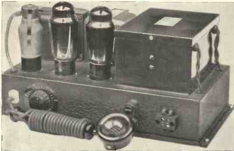
The finished amplifier with crystal microphone and built-in converter. The output is between 5 and 7 watts depending on the percentage of distortion allowed.
