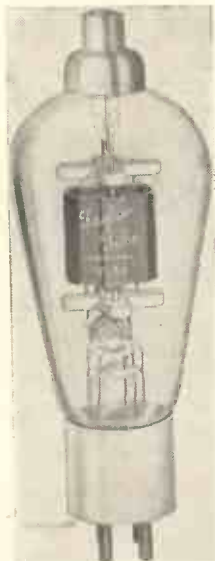
One of the best low-capacity triodes available. It is the Taylor T-55 with a 55-watt anode dissipation.
