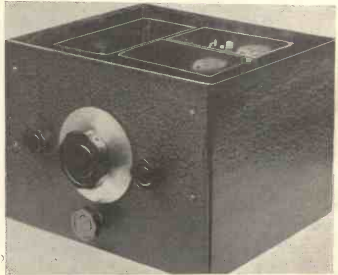
The finished receiver presents quite a professional appearance, being built on a steel chassis and housed in a steel cabinet.
