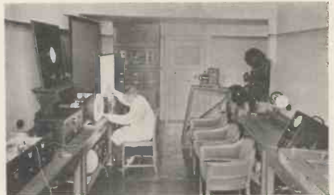
Television laboratory. The receiving set for 441 lines can be seen on the left, while in the foreground is an electrolytic trough for plotting field lines. At the back is a film scanner and apparatus for investigating stereoscopic projection.
