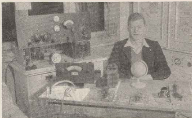
G6ZO only operates on C.W. on the higher-frequency bands. A two-stage transmitter is used with a 4304A in the final stage.
