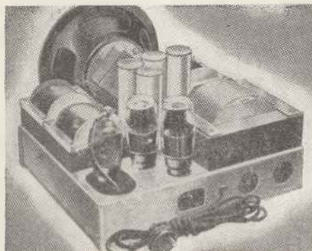
The chassis of the power unit also carries the moving-coil speaker.
