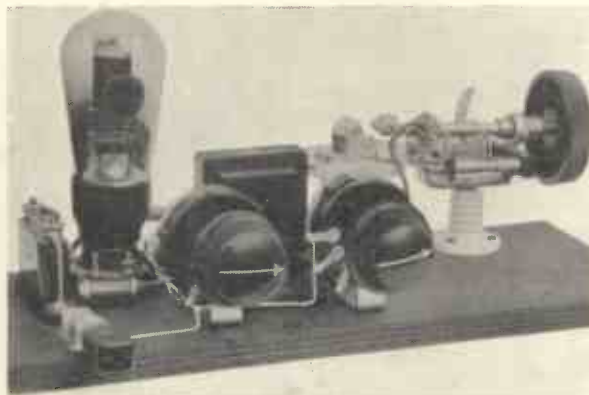
The tuning condenser in the receiver is mounted on a stand off insulator so that it is level with the grid and anode contact of the acorn valve. A head-phone jack is in the left-hand corner.
