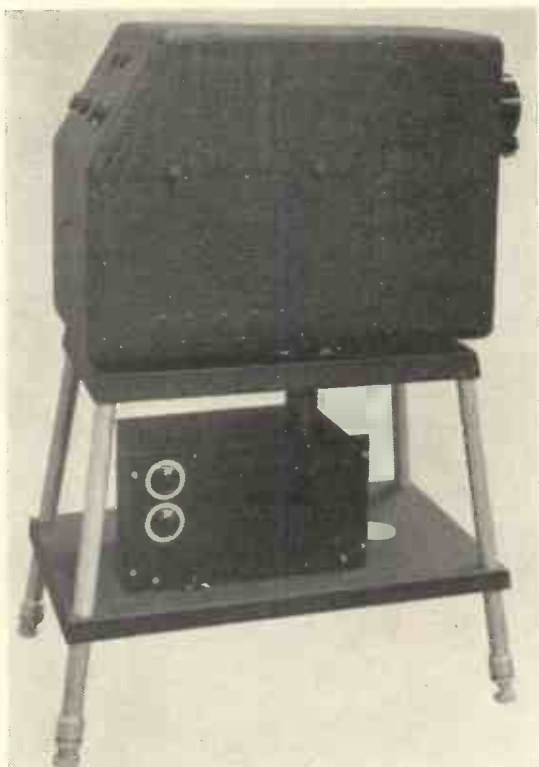
This photograph shows the Baird projection unit incorporating the tube, time base, final stage vision amplifier and intermediate vision frequency amplifier.
