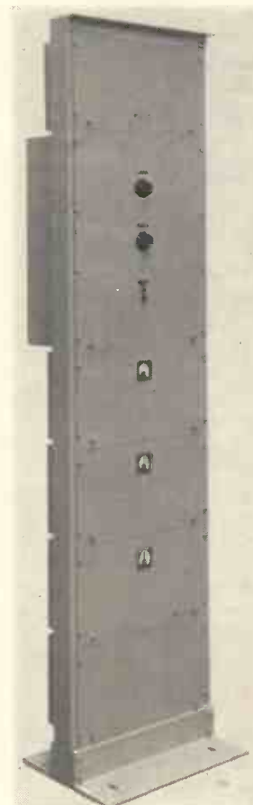
The rack containing the sound and vision receivers and their power supply units.
