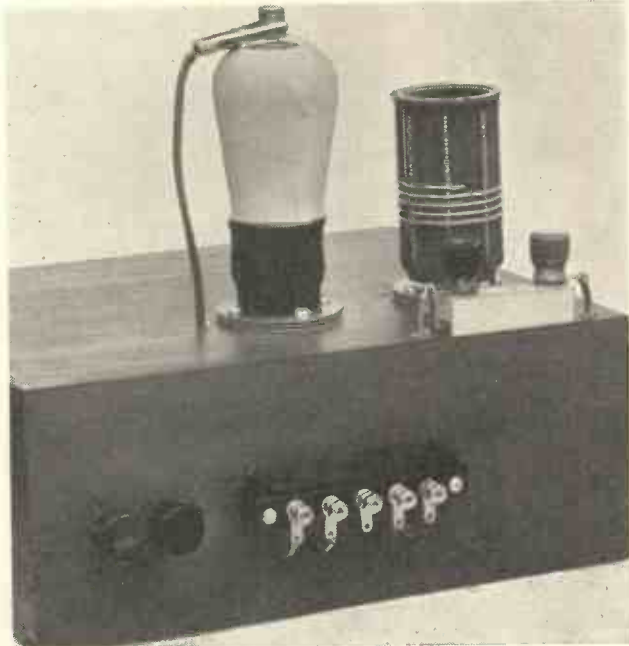
Only four of the terminals are used with the single valve. The fifth terminal comes into use when the second valve is added.
