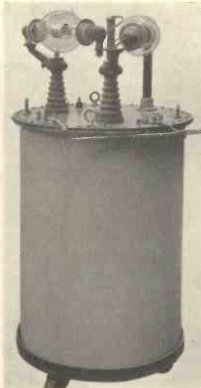
The extra-high tension unit. Note the special precautions taken for insulating.
