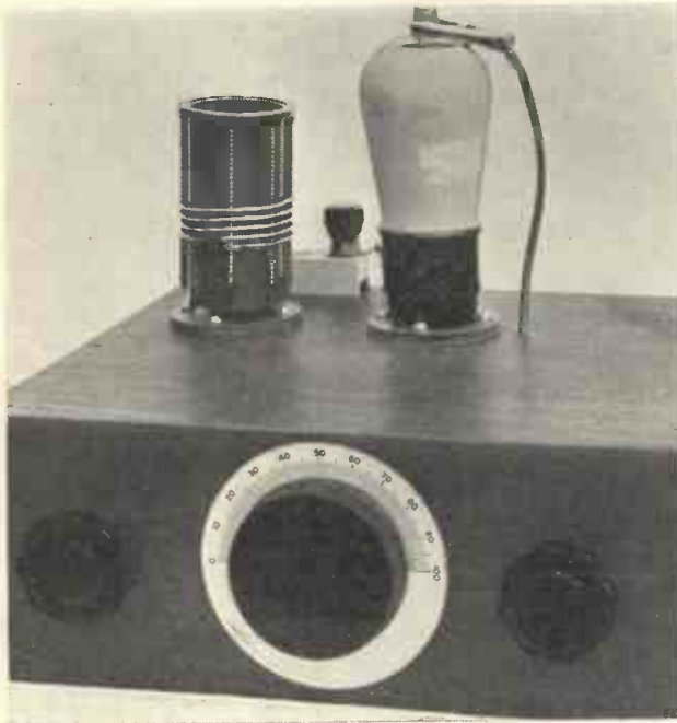
The control on the left is the Eddystone bandspread condenser. The tuner is in the middle and the reaction control on the right.
