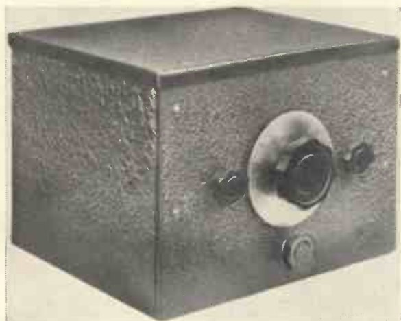
The receiver is entirely screened so that it does not pick up local noise or any signals other than those via the aerial feed line.
