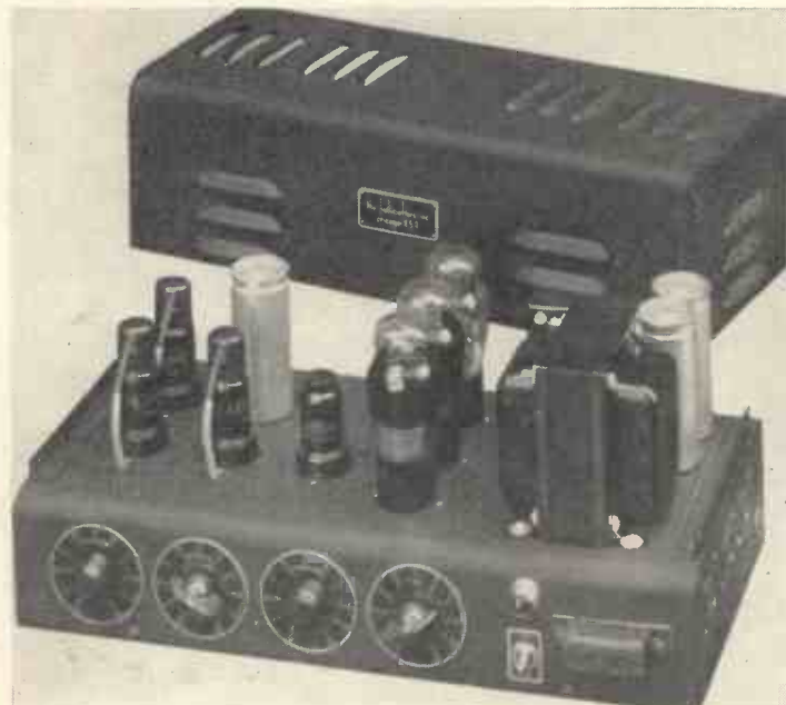
Although designed for public address work this amplifier is becoming very popular amongst amateurs. It includes two-channel input, tone correction and variable base compression.
