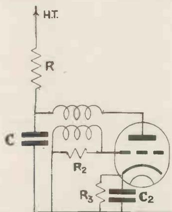
Fig. 1. A single-valve discharge circuit with anode and grid coupling.
