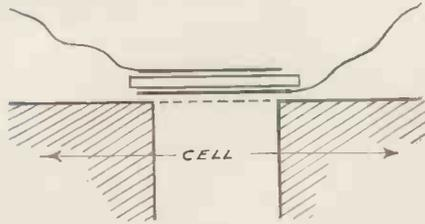
Fig. 5. Crystal electrode arrangement.
