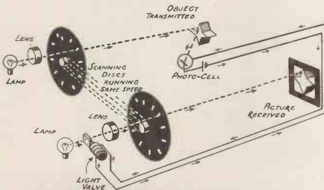
C. Schematic outline of mechanical transmitter and receiver.
