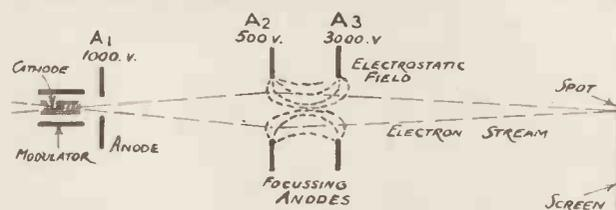
How the cathode beam is focused by applying voltages to the anodes of the cathode-ray tube.
