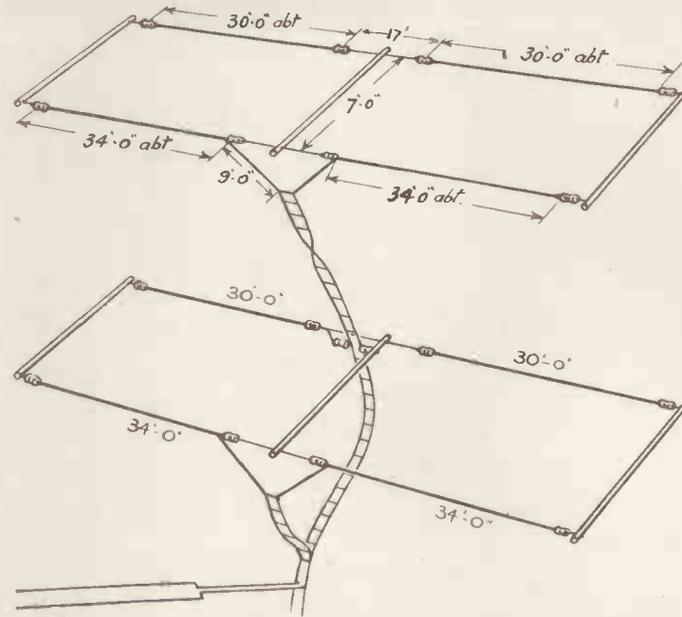
Fig. 3. The final scheme which has a very strong broadside pattern. Only a moderate length is required between poles, but the best results will only be obtained when the top length is at least 70 feet above ground.
