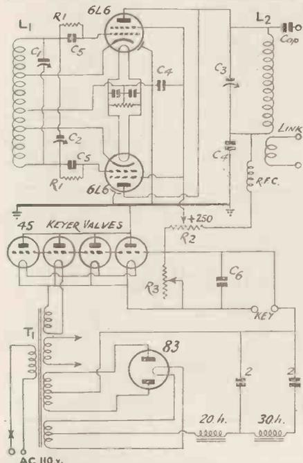
Fig. 1. W9JID developed this ECO circuit and recommends the use of a valve keying circuit as shown.
