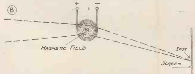
Diagram showing how the cathode beam is deflected magnetically.
