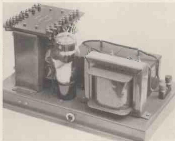
This is a suggested power pack of conventional design with a 500 volt-transformer, 200 mA. smoothing choke, a 5Z3 rectifying valve and two 4-mfd. condensers.
