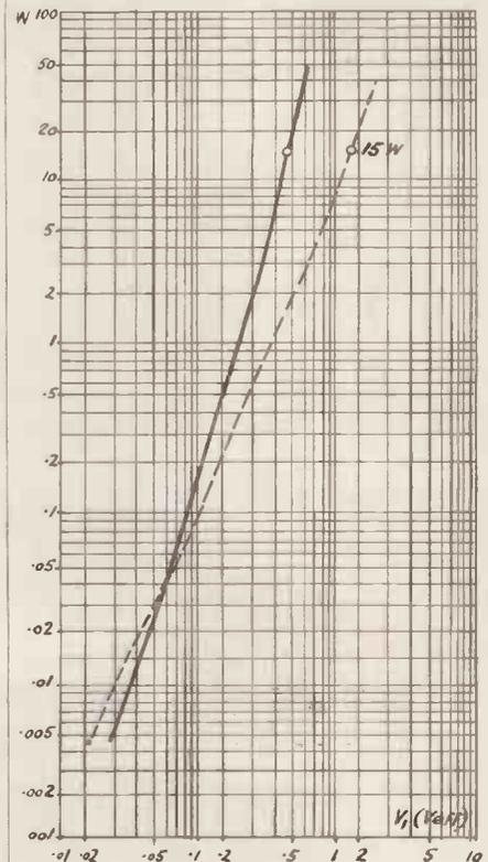
Fig. 5. These curves show the operation of the volume expander.
