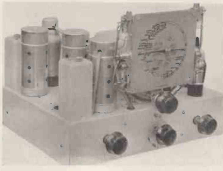
Although this 8-valve B.T.S. chassis only costs 12 guineas it tunes down to 10 metres and has a good performance on that wavelength. A 9-valve model costs £14-14-0
