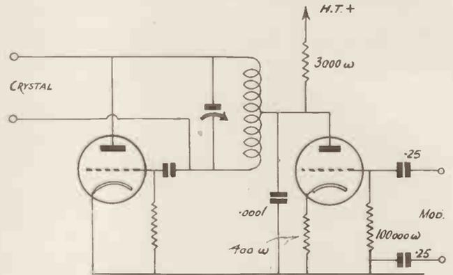
Fig. 7. Oscillator (left) and modulator (right) circuits.
