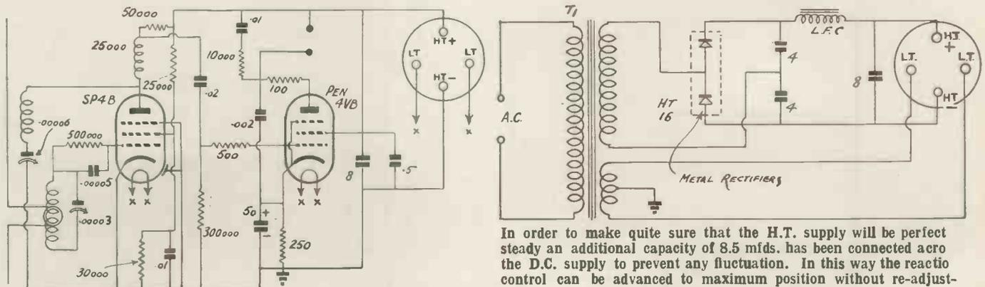
Only trimmer condensers are needed in this receiver and once the station has been received they do not need touching.
