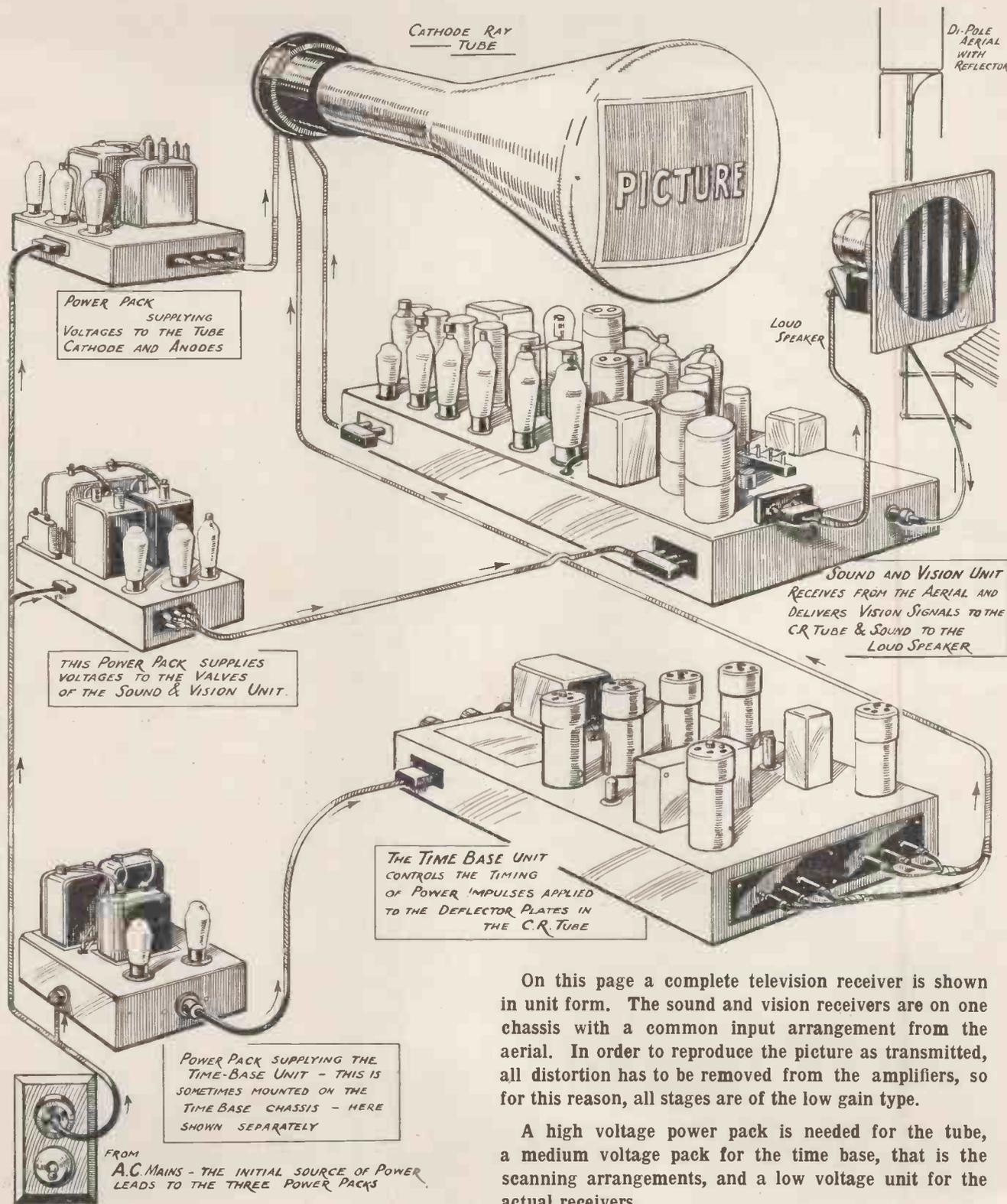
On this page a complete television receiver is shown in unit form. The sound and vision receivers are on one chassis with a common input arrangement from the aerial. In order to reproduce the picture as transmitted, all distortion has to be removed from the amplifiers, so for this reason, all stages are of the low gain type.
