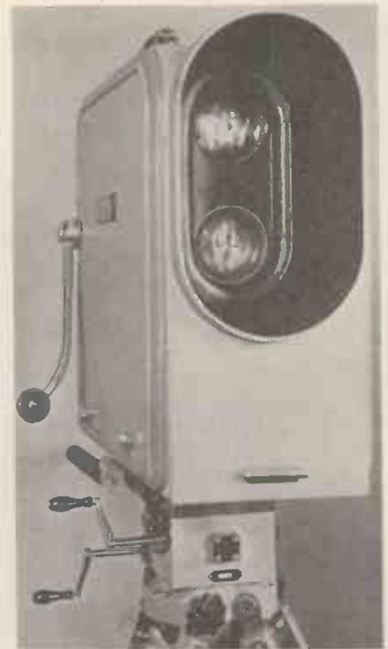
The Fernseh Iconoscope camera.
