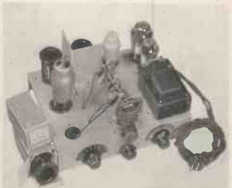
An A.C. receiver from New Times Sales. It has four valves and band spread tuning. The price of the kit is 75/-.
