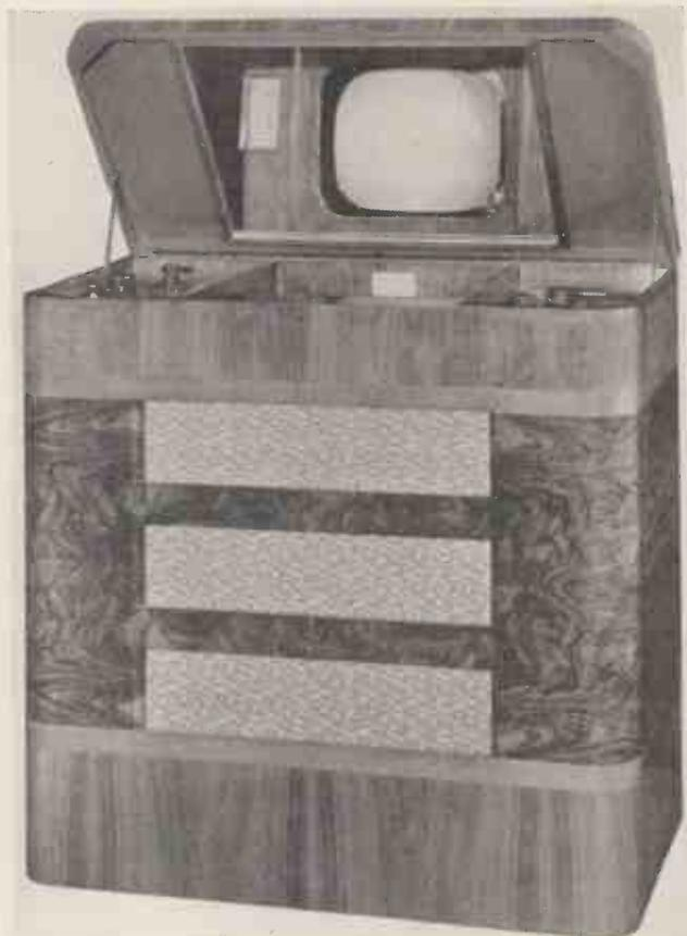
This is one of the de luxe models exhibited by the G.E.C. In addition to the sound and vision receiver, which gives a picture 13½ in. by 11 in., a powerful 6-valve all-wave set is incorporated.
