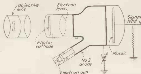
Diagram of the new Iconoscope. The mosaic, bombarded by an electron image from the illuminated photocathode, emits secondary electrons. The mosaic is scanned by a beam from the electron gun.
