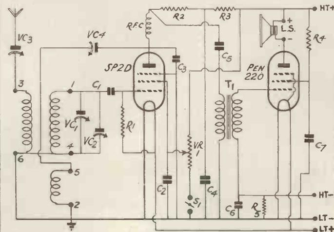
The first part of the receiver is almost unchanged. A pentode valve has been included in the output stage which is parallel-fed transformer coupled to the detector valve.
