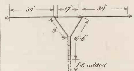
Fig. 2. With this arrangement the aerial has an effective length of 43 feet.
