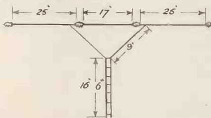
Fig. 1. This antenna has a portion of the top length bent towards the stub.
