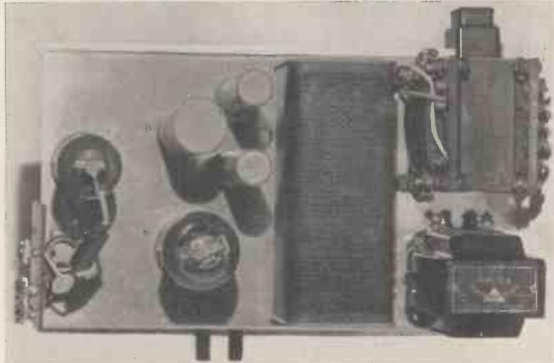
A plan view of both units. The upper of the two small condensers is the one to be isolated.
