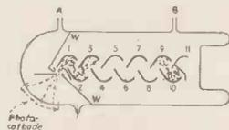
Diagram of ten stage electron multiplier using electrostatic fields only, described by V. K. Zworykin.
