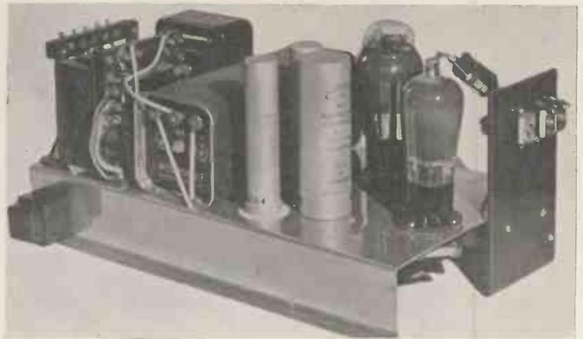
The complete two-valve receiver with power unit is mounted on a single chassis in this manner.
