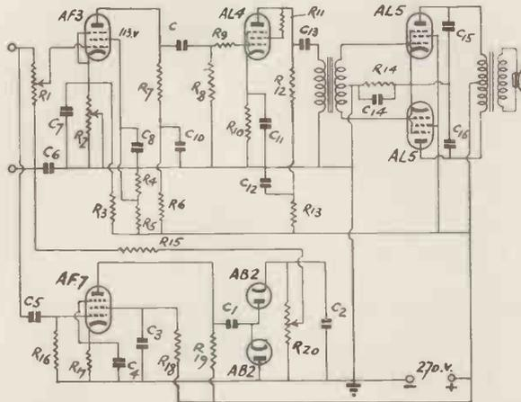
Fig. 4. Circuit of an LF amplifier giving 15 watts and including volume expansion.
