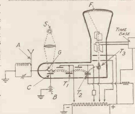
Combined cathode-ray tube and electron multiplier. Patent No. 485,412.
