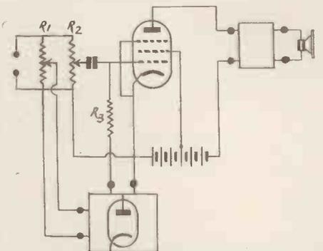
Fig. 3. Theoretical circuit of an experimental volume expander.
