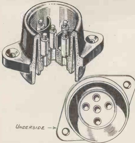
A high-tension valve holder for 12,000 volt use. A Belling-Lee product.
