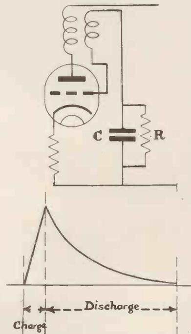
Fig. 2. (a) 'Squegger' circuit in which the condenser C is charged during oscillation and discharges slowly. (b) The discharge curve is exponential when R is used across the condenser.
