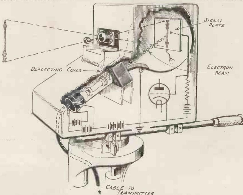
F. Diagram of pick-up camera which converts light into electrical impulses.
