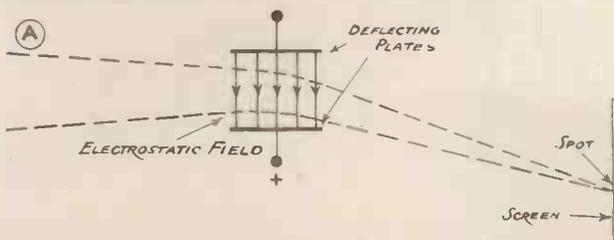
Diagram showing how the cathode beam is deflected electrostatically.
