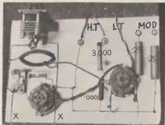
Fig. 9. Modulated oscillator. Points marked x show crystal connections.
