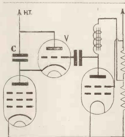
Fig. 3. A discharge valve (V) driven from an oscillator. Minor details have been omitted in the circuit, which is only diagrammatic.
