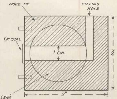
Fig. 4. Cell, with dimensions.
