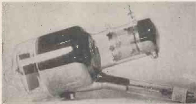
Photograph of new Iconoscope. The mosaic may be seen at the extreme left. The gauze cylinder, adjacent to the photocathode, aids in focusing the electron image. The electron gun is similar to that used in modern cathode ray tubes.
