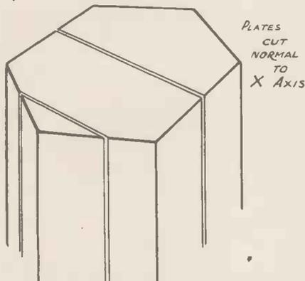
Fig. 1. Cutting quartz crystals.
