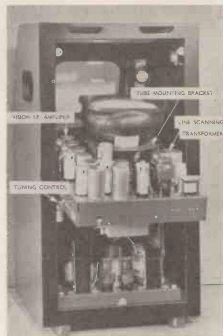
A rear view of the Murphy receiver showing the hinged chassis.
