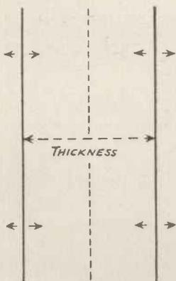
Fig. 2. Mode of Vibration of crystal.
