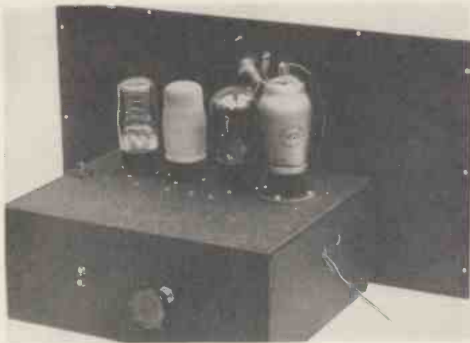
The amplifier in skeleton form looks most business-like and as all the components of the smaller kind are protected by the chassis, there is very little likelihood of any breakdown.
