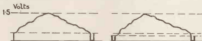
Figs. 4 and 4a. The signal at the output of the diode. (a) The same signal altered by diode characteristic.
