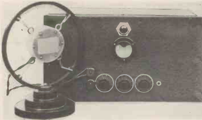
The entire amplifier is self-contained in a standard Eddystone steel cabinet. Separate volume controls for each microphone and a common tone corrector are embodied.
