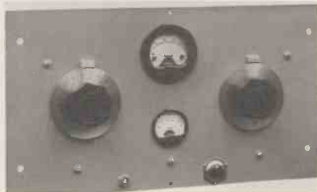
Fig. 2. Despite the symmetrical layout of the chassis components, the panel also has a pleasing appearance. Constructors wishing to use metal-cased anode meters can connect in series with the centre tap of the filament transformer.
