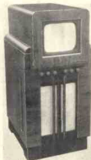
The Ferranti 10 in. by 8 in. console television receiver.
