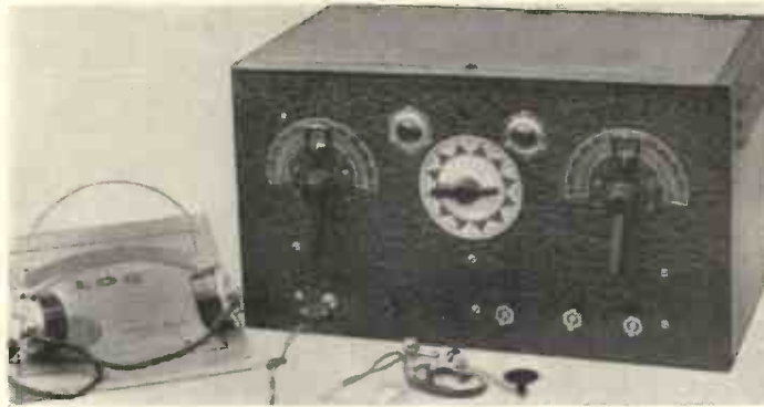
This front view gives a good idea of the controls and layout. The transmitter is designed for C.W. operation and cathode keying.
