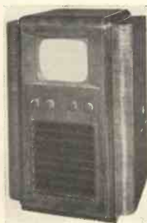
Below: The Burndept console television receiver. Picture size 10 ins. by 8 ins.
