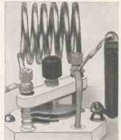
This is the coil for 10-metre output, and is made of 10 gauge wire.
