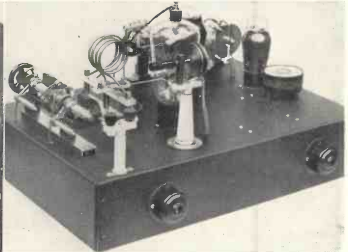
Above is a view of the transmitter showing particularly the tank coil and link winding while on the left is a plan view showing the layout of the components.
