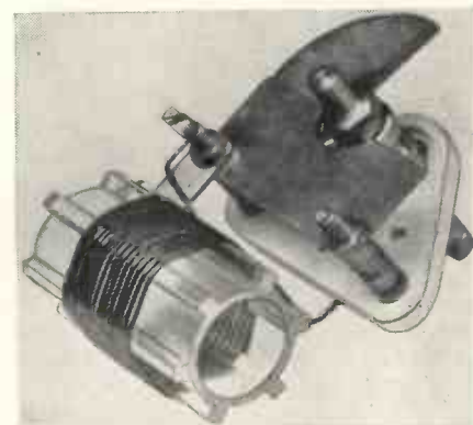
The 20-metre anode coil is fixed directly to the tuning condenser.
