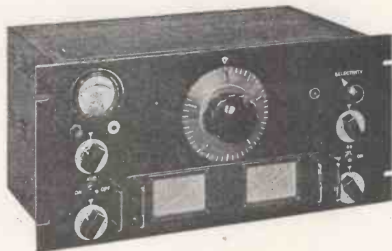
One of the most popular sets is the HRO which covers 1.7 Mc. to 30 Mc.
