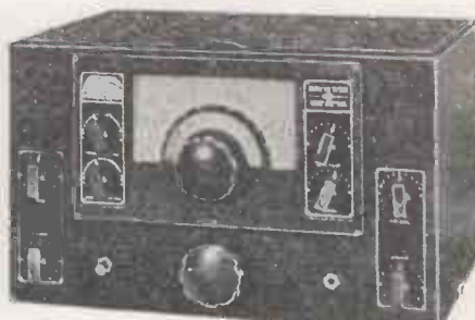
National receivers are very popular. This is the NC-100XA. It has a crystal filter and covers 540 Kc. to 30 Mc.
