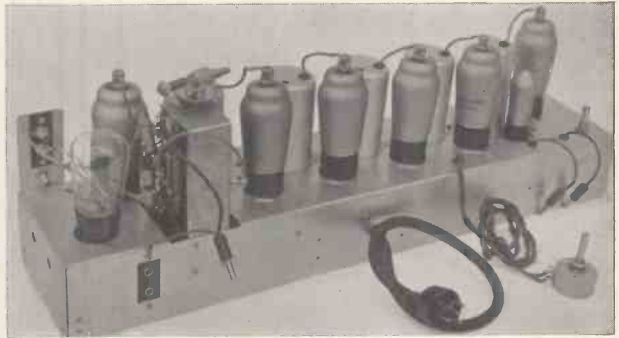
Fig. 1. An early vision receiver employing many stages of amplification.
