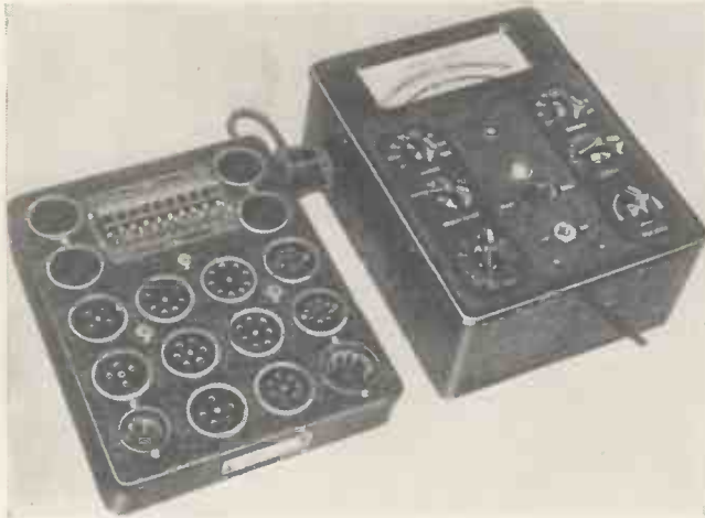
Fig. 4. The Avo valve tester with associated universal panel. As explained in the text this is a most comprehensive instrument.
